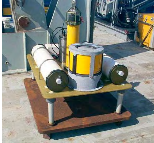
Figure 26. Bottom Pressure Sensor Platform.
