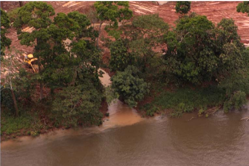
Figure(s) 4.5. Photographs showing drastic alteration of natural surface runoff patterns and sediment run-off into the San Juan de Nicaragua River
