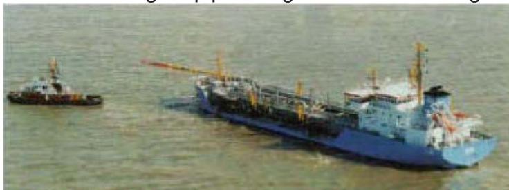
Suction dredger under way, designed to unload through pipes.
