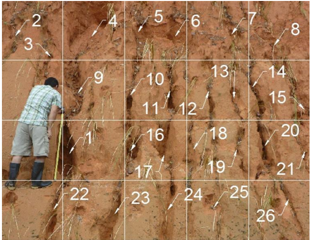
Figure 30. Rill erosion monitoring site on a cut slope, with rills numbered and 1 metre grid overlaid for scale (from the UCR Report).
