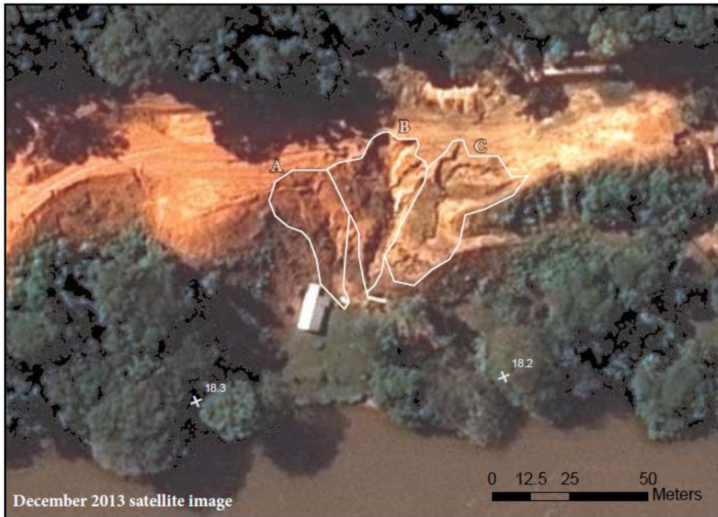
Figure 2.10. Severely Eroding Site 9.6, 18.2 km downstream of Mojon II. High-resolution satellite image of December 2013.
