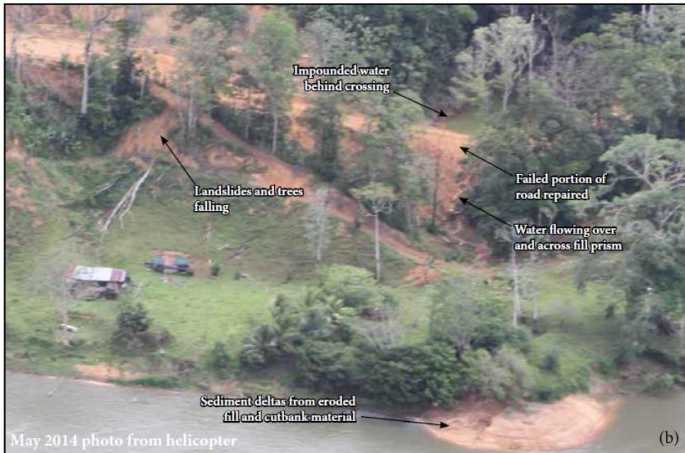
Figure 2.4. Severely Eroding Site 9.4, 18 km downstream of Mojon II. Oblique aerial view from May 2013.
