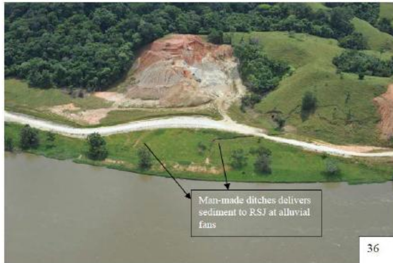
Figure 2.28. Quarry site approximately 7.7 km downstream from Mojon II, where man-made ditches deliver sediment to the River. Photograph from 2012 Kondolf Report, Appendix B (October 2012).
