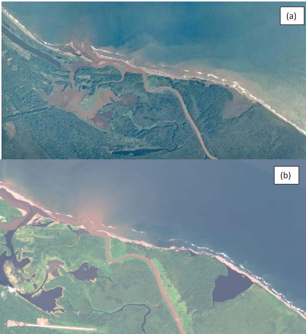
Figure 5.4 Satellite images showing that flow from the lower Río San Juan carries turbid water with a high concentration of fine sediment into both the Bay of San Juan del Norte and the littoral sediment system of the Caribbean Sea. Image dates (a) 13 December 1997 (b) 26 November 2013.
