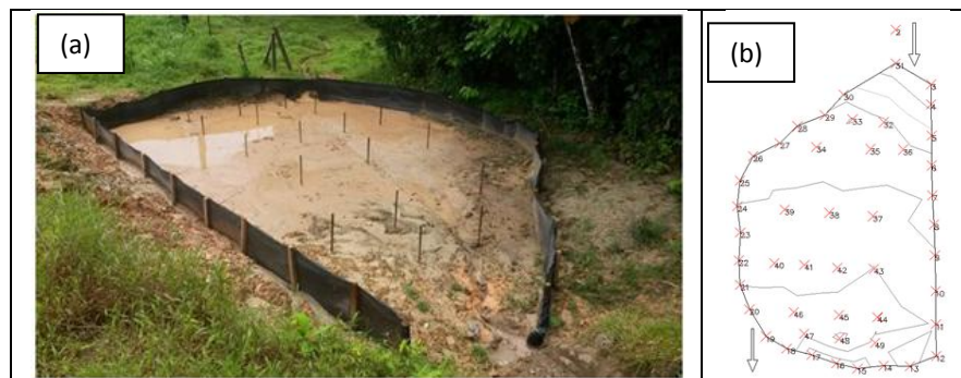
Figure 4.4 (a) Sediment trap at Site 5 on October 1, 2014. (b) Survey points and contour map of sediment surface elevations on October 22, 2014 (from the 2014 UCR Report).
