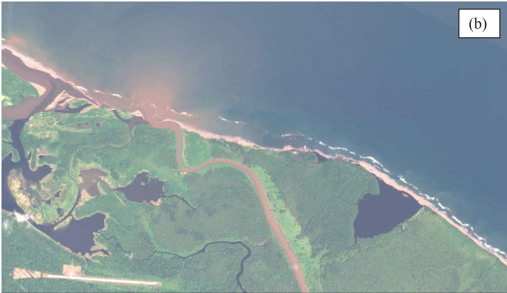
Figure 5.4 Satellite images showing that flow from the lower Rio San Juan carries turbid water with a high concentration of fine sediment into both the Bay of San Juan del Norte and the littoral sediment system of the Caribbean Sea. Image dates (a) 13 December 1997 (b) 26 November 2013.
