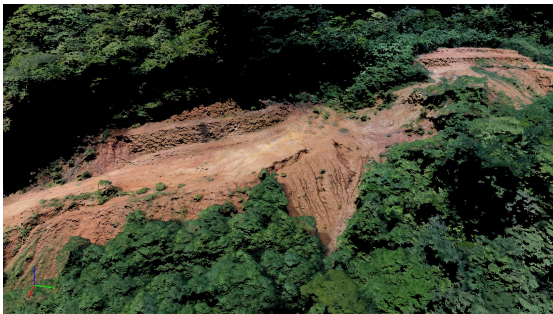
Figure 6. LAS point cloud generated during pre-processing of UAV photogrammetry.
