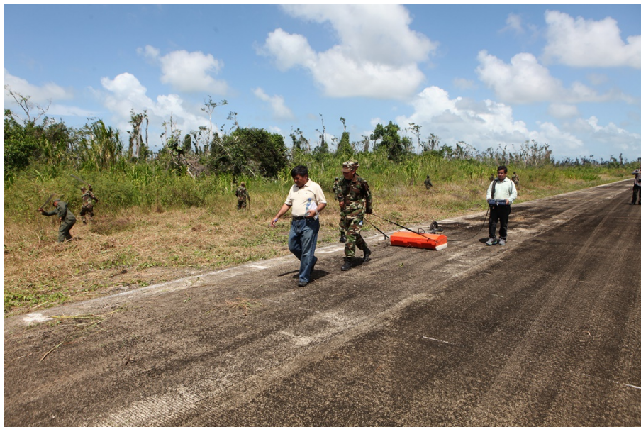
Figure 64. Prospecting for the marker of Plaza Victoria in the airstrip of the San Juan del Norte airport with a GPR (Ground Penetrating Radar) of the Nicaraguan delegation using a 200 MHz shielded antenna. The vegetation in the northern flank of the airstrip was being cleared for GPR and metal detector surveying. Image taken during the second site visit on 13 March 2017.
