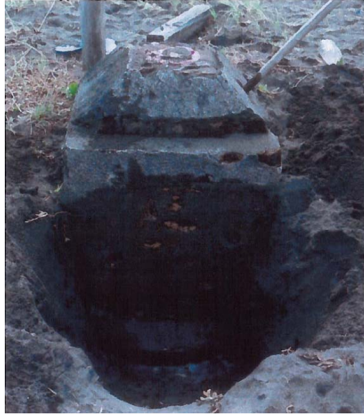
Figure 56. Marker found in the beach by the Sub-Commission on Limits and Cartography on 21 February 2003 and on 25 November 2003. The side exposed by the excavation was marked with a letter “A” accompanied by another illegible symbol. This marker was measured by both Parties for 2:50 hours with hand-held GPS devices.
