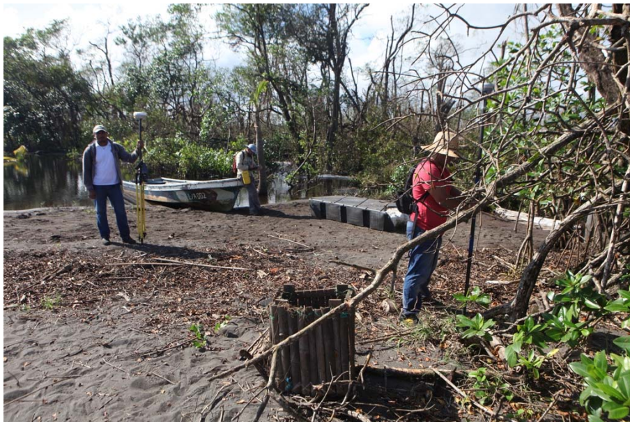
Figure 28. Point Plw measured during the first site visit at the western extremity of Los Portillos/Harbor Head lagoon. The point was located at a high-water mark defined by stranded vegetation indicating the maximum level reached by the water of the lagoon after Hurricane Otto. Image taken on 6 December 2016.
