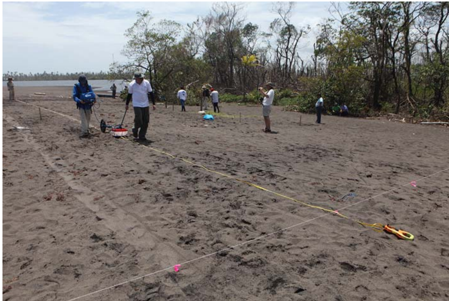
Figure 61. GPR survey carried out in an area enclosing the co-ordinates measured by Nicaragua for the marker found in 2003 submerged in Los Portillos/Harbor Head Lagoon. A total of 12 GPR profiles 27 m long were acquired with a spacing of 2 m. Pink flags indicate the starting and end points of the profiles.
