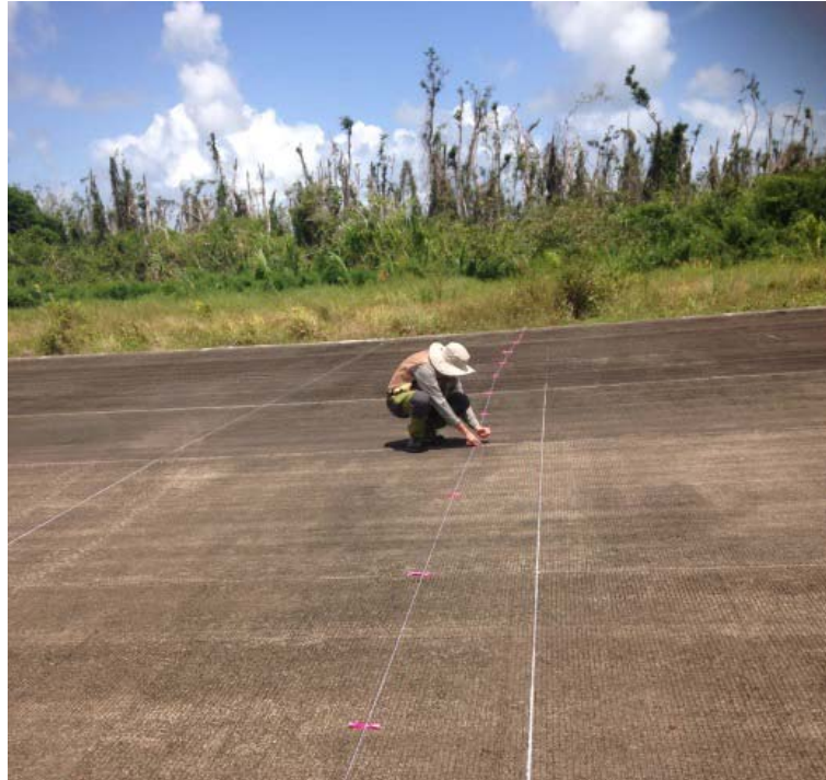
Figure 10. Placing of colored ribbons every 1.55 m on the cords marking off the eastern and western extremities of the initial research area, covering a 60 m long section of the landing strip.
