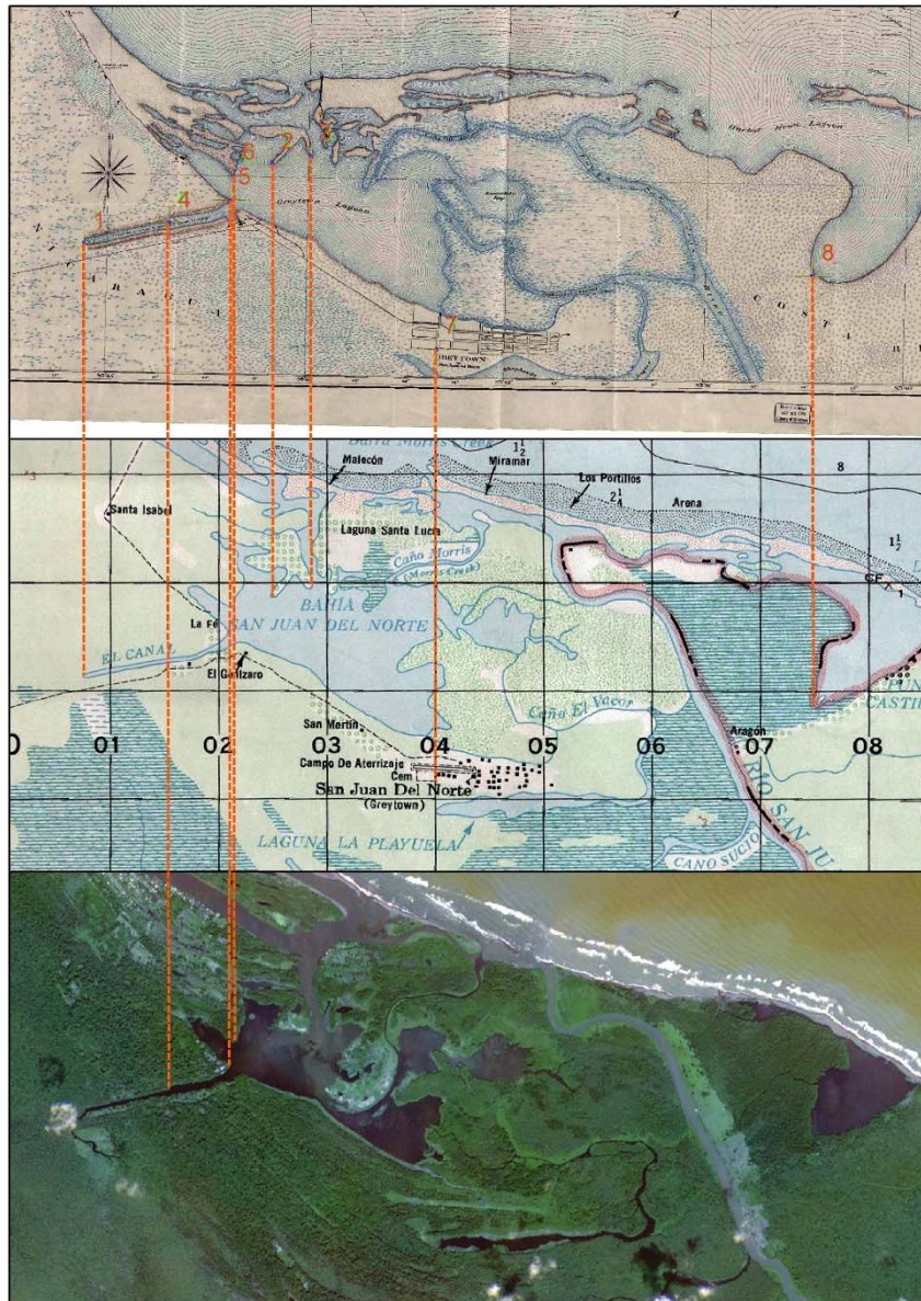
Figure 69. Ground Control Points used for georeferencing the Map of Greytown Harbor of 1899 (top) using as basemaps the Map of San Juan del Norte of 1966 (center) and a satellite image from 2009 (bottom).
