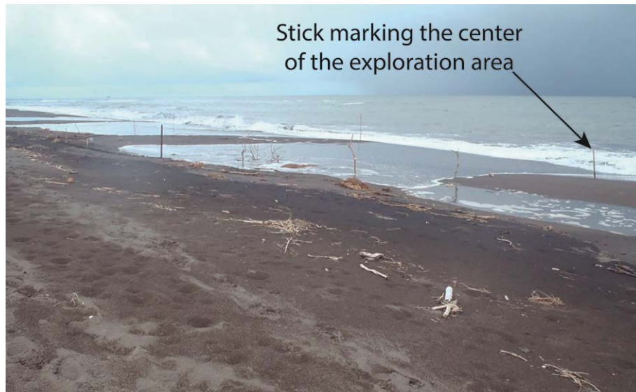
Figure 6. Exploration area around a point established assuming that the average of the co-ordinates measured on 25 November 2003 correspond to the location of auxiliary marker A_m and using the triangulation values indicated in the sketch-map included in Proceedings XX of the Costa Rica-Nicaragua Demarcation Commissions (1897-1900) .
