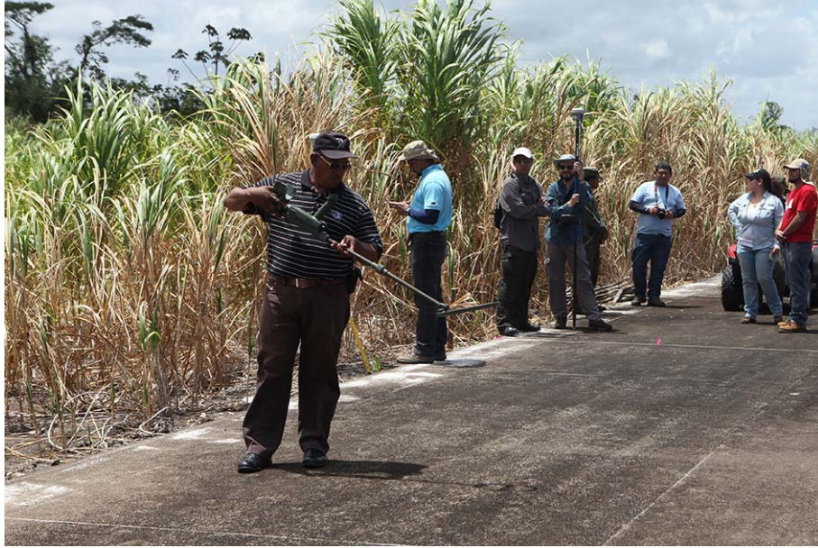
Figure 12. Surveying of the landing strip with the Nicaraguan metal detector (VALLON model VMH3CS).
