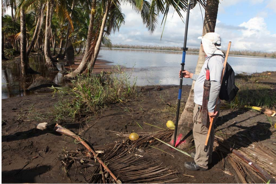
Figure 27. Point Ple located at the base of the sand spit-barrier of the Los Portillos/Harbor Head Lagoon. This point is located at the contact between the relatively stable surface covered by tree vegetation on the eastern margin of the lagoon, and the accumulation of loose sand that forms the spit-barrier. The GPS receiver of Costa Rica is located at the base of a coconut tree. The flooded coconut trees in the background reveal the high water level that reached the lagoon after Hurricane Otto. Image taken during the first site visit on 6 December 2016.
