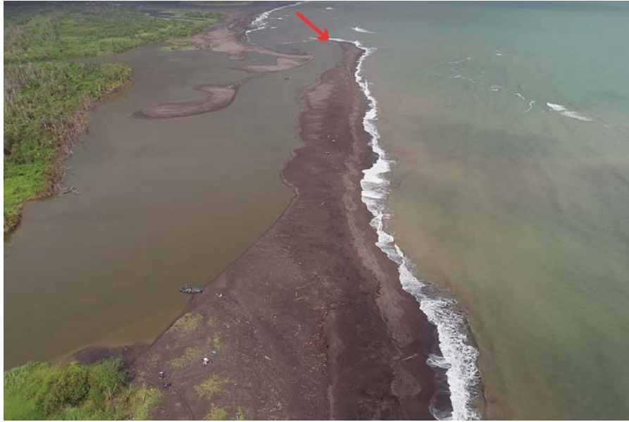
Figure 47. Spit of Isla Portillos and the mouth of the San Juan River on its eastern bank (arrow) during the second site visit. The spit experienced a significant westward growth by sand accretion between the first and the second visit (see Figure 46 for comparison). Image captured by the drone of the Costa Rican delegation in March 2017.
