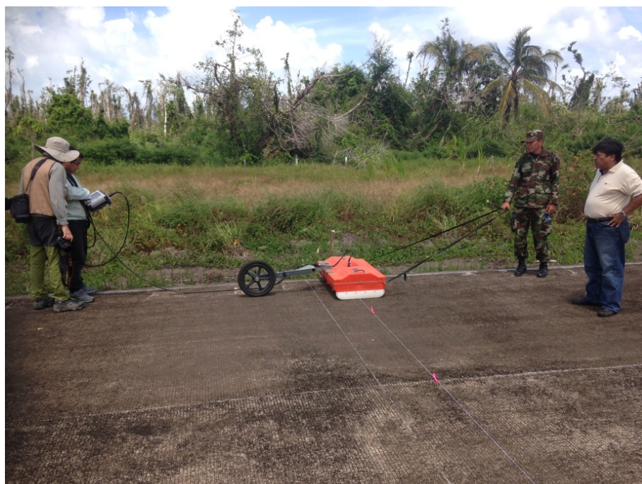
Figure 11. Acquisition by Nicaragua of GPR profiles using a GSSI system equipped with a 200 MHz shielded antenna.
