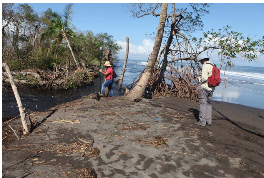
Figure 30. Topographer of the Costa Rican delegation measuring the eastern bank of the channel through which the lagoon was draining towards the sea (point Pch). On the other side of the channel the tree vegetation is in direct contact with the sea waves. Image taken during the first site visit on 6 December 2016.
