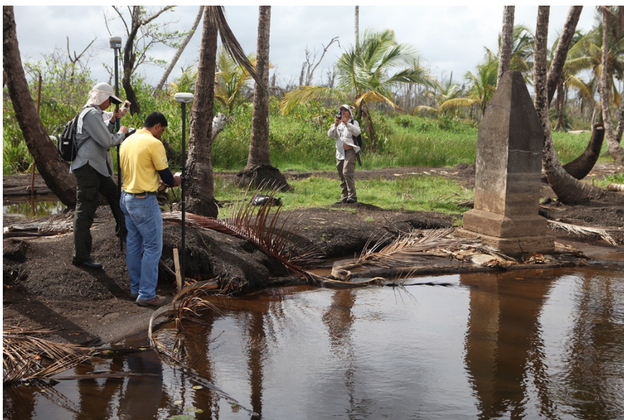
Figure 32. Image of Point Ple2, which represents the easternmost edge of the water body of Los Portillos/Harbor Head Lagoon on its northeast corner during the second site visit. The point was marked with a wooden stick, being measured by a topographer from Nicaragua (right). The monument to the right corresponds to a marker whose designation ( \Delta and a reversed s as subscript, referred to by the Parties as the “A2” Marker) has not been identified in the Proceedings of the Costa Rica-Nicaragua Demarcation Commissions of the end of the 19 th century. Image taken during the second site visit on 15 March 2017.
