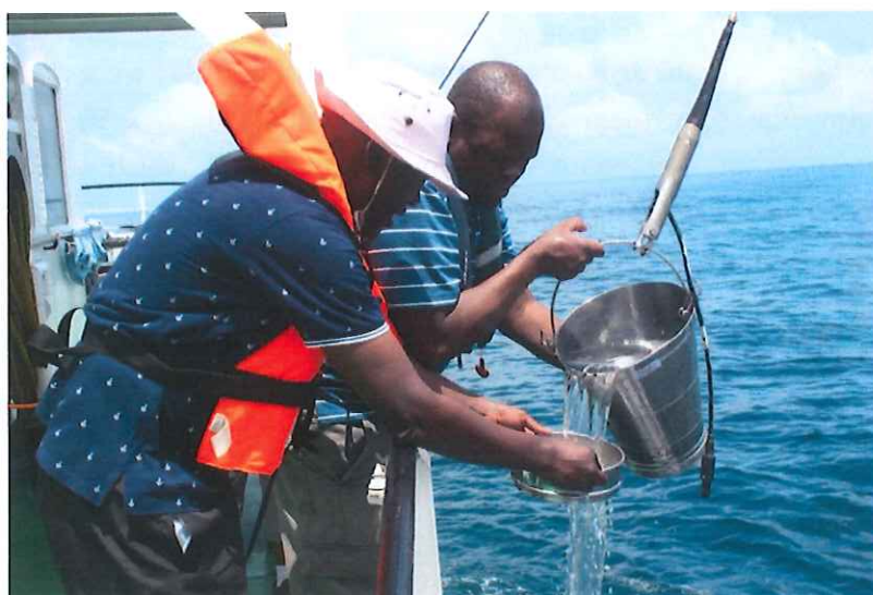
Plate 1: Bulk surface seawater sampling for MPs
