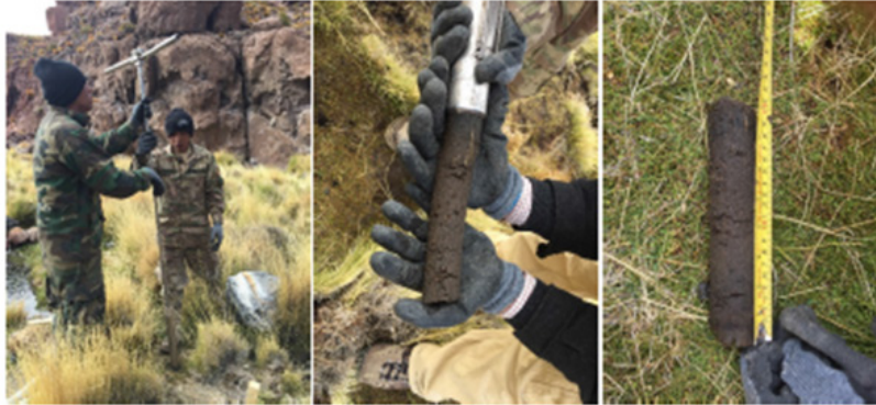
Figure 4. From left to right: drilling, extraction and measurement of samples to determine soil moisture.
