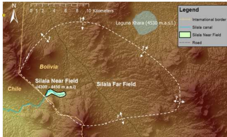
Figure 2-3 Approximate extents of the Silala Far Field (the groundwater catchments likely to contribute to Silala Springs System)
