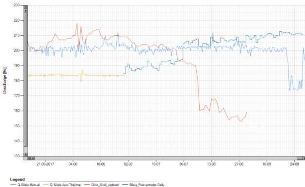
Figure C-16 Long-term series of Silala flows close to border In Chile and at the desiltation chambers and at DGA's Siloli Station in Chile Close to the border upstream of the Fcab offtake. Data from 2017.
