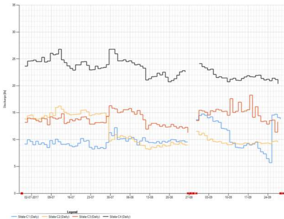
Figure C-8 Measured flows in weirs C1-C4 located in the Southern wetland averaged to daily values and with obviously spurious data replaced by missing values (red crosses)
