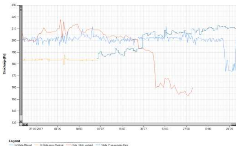
Figure 16 Long-term series of measured Silala Canal flows close to border, May-September 2017. Blue curve: manual readings C7, yellow curve: automatic floaters instrument C7, turquoise curve: daily average from the new pressure sensor C7; red curve daily data from DGA's Siloli station just downstream of the border.
