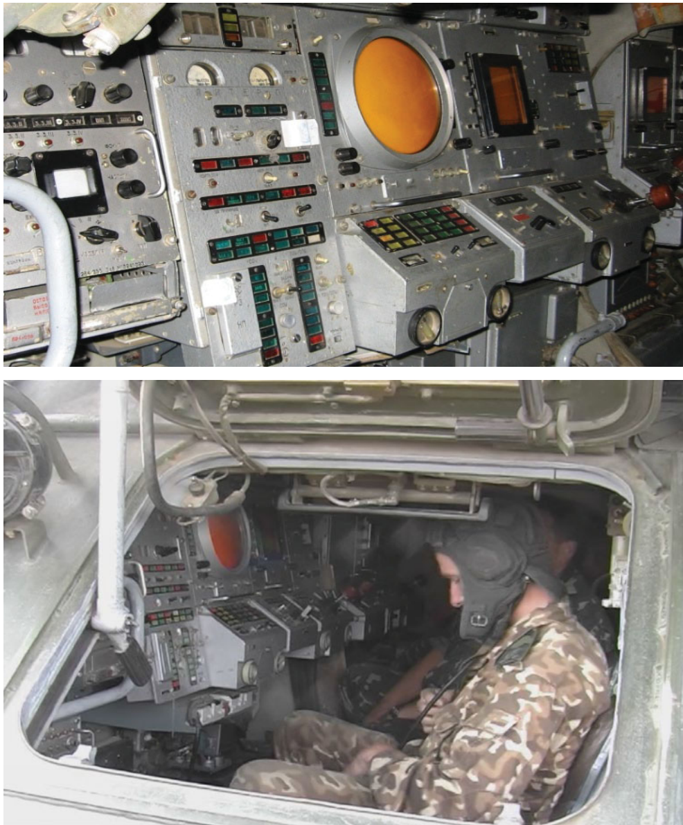
Figure 5. Workstations of the combat crew of the Buk-M1 TELAR (9A310M1) 16
