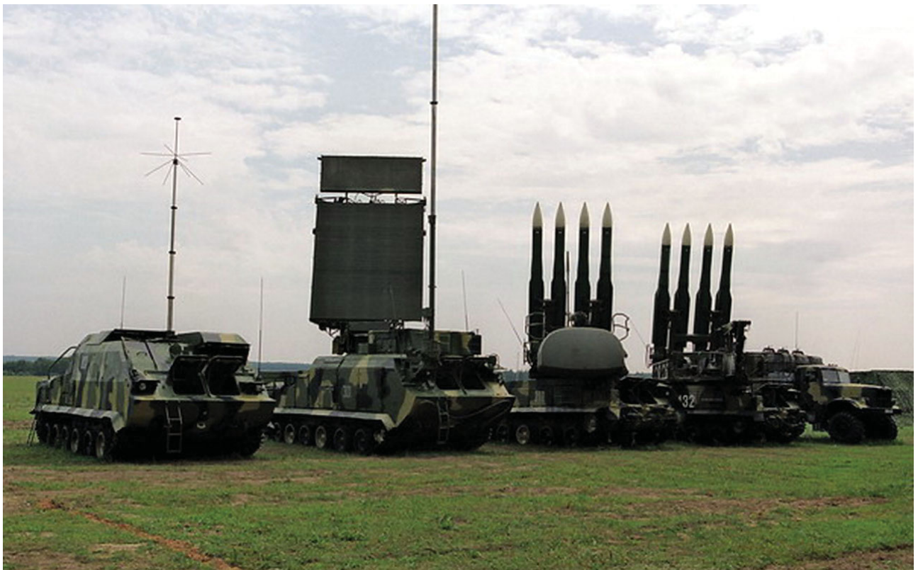
Figure 1. Buk-M1 surface-to-air missile system, including combat control center (left), target locator (second from left), TELAR (in the middle), launcher-loader (second from right), and transport vehicle (right). 7
