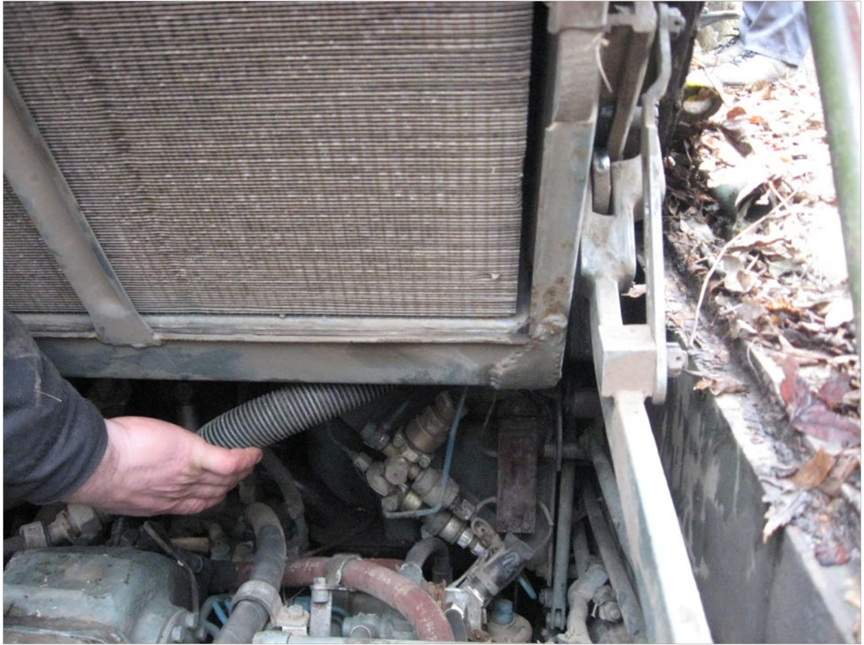
Air valve “ИЛ” in the transmission compartment
