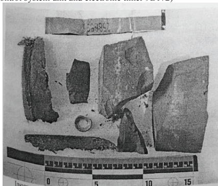
Illustration No. 23. Contents of safe pack No. 2586595 (fragments of graphite liner of nozzle cluster)
