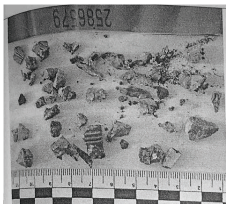
Illustration No. 13. Contents of safe pack No. 2586579 (fragments of 9N235 warhead fragmentation element)
