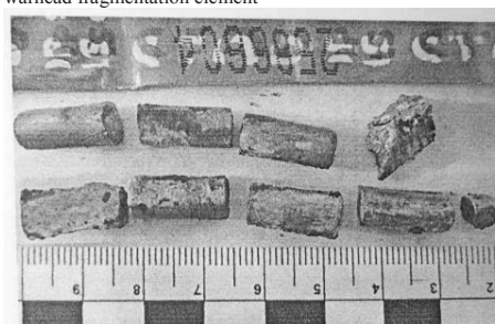
Illustration No. 16. Contents of safe pack No. 2586604 (fragments of 9N235 warhead fragmentation element)
