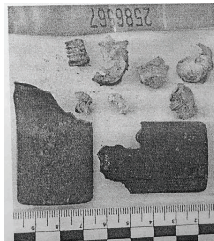
Illustration No. 18. Contents of safe pack No. 2586567 (fragments of 9N235 warhead fragmentation element)
