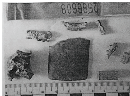
Illustration No. 12. Contents of safe pack No. 2586608 (fragments of 9N235 warhead fragmentation element)
