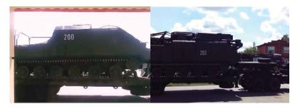
Left: Buk-M1 command vehicle 200; right: Buk-M1 Snow Drift radar 201.
