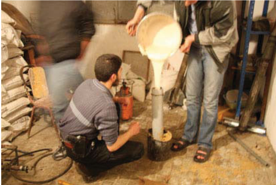
Figure 9.2 Improvised rocket fuel being poured into a plastic casting container to cool and cure. The container is then cut away and the casting is placed inside the rocket. [26]
