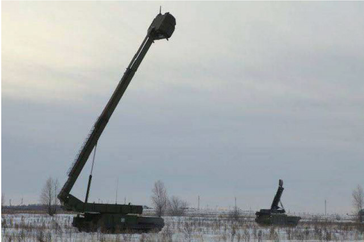
9S36 Buk-M2 radar system for target illumination and missile guidance. The antenna is raised to its operating position.
