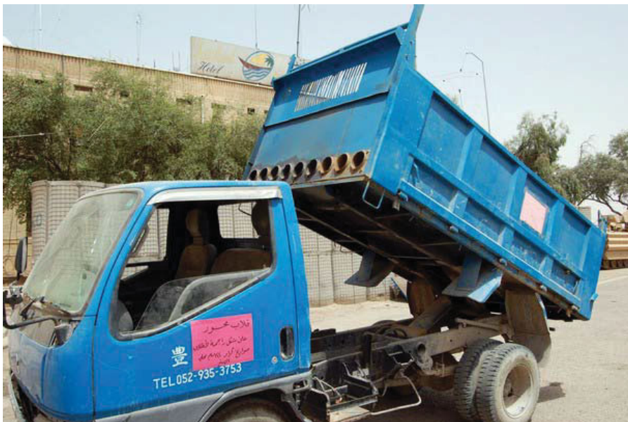
Figure 9.6 A small truck discovered in the Basrah area in Iraq displaying built-in rocket launching tubes in the floor of the platform. It is supposed that this unit is able to fire 122 mm BM-21 rockets. [29]
