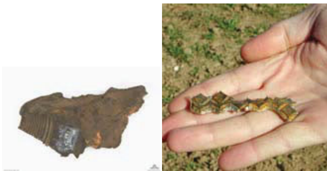
Figure 8.1 Examples of fragments. Left – a natural fragment, right – prefragmented fragments[17]
