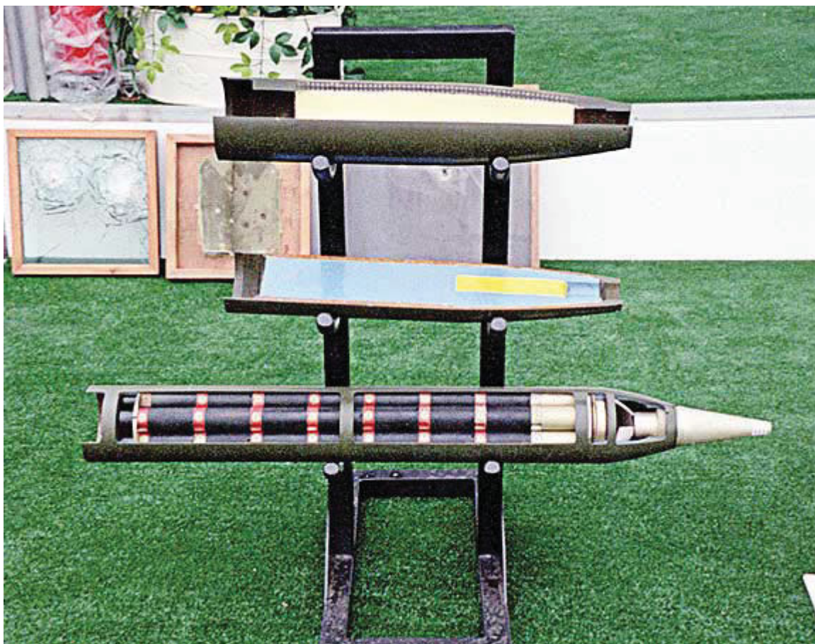
Figure H.2 Chinese warheads for 122 mm. From above: HE with enhanced fragmentation effect (metal spheres); ordinary HE, and DPICM warhead. ( http://rbase.new-factoria.ru/search/index7.htm )
