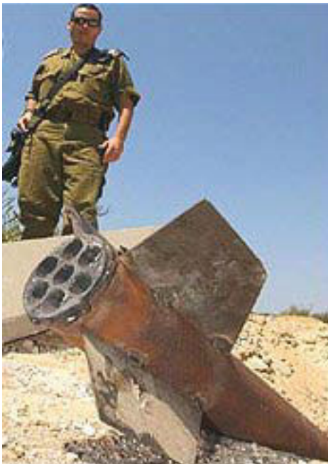
Figure 9.9 Finned and spin stabilized rocket wreck found in Israel.
