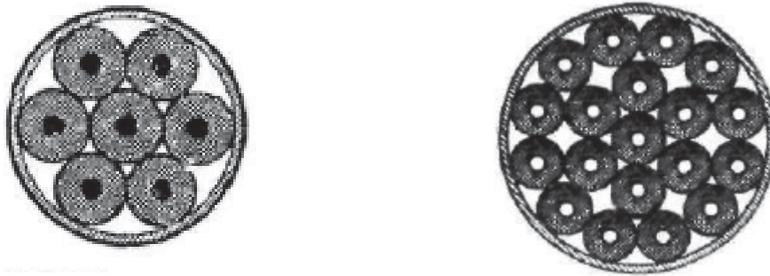
Figure 6.2 Cross sections of old propellant grain configurations (left - 140 mm; right - 240 mm)
