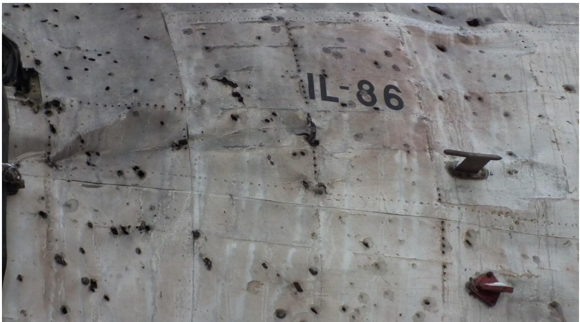
Figure 5.29 - Port outside the windows of the aircraft commander with signs of deformation of the outer skin, elements of the framework and thermal burn
