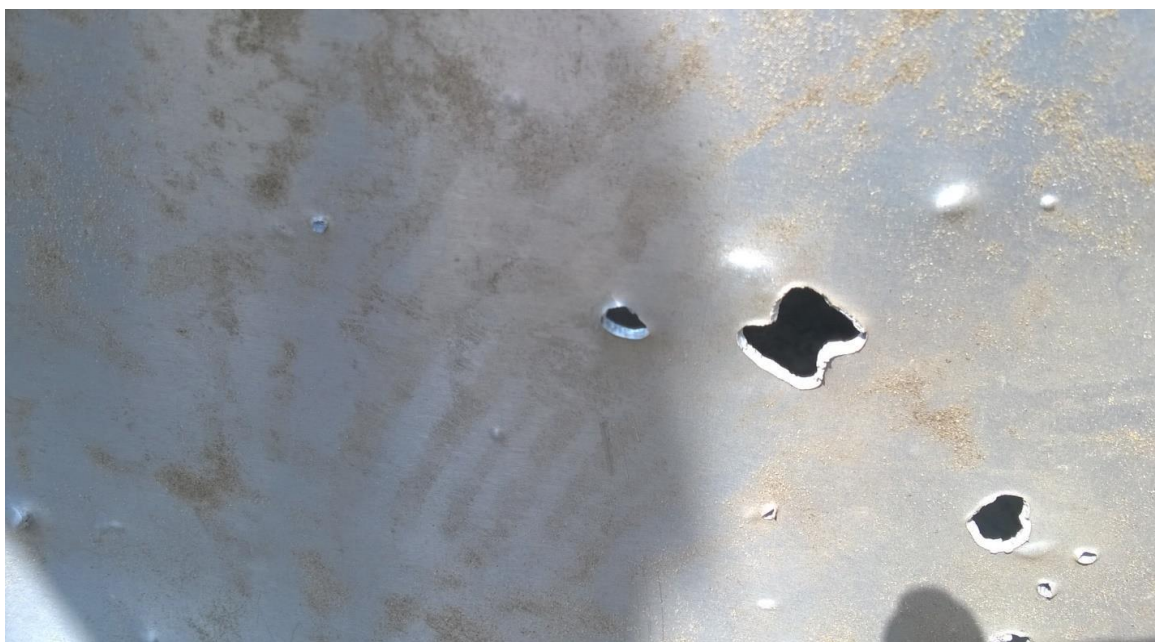
Figure A.197 - Exit holes and non-penetrating damage (view from the back of the shield)
