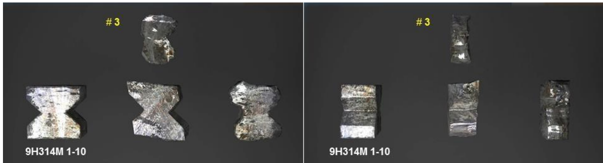
Figure 8.19 - Appearance of mock-ups of fragment #3 (top) and 9H314M 1-10 projectiles after the tests (bottom)
