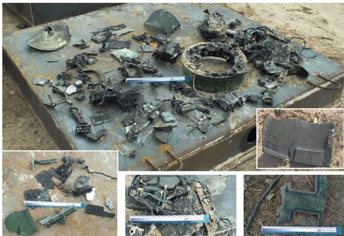
Figure 9.6 - Fragments of the 9M38M1 missile compartments
