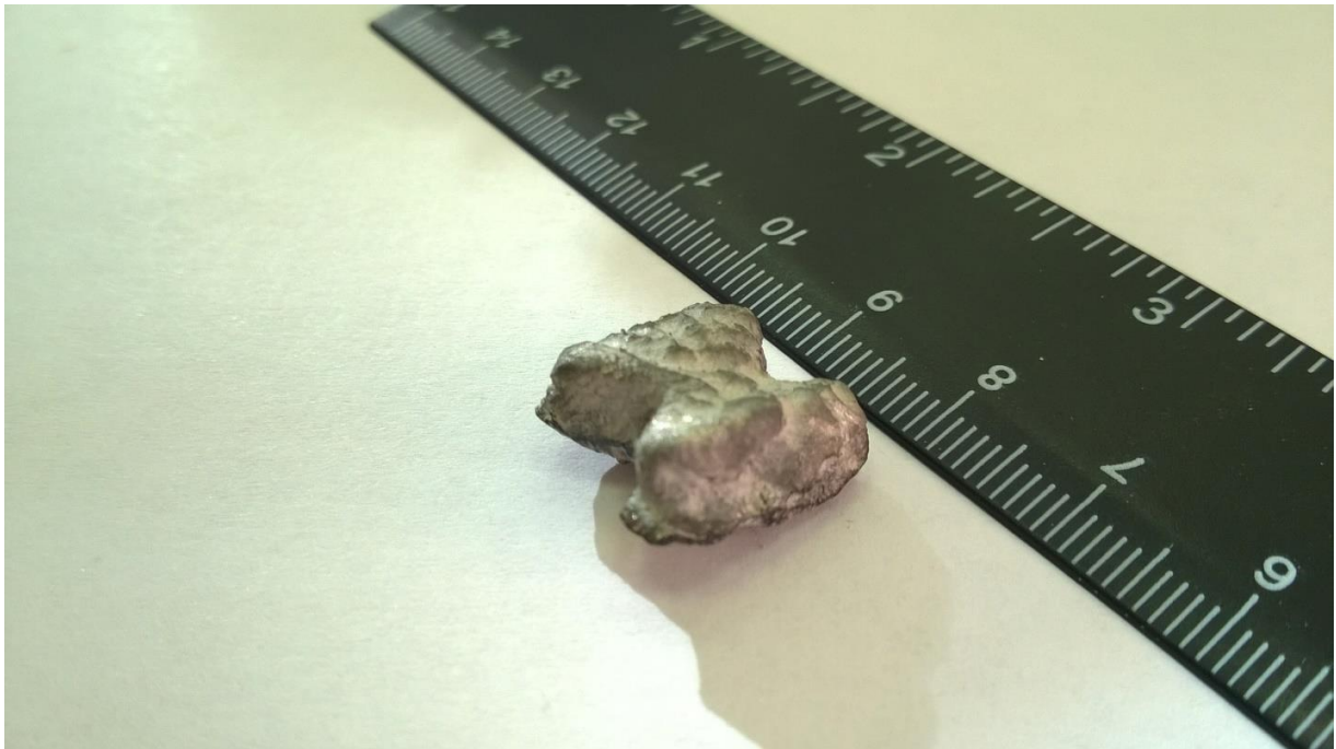
Figure 8.8 - 9H314M 1-10 projectile ("bowtie")
