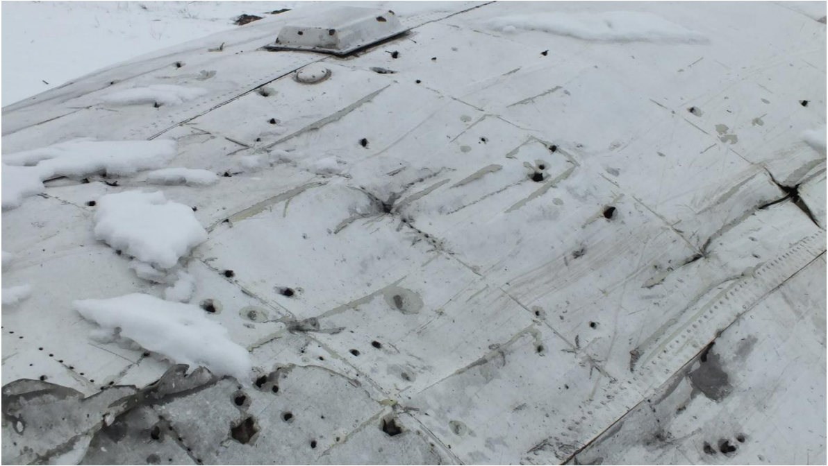
Figure 5.59 - Cockpit roof at the level of the front left passenger door L1 (top view). The roof fragment shows that through-and-through holes caused by ready-made projectiles are present on both left and right side on the roof
