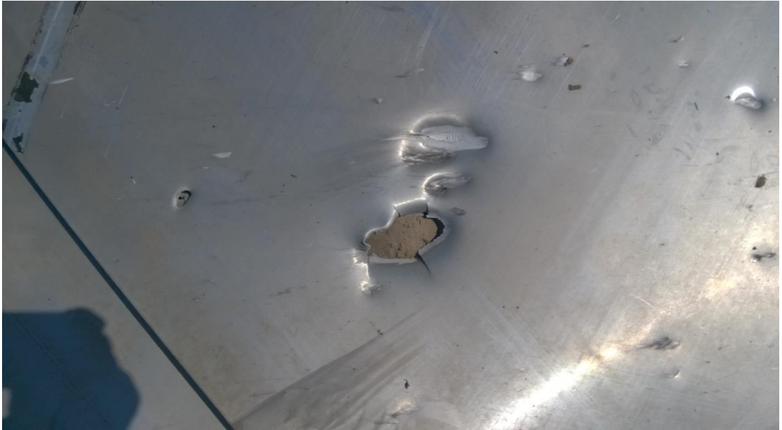
Figure A.176 - Piercing and non-penetrating damage caused by hull fragments
