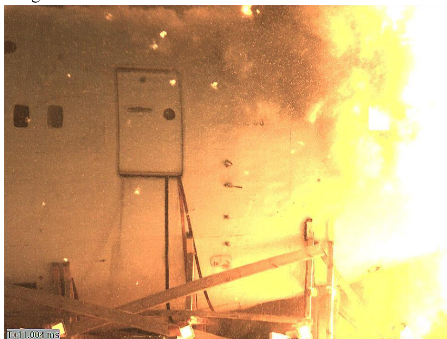
Figure 4.23 - Detonation of the 9H314M warhead
