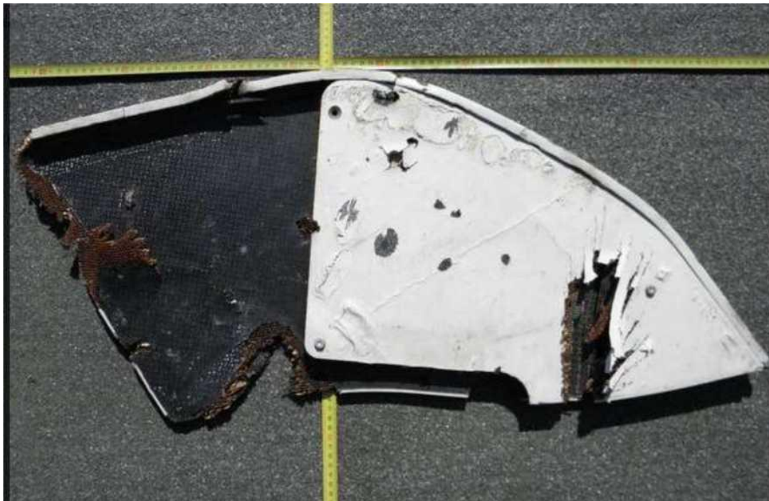
Figure 5.1.43 - Fragment of passenger compartment luggage rack with (presumably) fragmentation damage
