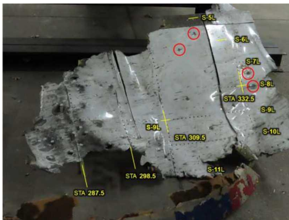
Figure A.1.19 - Fragment of the roof and top of the port side behind the cockpit. The fragmentation damage is located between bulkheads STA 309.5 and STA 332.5, which is almost 3 metres further than the DSB 'reference'
