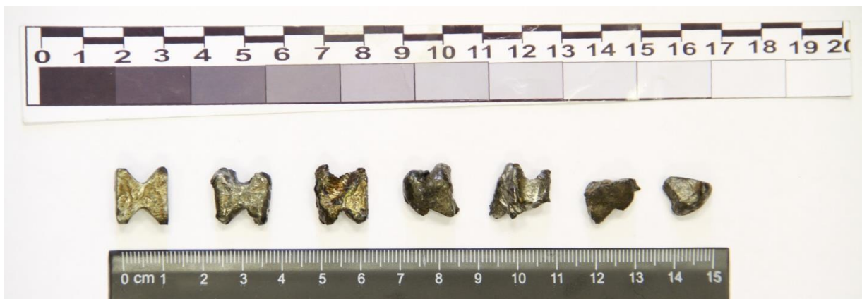
Figure 8.3 - Extracted 9H314M 1-10 projectiles (top view)
