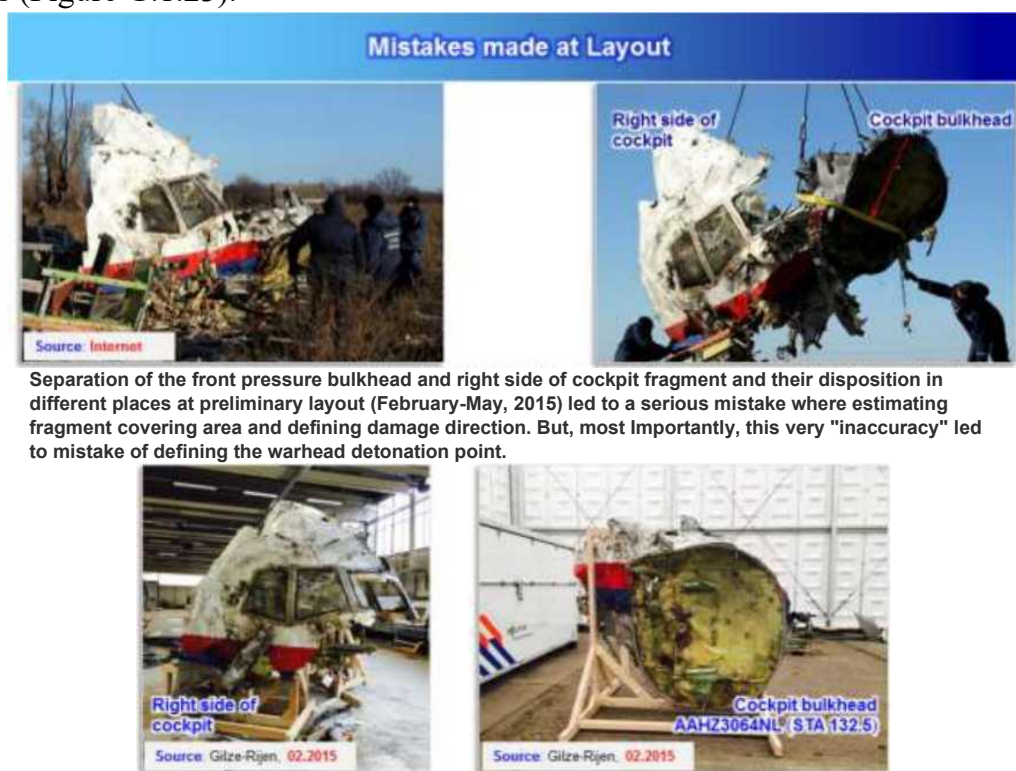
Figure G.1.23 - Separation of the forward pressure bulkhead with a fragment of the starboard cockpit and their subsequent location in different rooms led to a serious error in determining the detonation area
