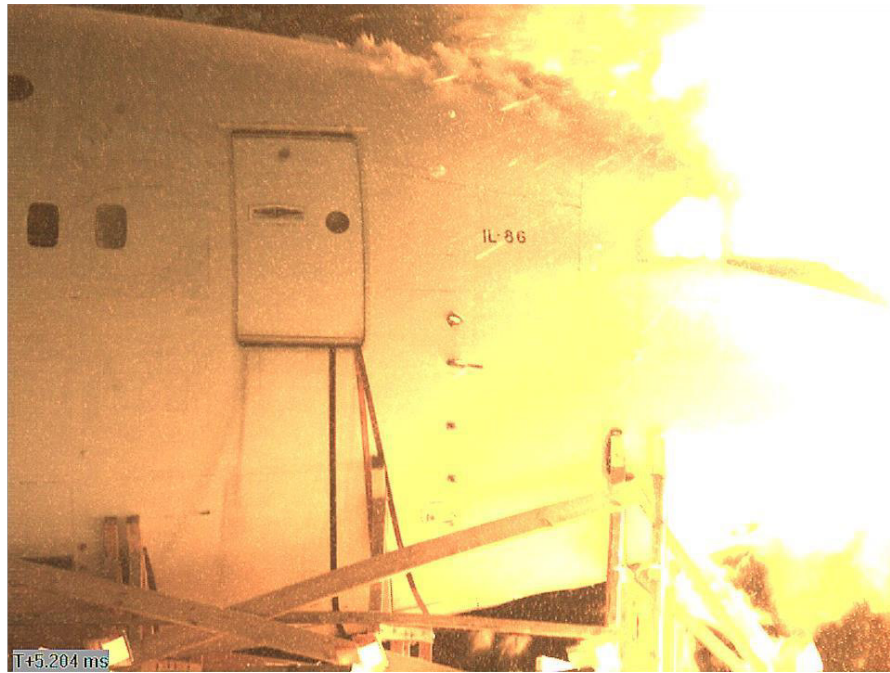
Figure 4.9 - Detonation of the 9H314M warhead
