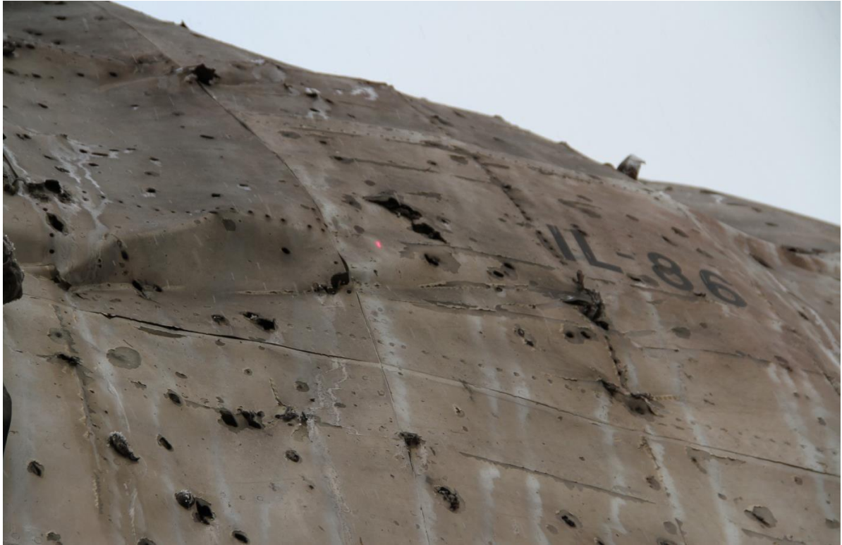
Figure 5.29 - Port outside the windows of the aircraft commander with signs of deformation of the outer skin, elements of the framework and thermal burn
