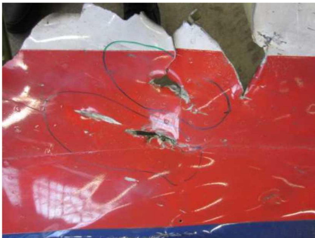
Figure 5.1.14 – Though-and-through and part-through non-penetrating damage at the lower boundary of the coverage field near bulkhead STA 265.5
