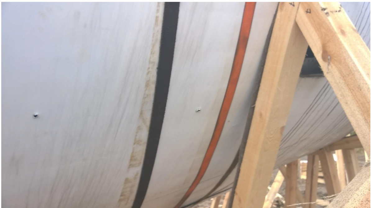
Figure 5.102 - Exit holes and non-penetrating damage
