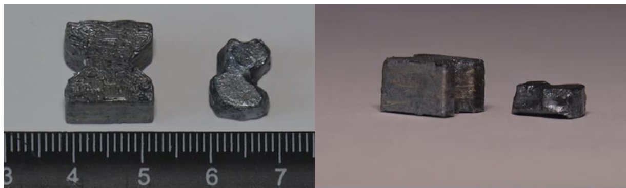
Figure 8.20 - Comparison of sizes of fragment #3 (from DSB Report) and 9H314M 1-10 projectile
