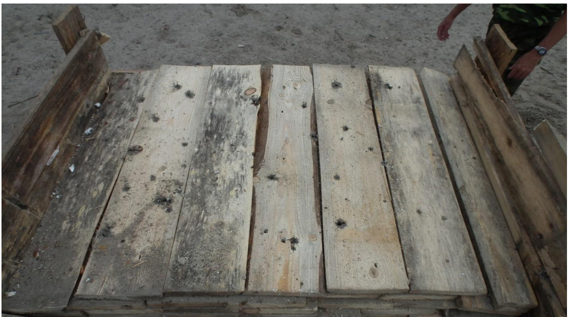
Figure A.38 - Third barrier of trap L1 (boards with a total thickness of 750 mm) after the testing
