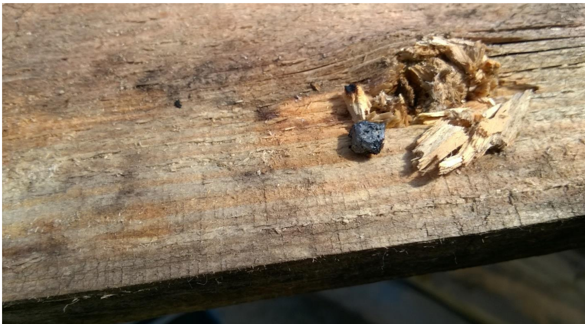
Figure A.49 – Removal of a projectile lodged in trap L2
