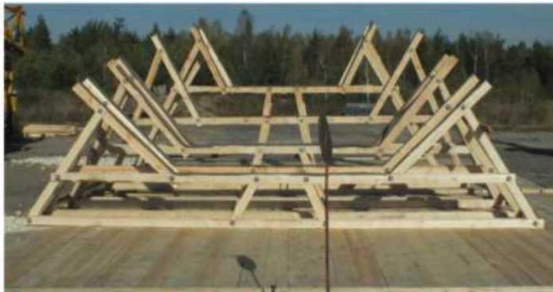
Figure C.3 - Stand to align cockpit roof contours. (Figure from Almaz-Antey Experiment Report, page 12 of 190)
