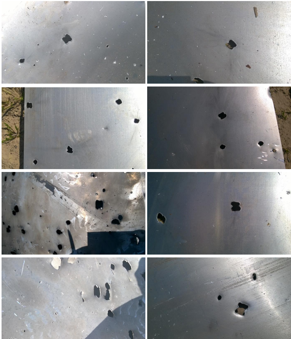
Figure A.168 - Characteristic "butterfly"-shaped holes
