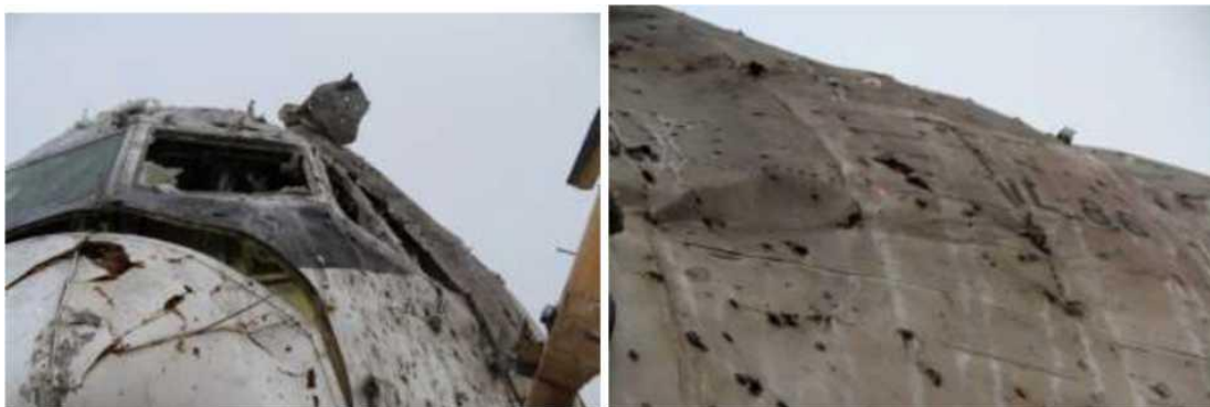
Figure A.4.16 - Deformation of the outer skin of the IL-86 target aircraft
