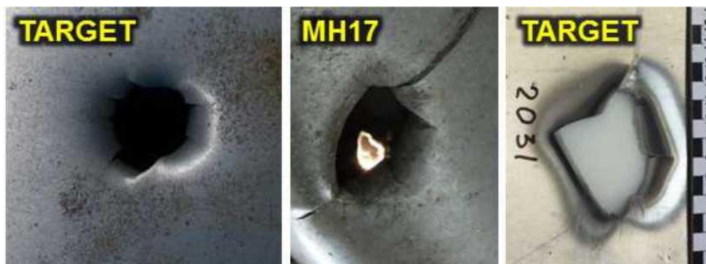
Figure 5.1.58 - "Large" holes caused by preformed fragments: left - from tests involving a 9H314M warhead; middle - on a Boeing 777 air intake; right - from special experimental studies assessing the penetrating effect of preformed fragments
