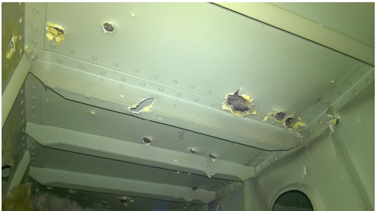
Figure 5.131 - Through-and-through holes in the cockpit floor (bottom view)
