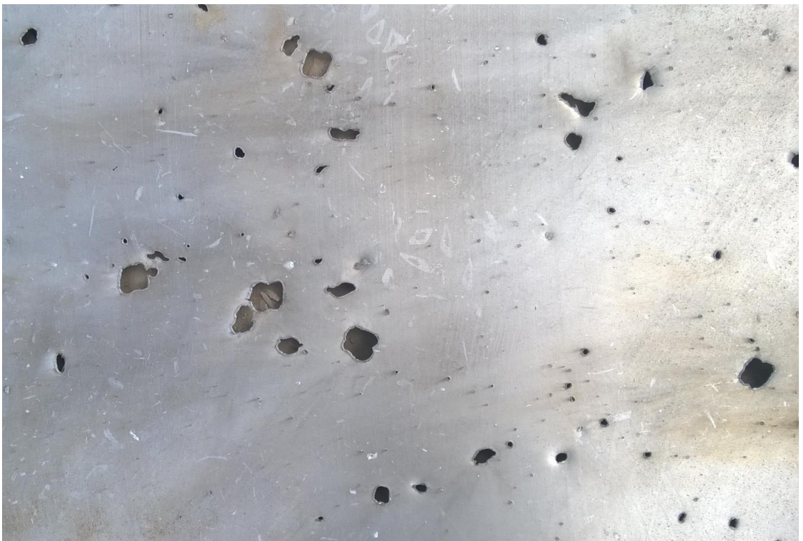
Figure A.182 - Target fragment with micro-crater marks and thermal oxidation
