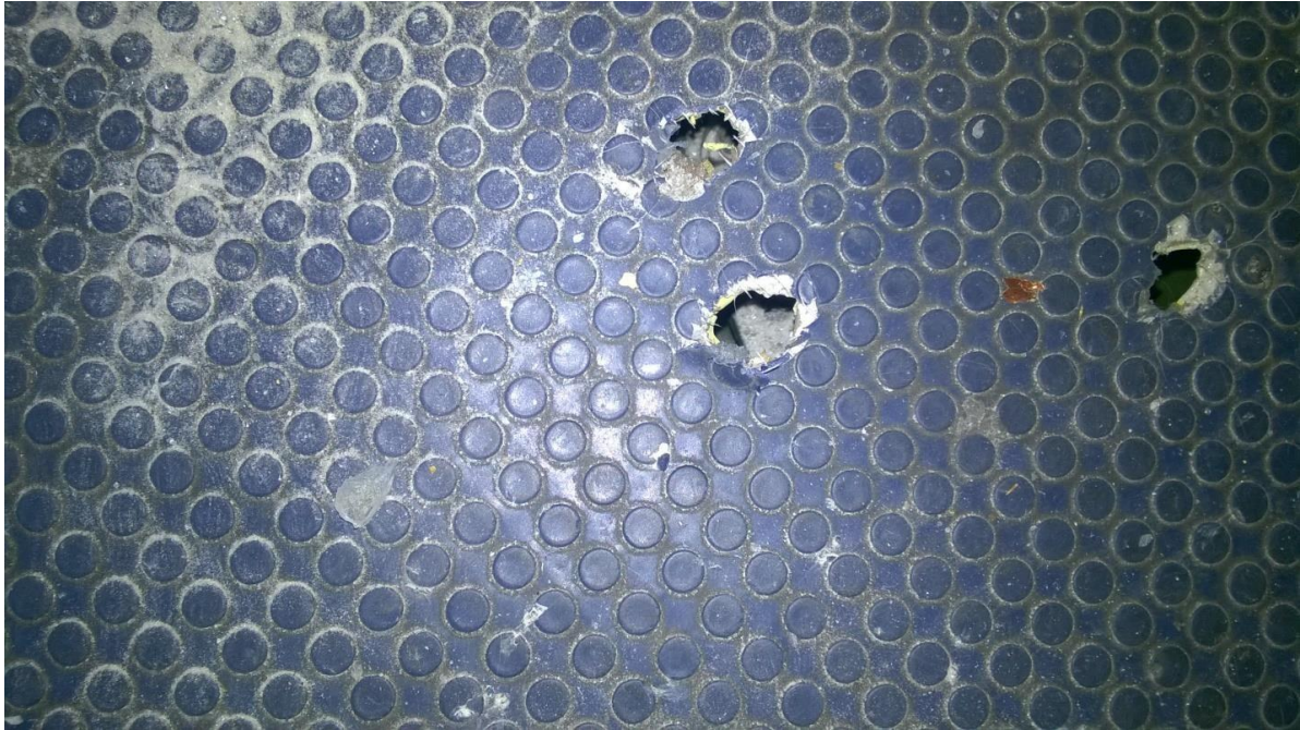
Figure 5.124 - Through-and-through holes in the cockpit floor (starboard)
