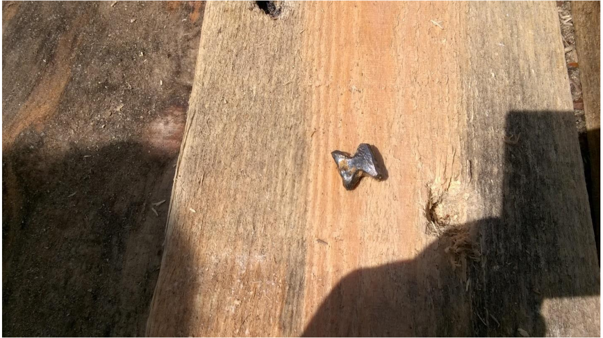
Figure A.47 - Removal of 9H314M 1-10 projectile lodged in trap L1
