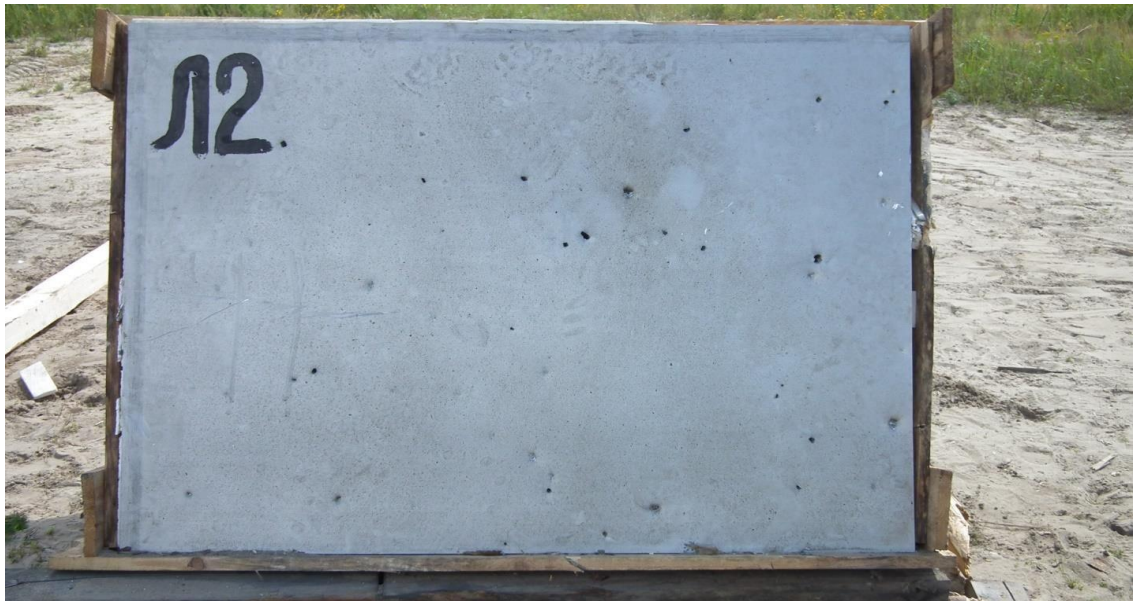
Figure A.39 - General view of trap L2 and first barrier (2.0 mm thick sheet of aluminium alloy AMg6M) after the testing
