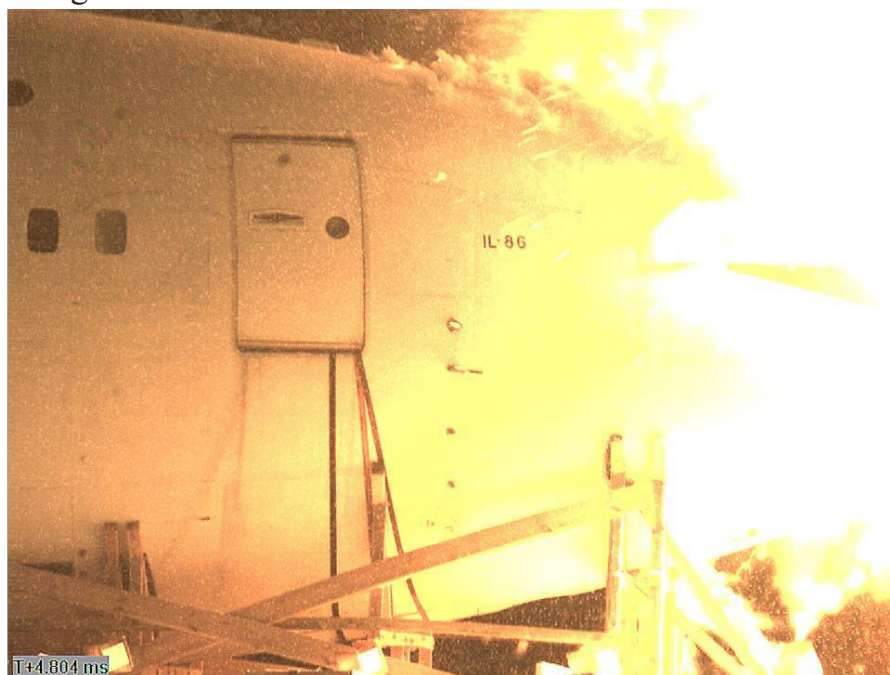
Figure 4.7 - Detonation of the 9H314M warhead
