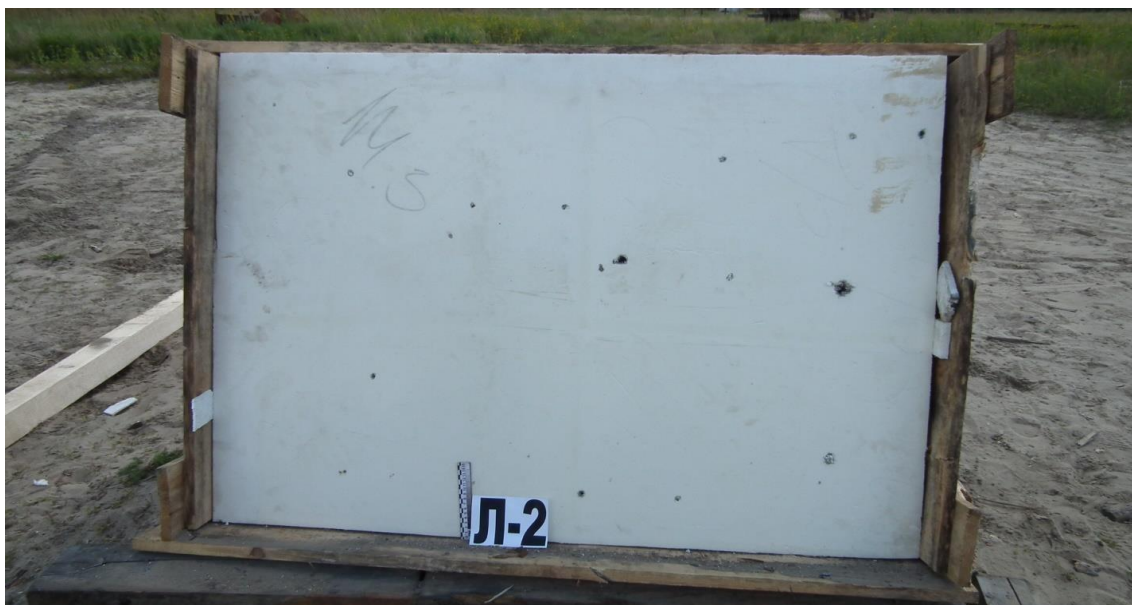
Figure A.41 - Second barrier of trap L2 (second layer of foam plastic PS-1-150) after the testing
