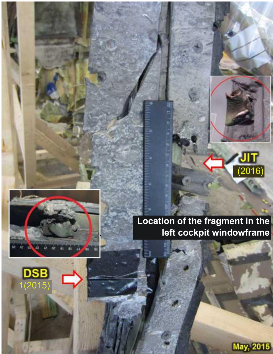
Figure G.5.3 - Two different 'metal fragment' detection locations under the hold-down bar of the second window of the aircraft commander (DSB, 2015); in the third windowframe break (JIT, 2016)
