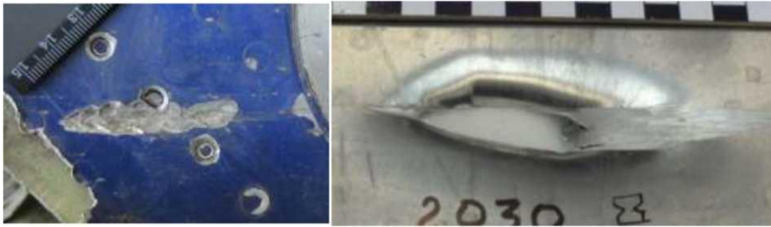
Figure A.3.9 - Exterior view of non-penetrating ricochet damage: on F.9 fragment of the left side of a Boeing 777 (left) and on the barrier after interaction with preformed fragments at an angle of 5° to the firing line (right)
