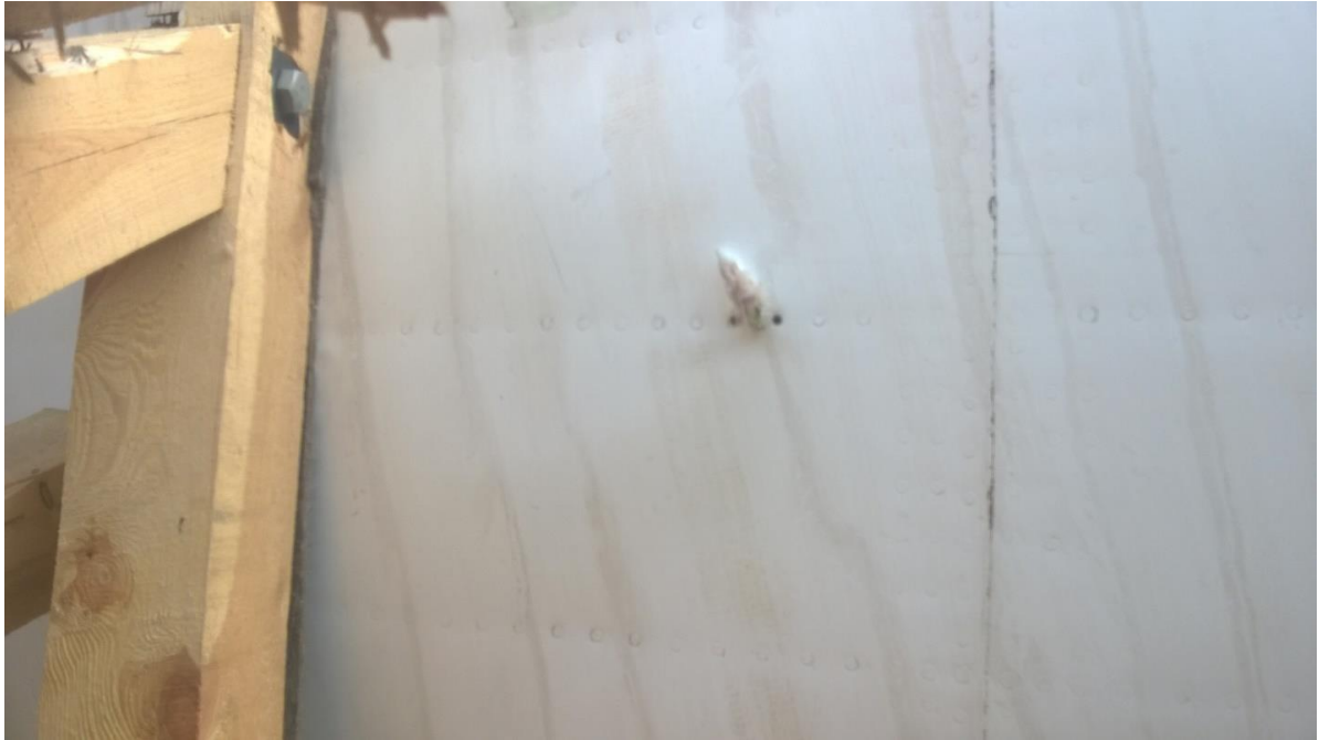
Figure 5.101 - Exit holes and non-penetrating damage
