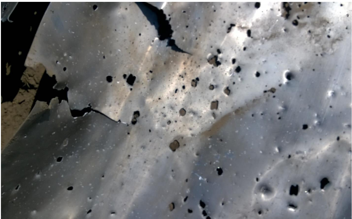
Figure A.187 - Target fragment with traces of deformation and rupture of skin sheets
