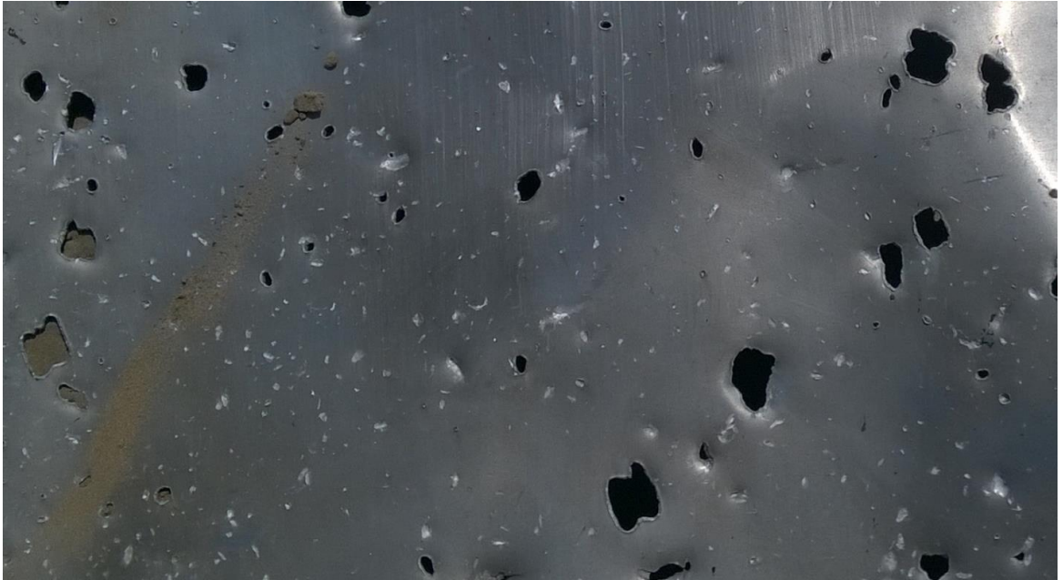
Figure A.188 - Fragment of target with marks of secondary damage
