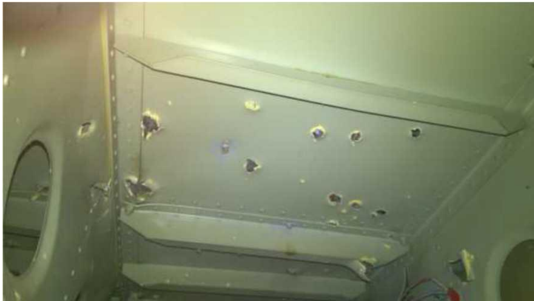
Figure B.3.17 - Example of through holes in the cockpit floor and framework of the B-86 target aircraft cockpit floor
