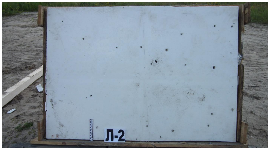
Figure A.40 - Second barrier of trap L2 (first layer of PS-1-150 foam plastic) after the testing
