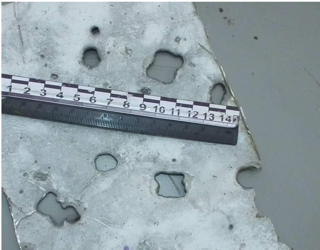
Figure 6.9 - Appearance of characteristic butterfly-shaped holes in a fragment of the cockpit roof (external view)
