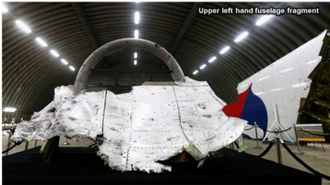
Figure G.1.8 - Fragment of the roof and top of the port side (front) and toe of the left engine air intake (rear) were located elsewhere in the final reconstruction
