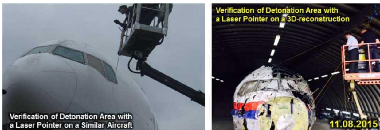
Figure 5.2.2 - Verification of the location of the detonation point area: left - on the reference aircraft (Boeing 777-200); right - on the 3D reconstruction in the hangar (Gilze-Rijen)
