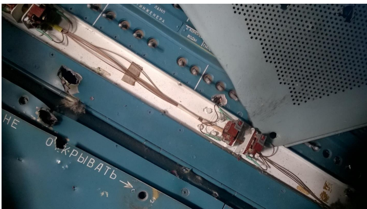
Figure 5.115 - Damage to the flight engineer's control panel (starboard side of the cockpit)
