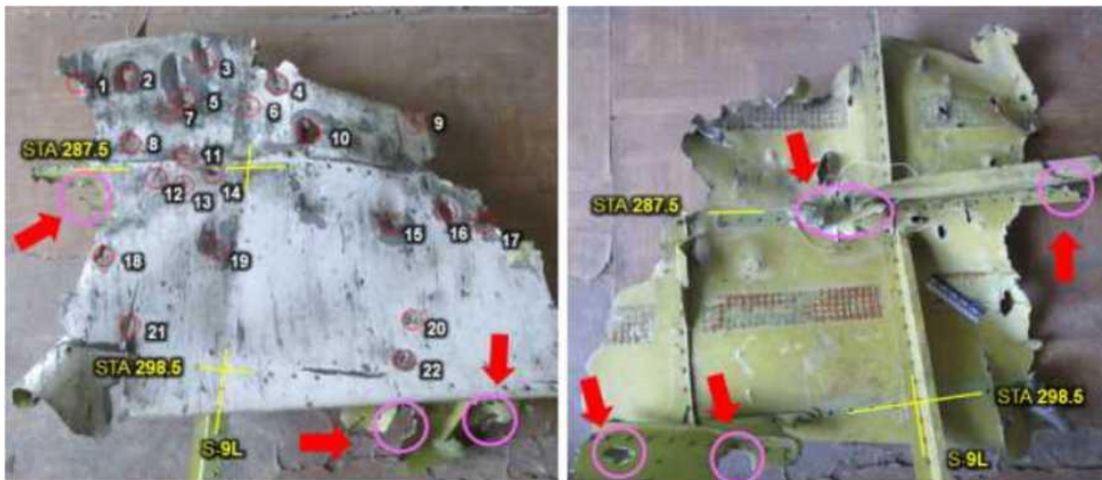
Figure F.4 - Fragment of upper port side: external (left) and internal (right) views. Multiple penetrations in bulkheads STA 287.5 and STA 298.5 caused deformation and failure of the structural members (red arrows indicate characteristic damage)
