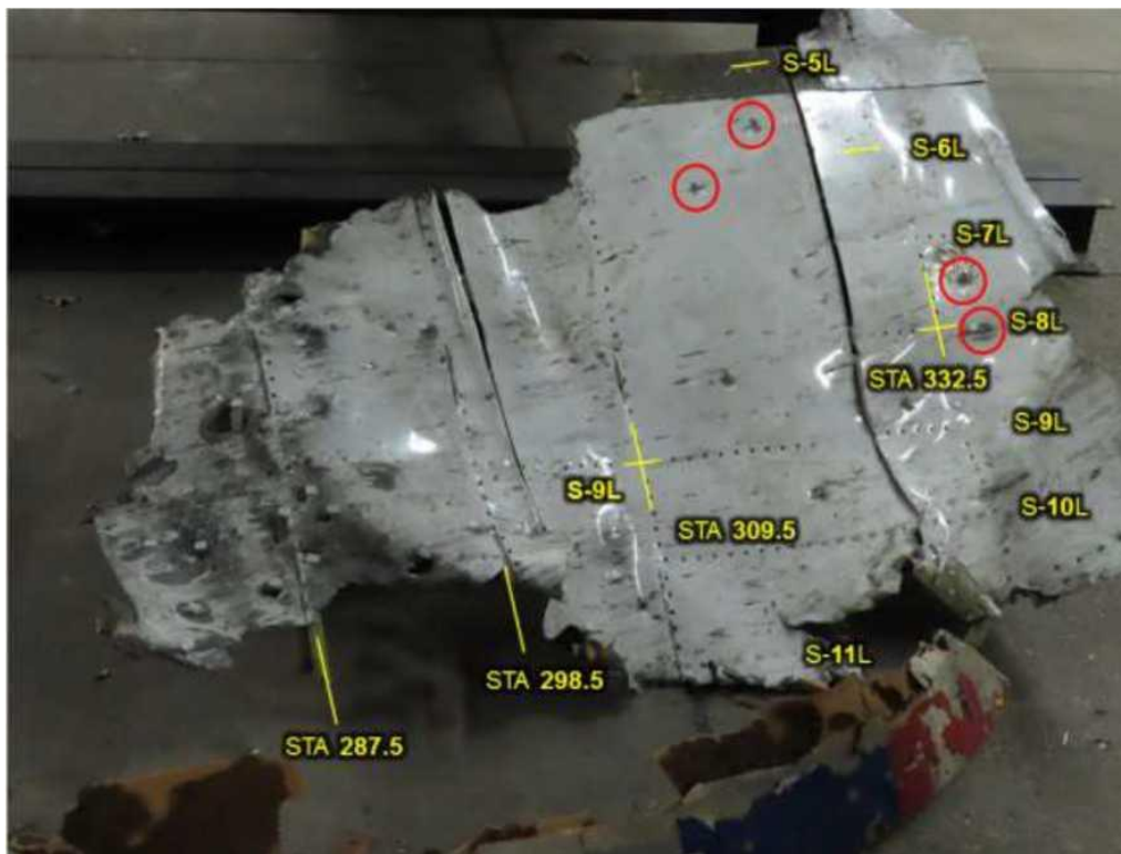
Figure F.5 - At the rear of the fragment, fragmentation damage is located between bulkheads STA 309.5 and STA 332.5, which is almost 3 metres beyond the accepted "reference" damage
