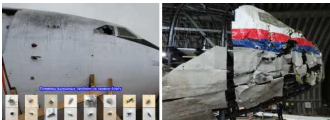
Figure A.4.3 - Examples of through-hole exit holes on the starboard side of the IL-86 target aircraft (left) and no exit holes on the starboard side of the Boeing 777 (right)
