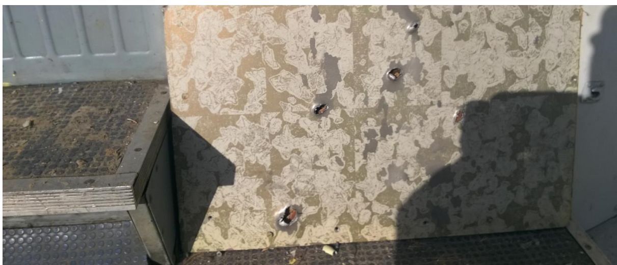
Figure 7.10 - Exit holes in the lower right-hand side of the first passenger compartment (rear view)
