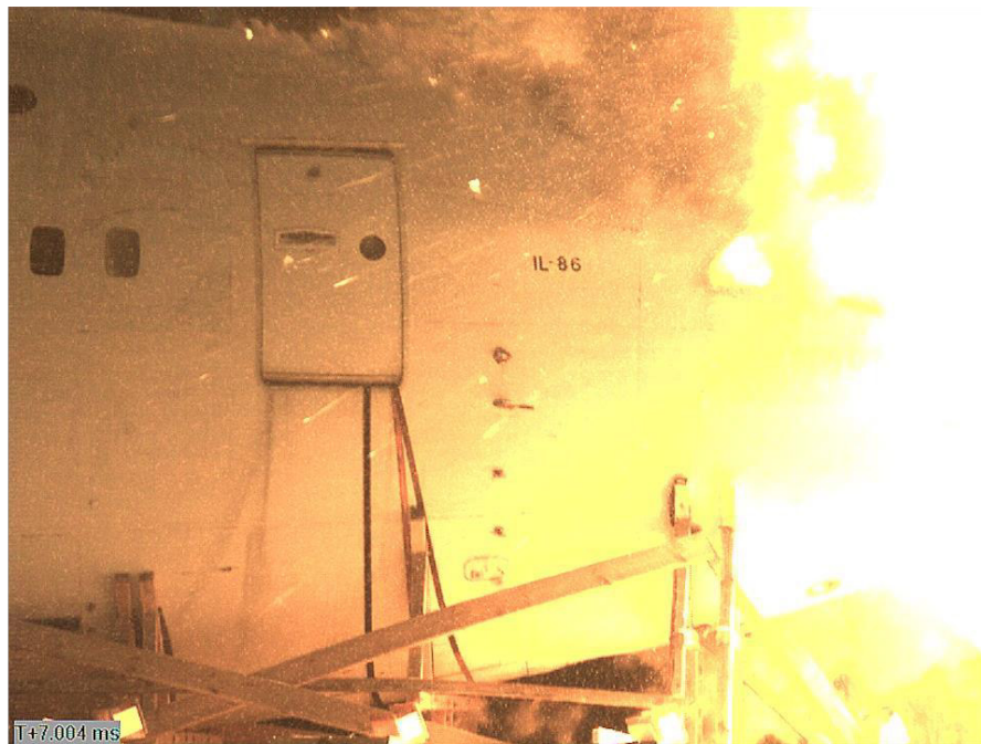
Figure 4.15 - Detonation of the 9H314M warhead
