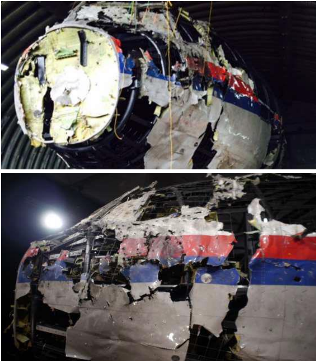
Figure 5.1.68 - Destruction and deformation of the aircraft nose structure
