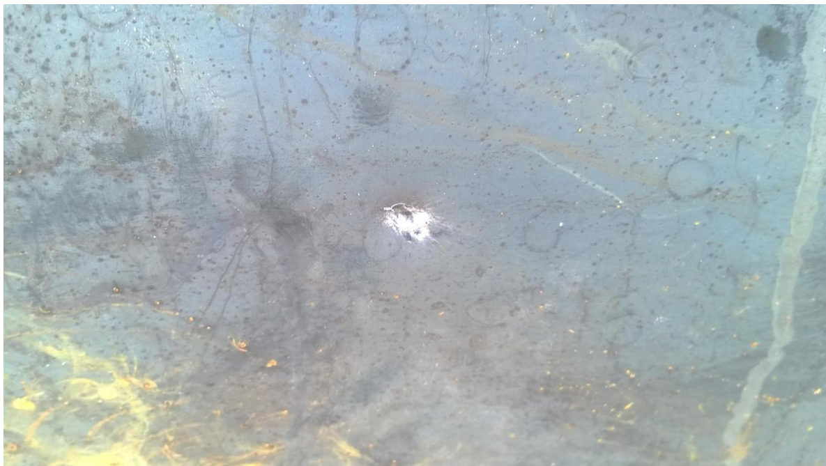
Figure A.179 - Non-penetrating damage to target No. 6M.D (left engine) caused by a hull fragment
