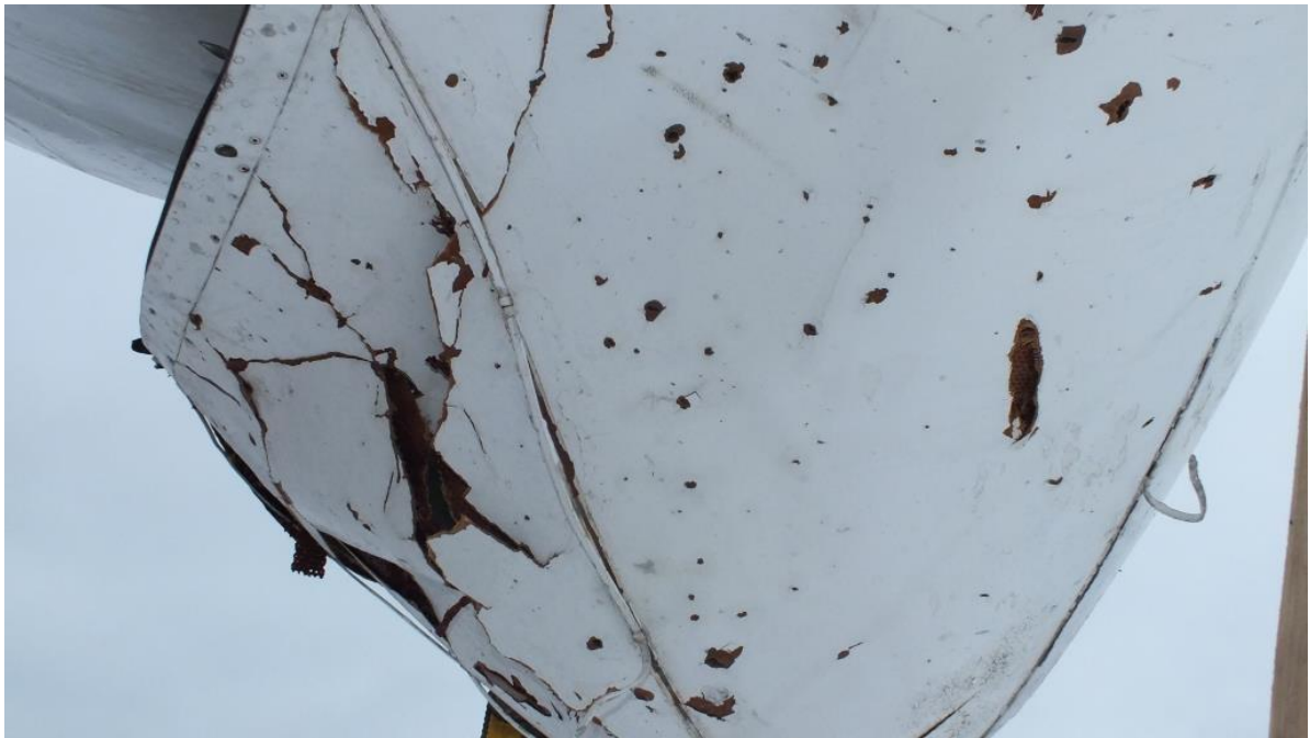
Figure 5.11 - Entry holes in the radiotransparent radome
