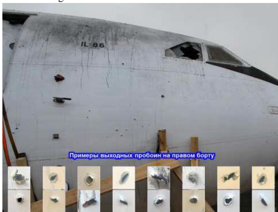
Figure 5.2.30 - Examples of through-hole exit punctures ("inside-out") on the starboard side of the IL-86 target aircraft
