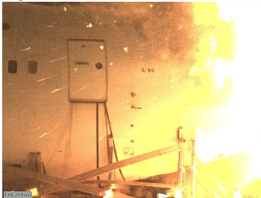
Figure 4.17 - Detonation of the 9H314M warhead
