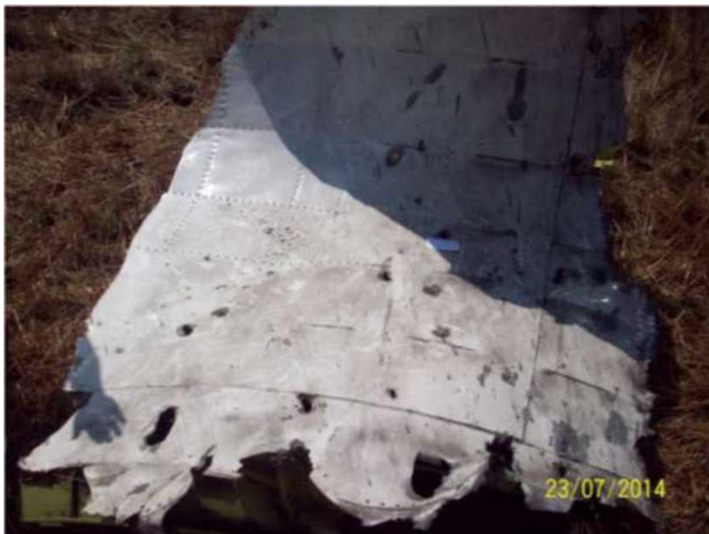
Figure 5.1.2 - Fragment of the cockpit roof. In the Preliminary Report materials it was one of the main pieces of evidence for the impact of high-energy objects (DSB submissions)
