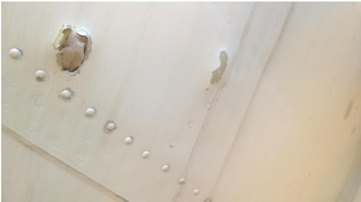
Figure 5.88 - Exit hole (left) and non-penetrating damage (right) close-up
