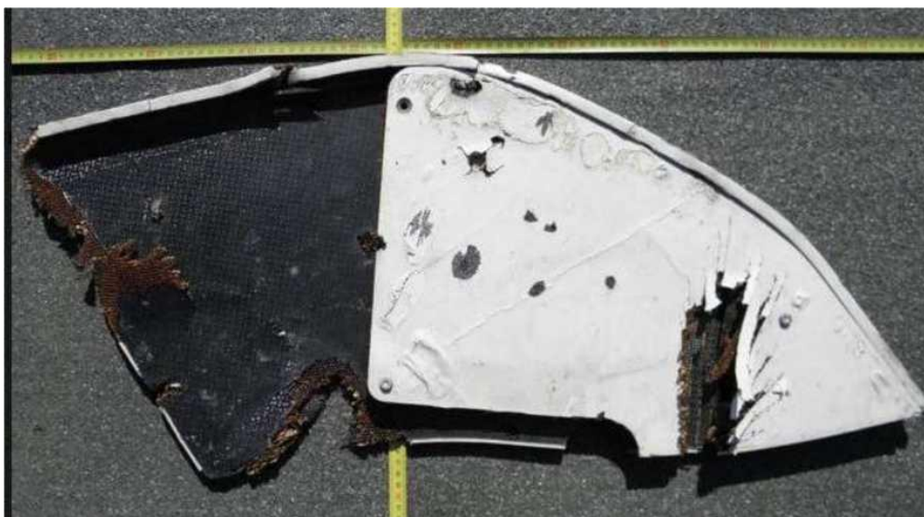
Figure A.3.12 - Fragment of passenger compartment luggage rack with (suspected) fragmentation damage
