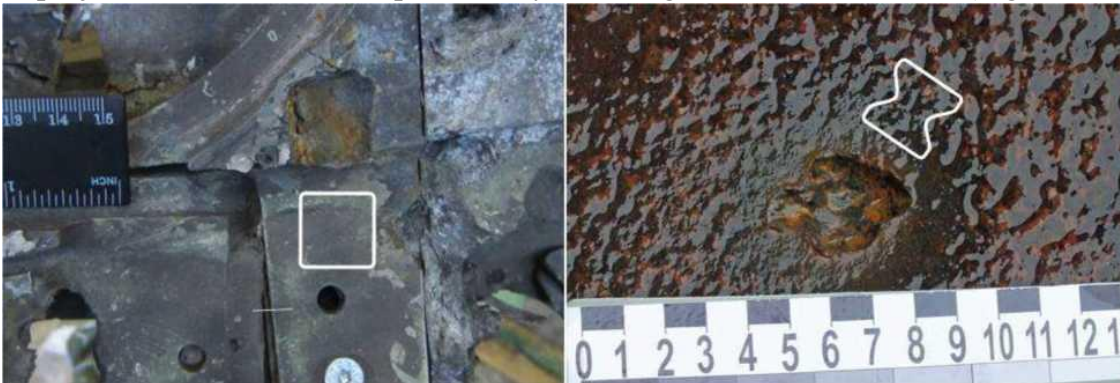
Figure A. 2.6 - Characteristic non-penetrating damage: left - MH17; right - target acquisition (experiment)
