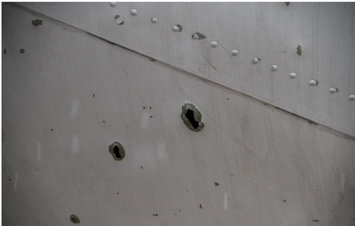
Figure 5.85 - Exit holes and non-penetrating damage
