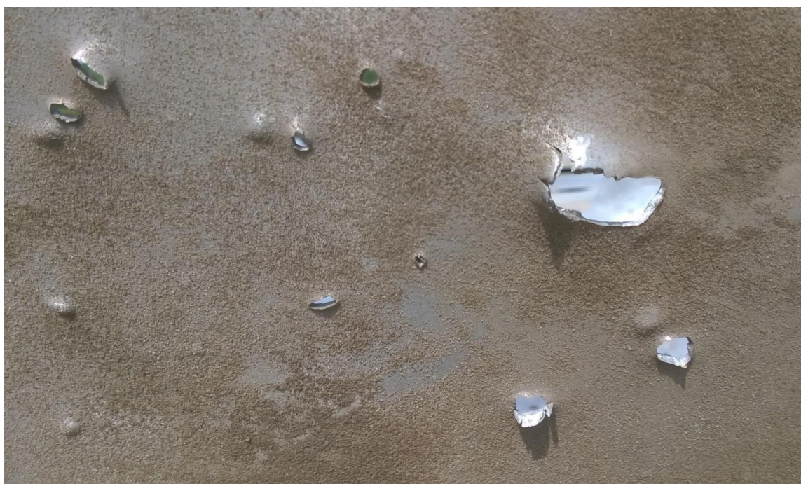
Figure A.199 - Exit holes with jagged edges and non-penetrating damage on target No. 4 (view from the back of the shield)
