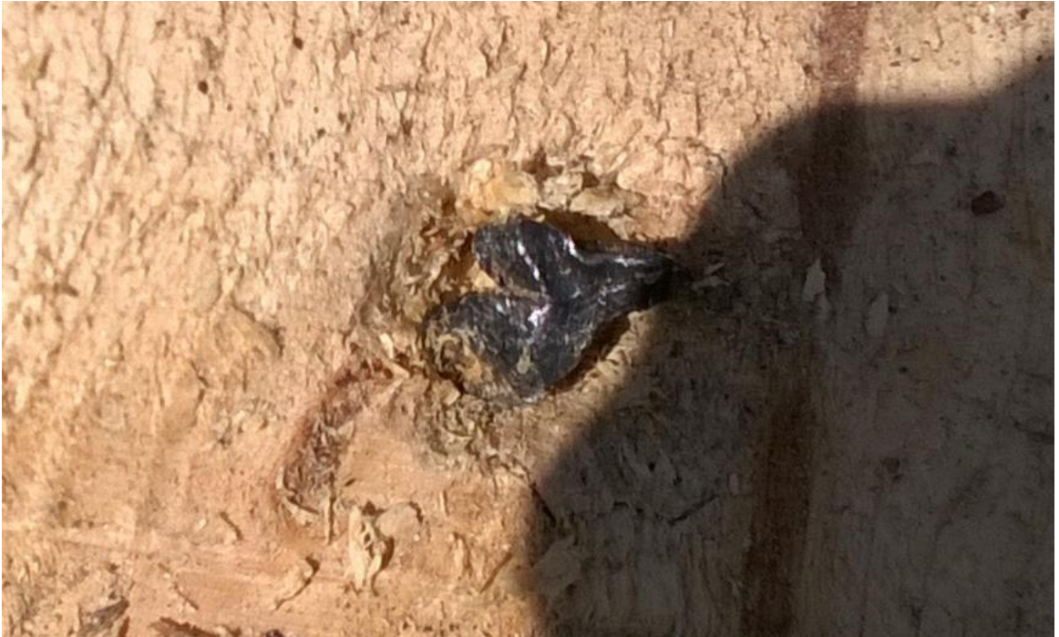
Figure A.203 - 9H314M 1-10 projectile ("bowtie ") which was deformed but retained its original shape
