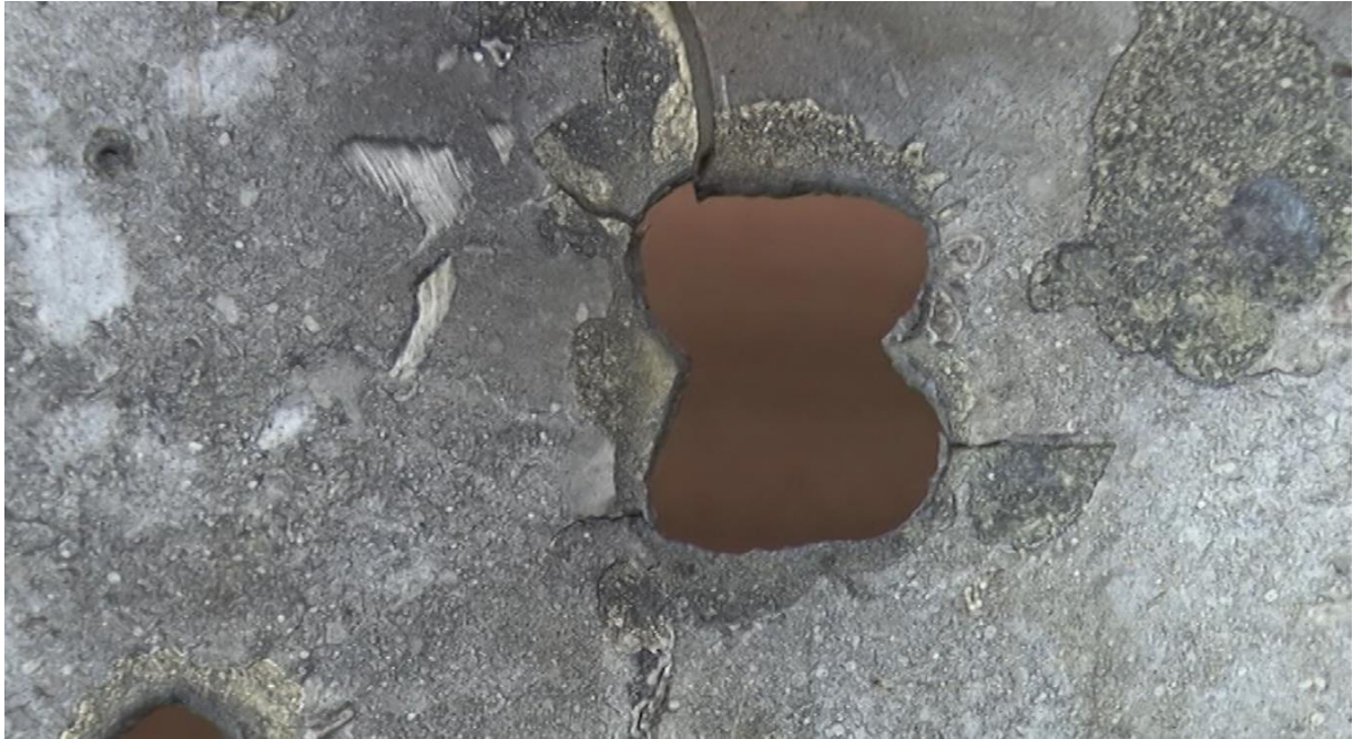
Figure 6.20 - Characteristic butterfly-shaped penetration
