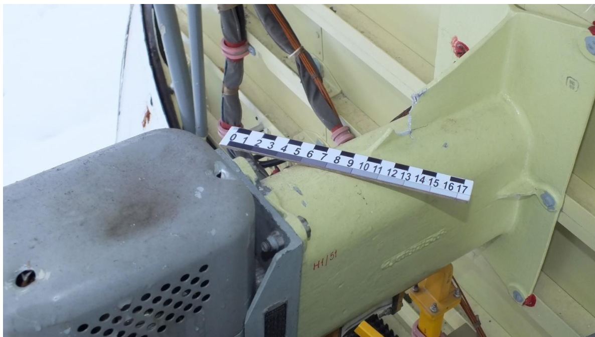
Figure 5.15 - Through-and-through holes in weather radar equipment
