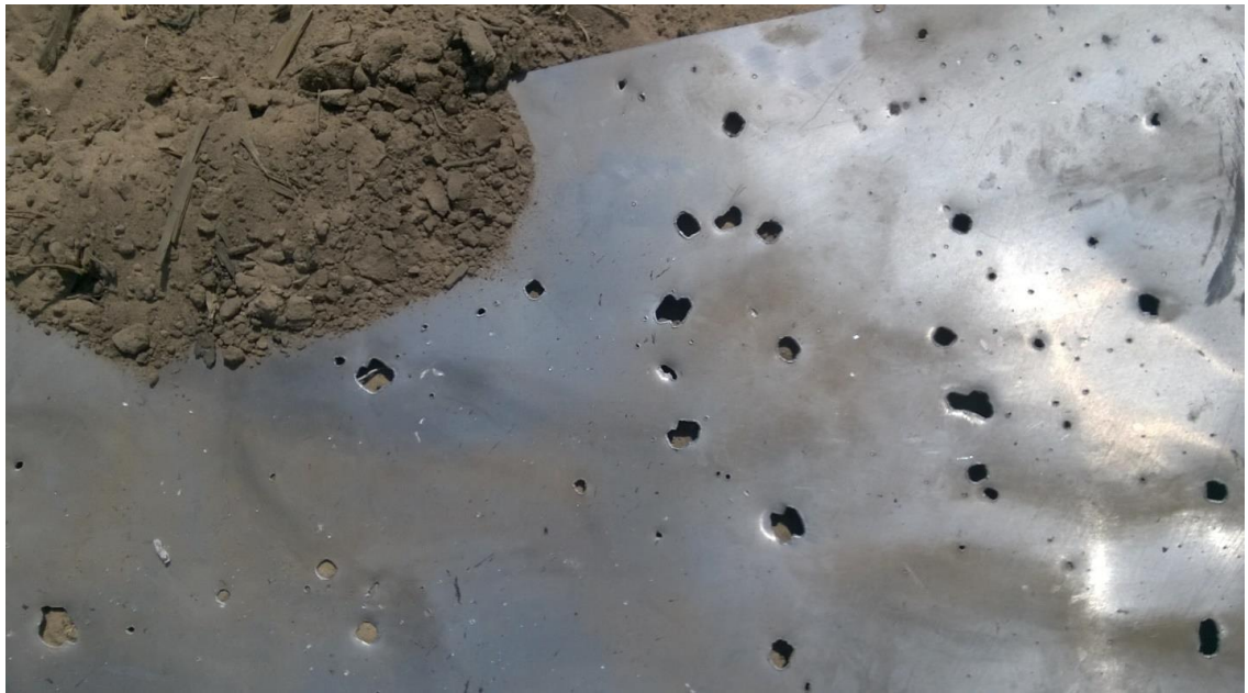
Figure A.171 - Characteristic "butterfly"-shaped holes
