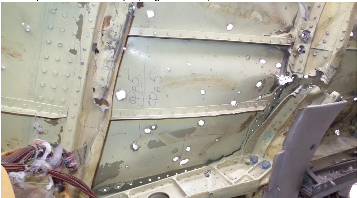
Figure 5.168 - Fragment No. 5 before extraction (internal view)
