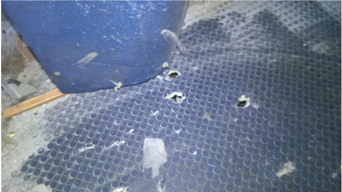
Figure 5.122 - Through-and-through holes in the cockpit floor (starboard)
