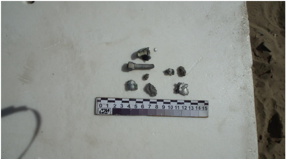
Figure A.51 - Hull fragments (those of the compartment hull) recovered from traps
