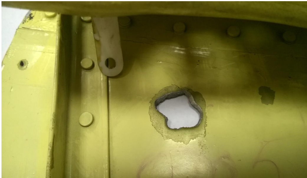
Figure 5.174 - Characteristic butterfly-shaped hole in the outer skin of the port caused by a bowtie shaped preformed fragment of 9H314M 1-10 (inside view)
