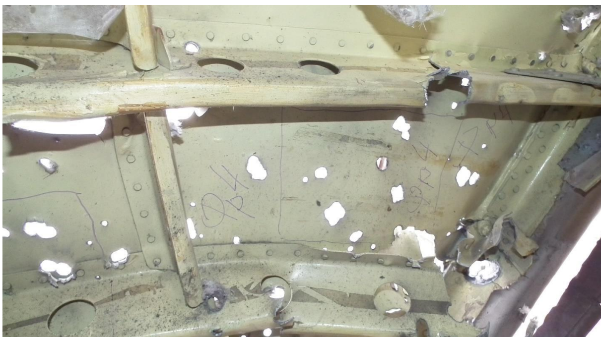
Figure 5.146 - Through-and-through holes in the roof and cockpit stringer (right side)
