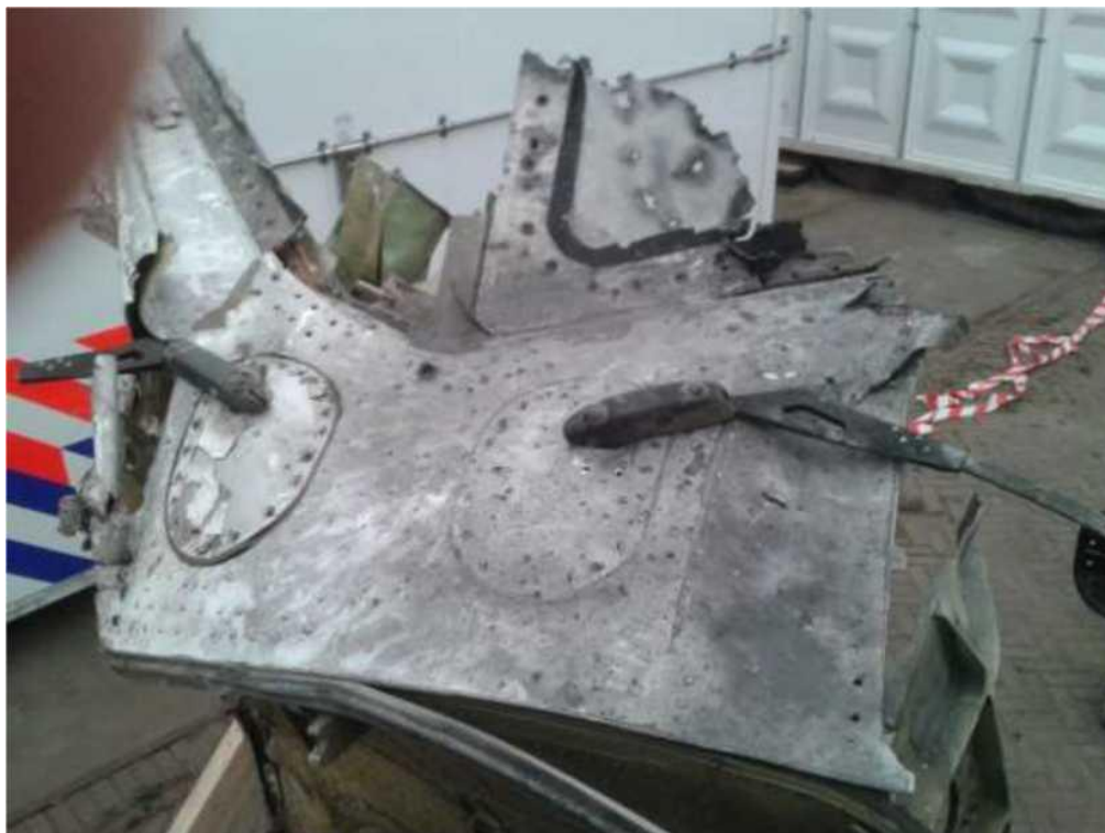
Figure 5.1.7 - Fragment of the nose of Boeing 777 adjacent to the forward pressure bulkhead, from above (photo of February, 2015)
