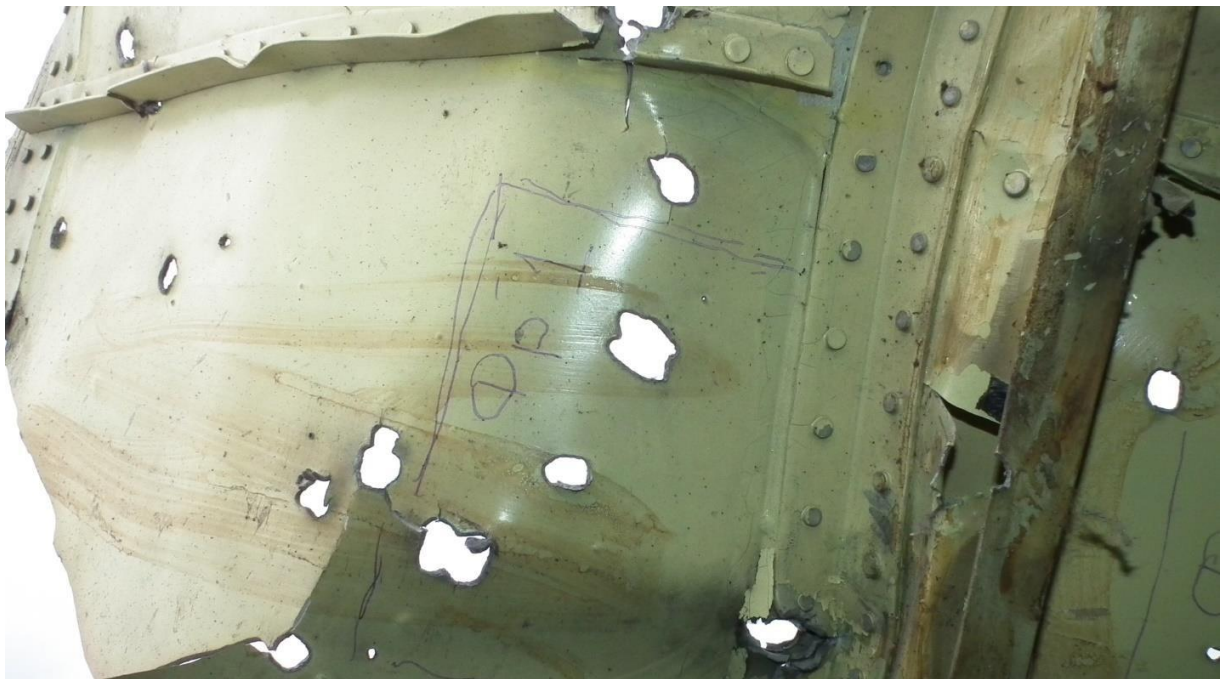
Figure 5.156 - Fragment No. 1 (close-up, inside view). Characteristic holes caused by preformed fragments of 9H314M 1-10 are seen on the inner surface of the skin.
