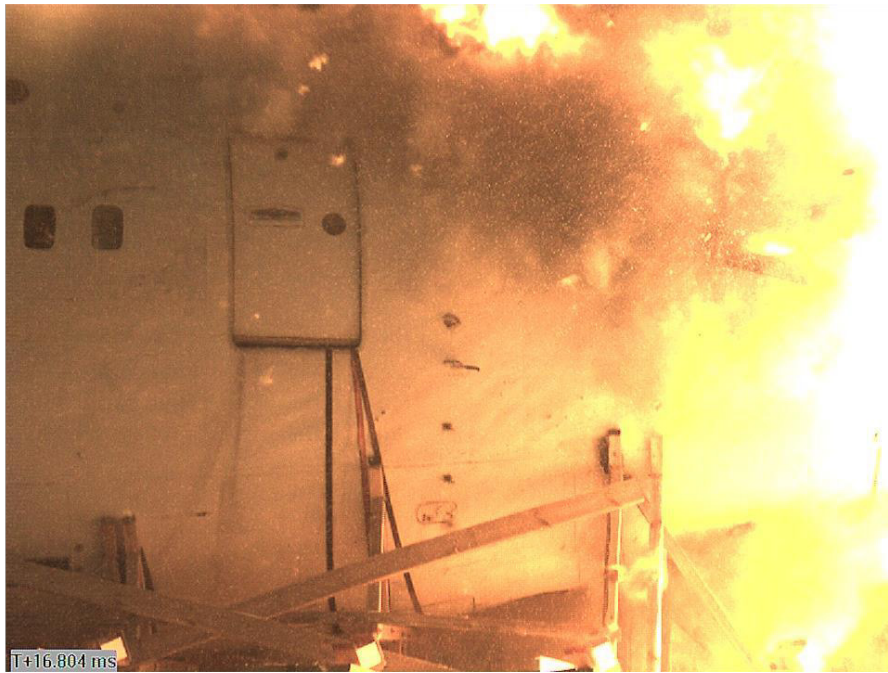
Figure 4.31 - Detonation of the 9H314M warhead
