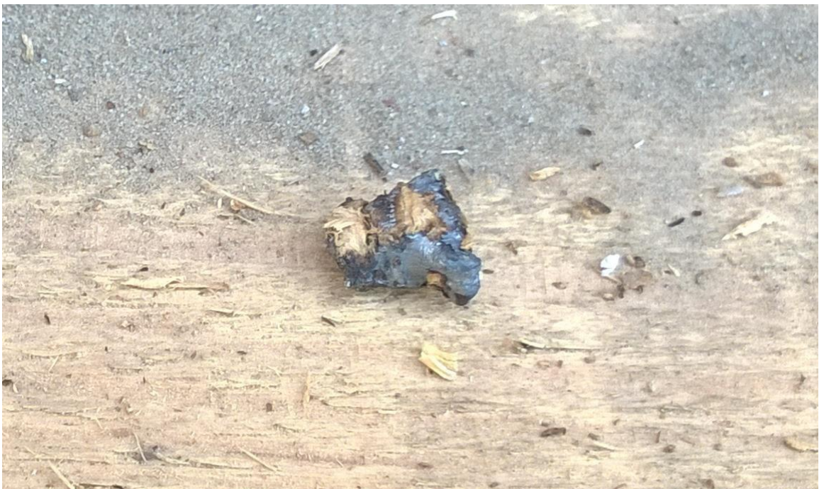
Figure A.204 - 9H314M 1-10 projectile ("bowtie") which lost its original shape
