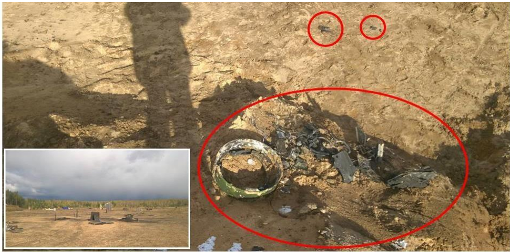
Figure 9.7 - First compartment fragments impact point (the place where first compartment fragments fell is shown in the bottom left corner)
