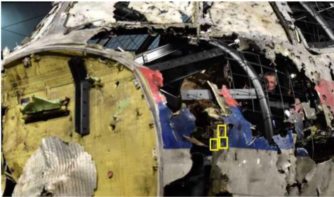
Figure A.3.1 - Through-and-through-and-through damage to the forward fuselage bulkheads
