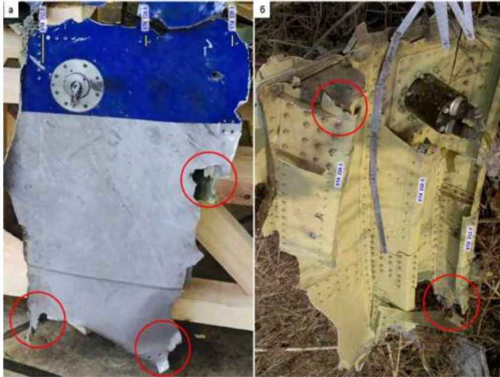
Figure 5.1.69 - Blast damage on a fragment with an angle of attack sensor on the outer (a) and inner (b) sides
