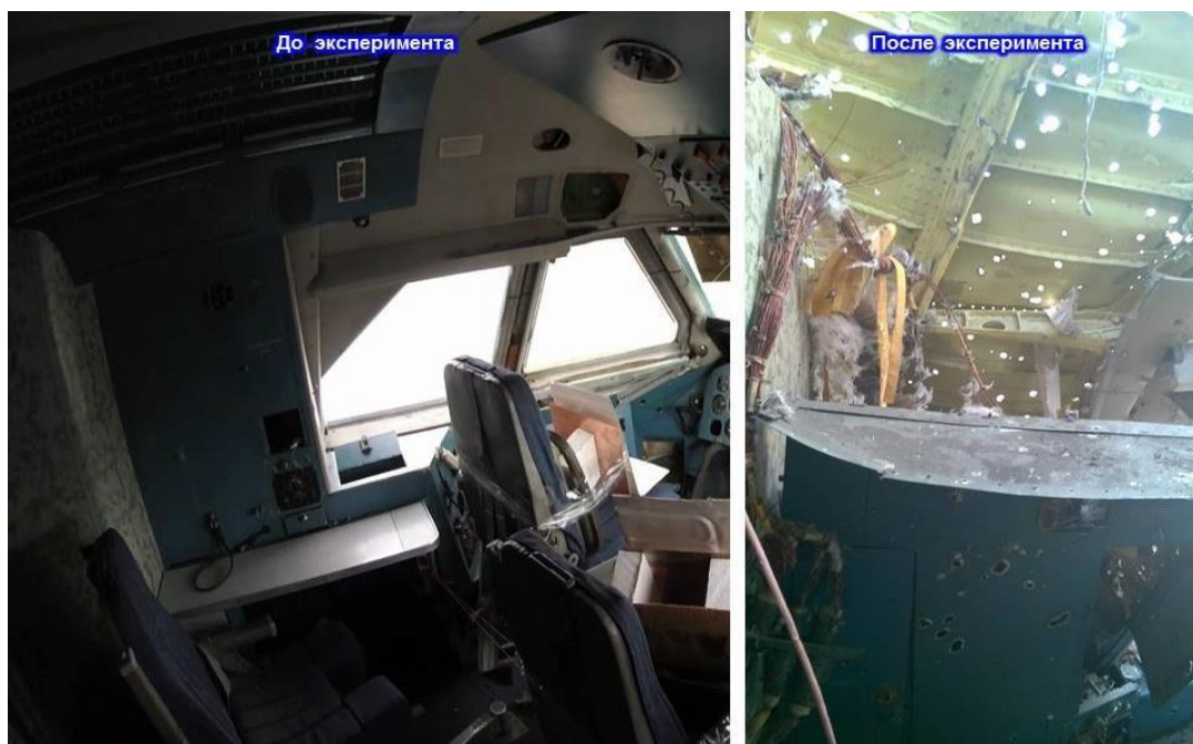
Figure 5.107 - Appearance of the cockpit's interior on the port side of the target aircraft: before the tests (left) and after detonation of the 9H314M warhead (right)
