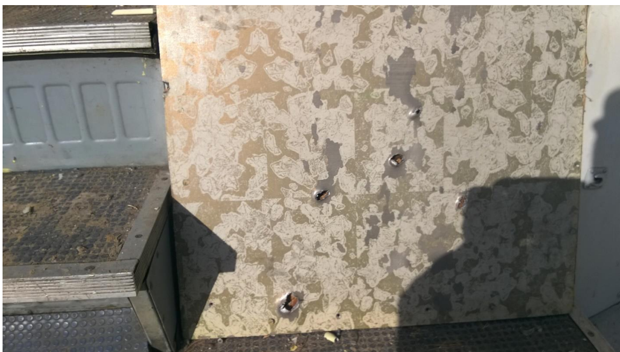
Figure 5.138 – Exit holes in the lower right section of the first passenger compartment (rear view)
