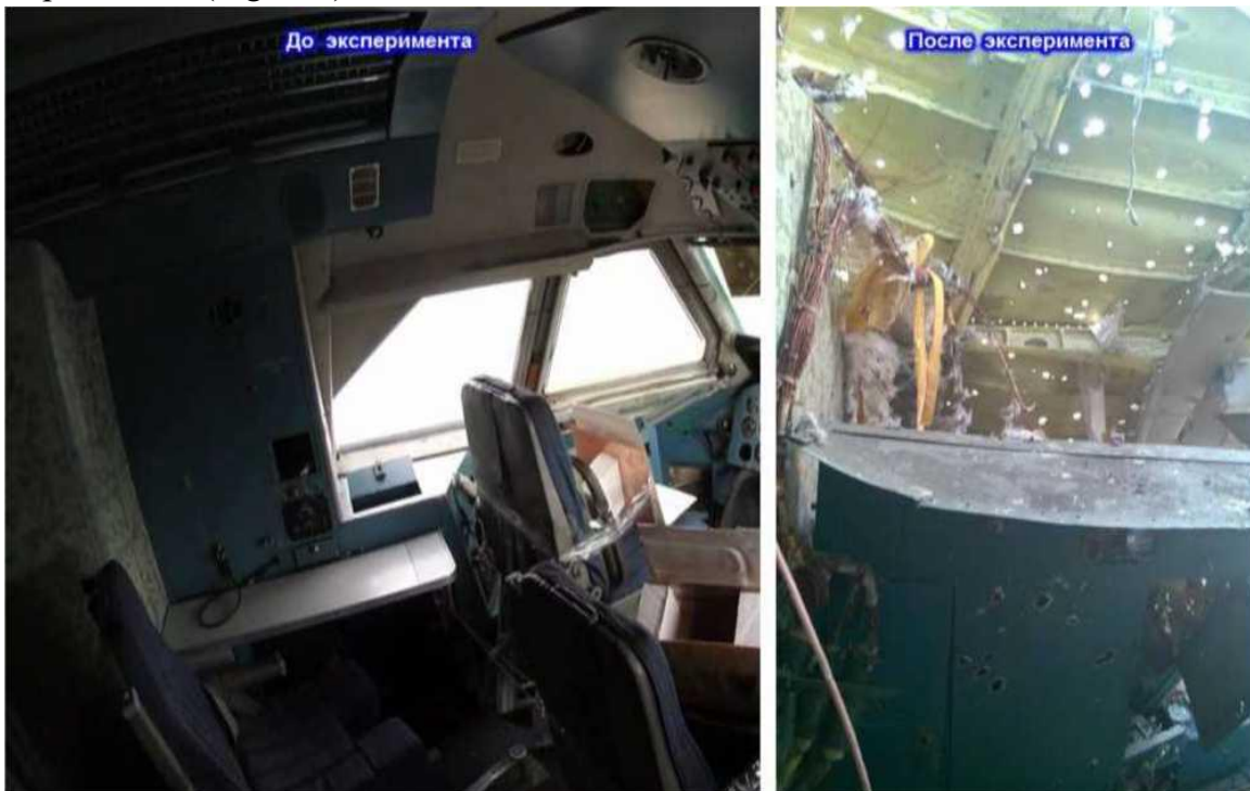
Figure C.4 - Metal cabinet and steel safe on the port side, located behind the crew commander's seat: left - before the experiment; right - after the experiment
