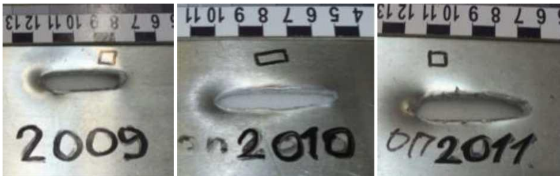
Figure B.4.8 - Exterior view of barriers after interaction with the projectiles
