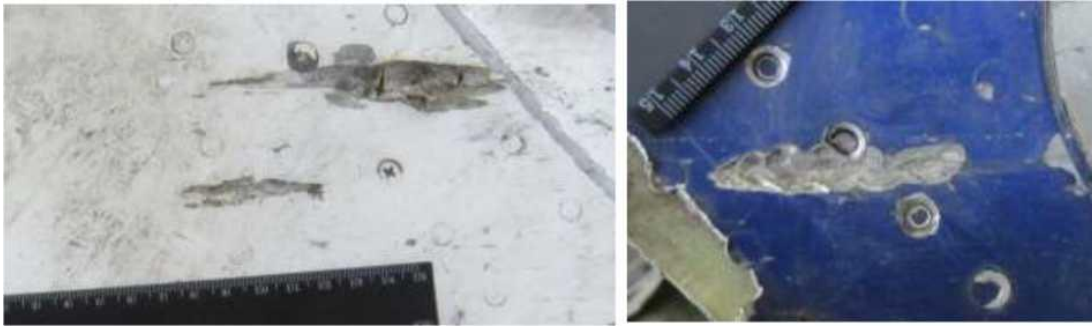
Figure A.1.15 - Examples of boundary damage in fragment "F.1" (left) and fragment "F.9" (right)
