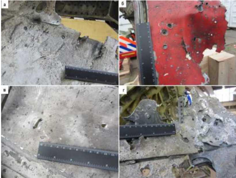
Figure 5.1.64 - Microcrater areas: right side of cockpit roof (a), forward part with pressure bulkhead (b, c), transparency frame (d)
