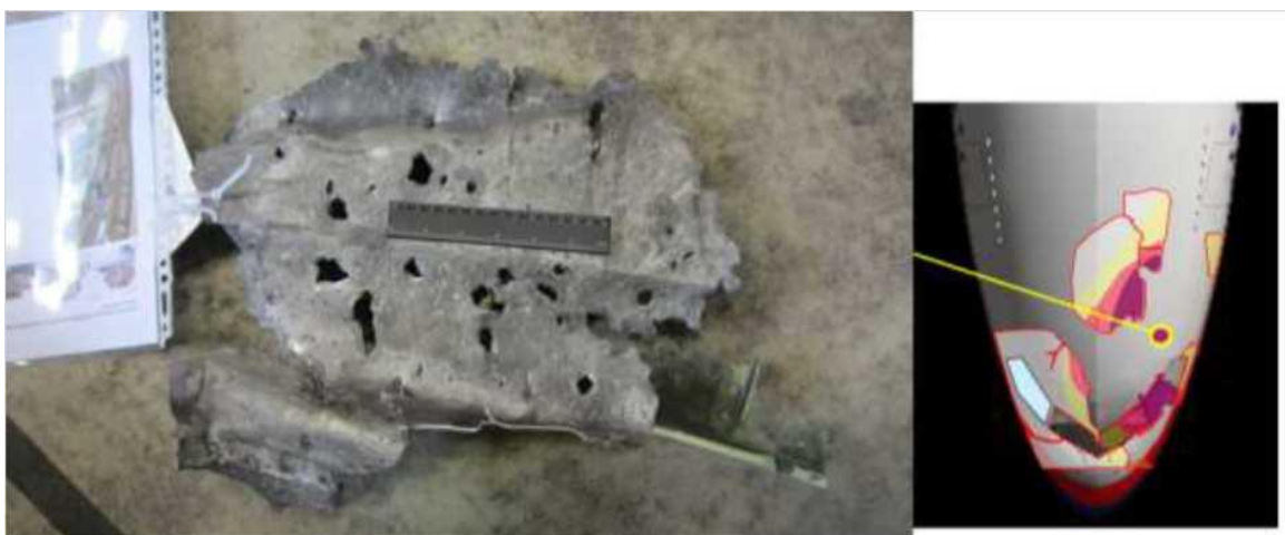
Figure 5.1.33 - Fragment of the port side behind the cockpit windows
