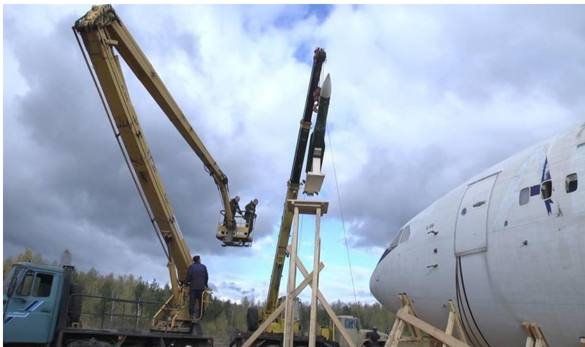
Figure 3.7 - Mounting the item 9M38M1 on the test bench
