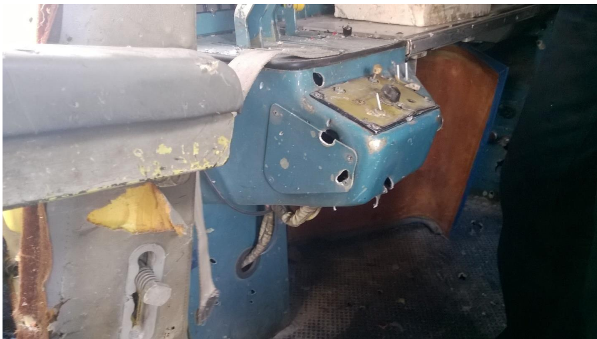
Figure 5.115 - Damage to the flight engineer's control panel (starboard side of the cockpit)
