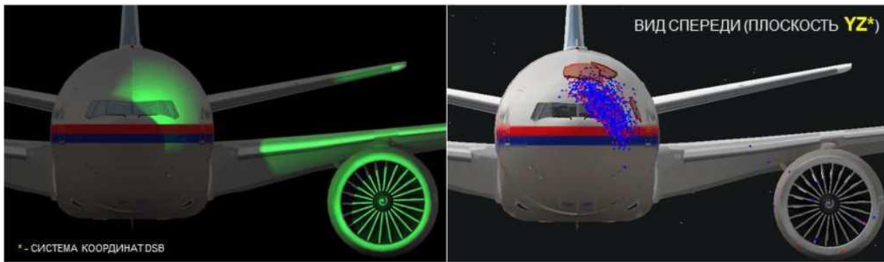
Figure 5.2.19 - Damage model visualisation for the "collision course" version, which explains all damage to the outer skin, airframe, left wing plane and left engine of the Boeing 777: left - damage boundary model; right - fragmentation coverage field
