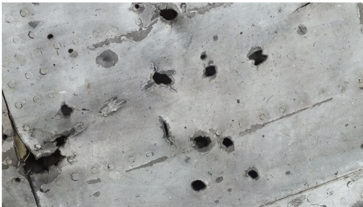
Figure 5.45 - Port side skin with characteristic butterfly-shaped holes caused by 9H314M 1-10 projectiles (close-up)
