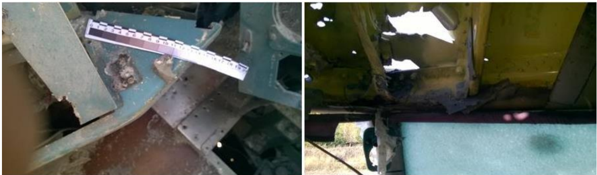
Figure 9.4 - Second compartment hull fragments and holes left by them
