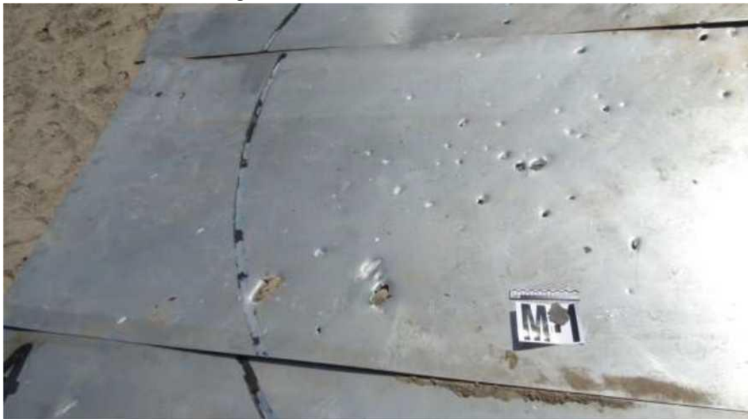
Figure 5.2.29 - At small angles between the velocity vector and the plane of the obstacle, hull fragments do not penetrate beyond the obstacle and ricochet occurs
