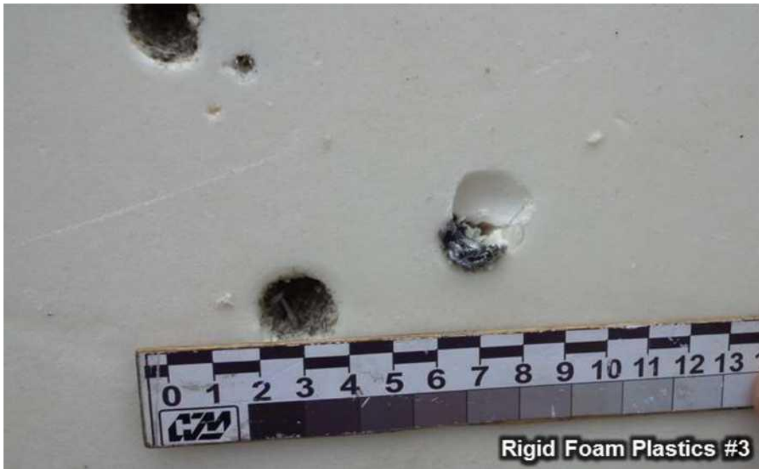
Figure 5.2.27 - Hull impactor (compartment hull fragment) lodged in the third layer of stopping foam PS-1-150 of trap "L.1" of the shielded target layout (31.07.2015)
