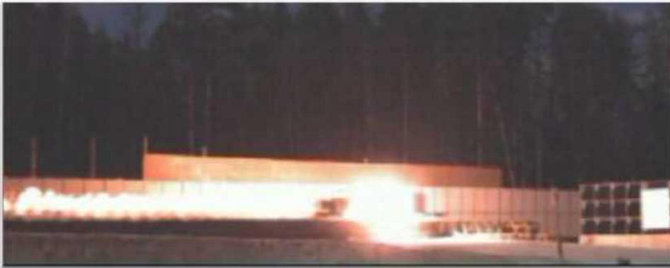
Figure D.13 - Ground tests in a shield target layout under dynamic conditions at the rocket booth. Velocity of the experimental setup at the moment of detonation - 1,010 m/s
