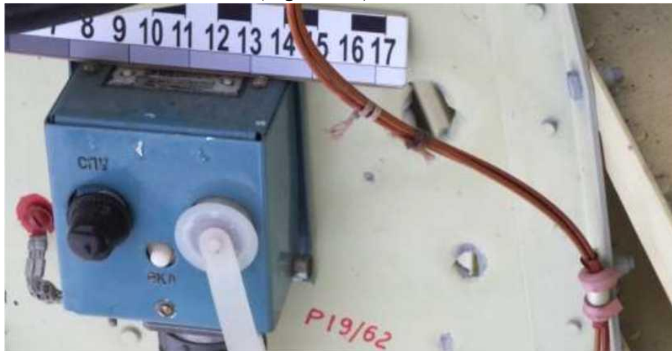
Figure F.8 - Example of through-holes in the weather radar equipment of target aircraft IL-86 (Proceedings of the Experimental Report)
