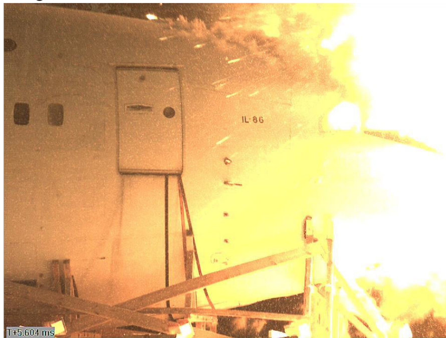
Figure 4.9 - Detonation of the 9H314M warhead
