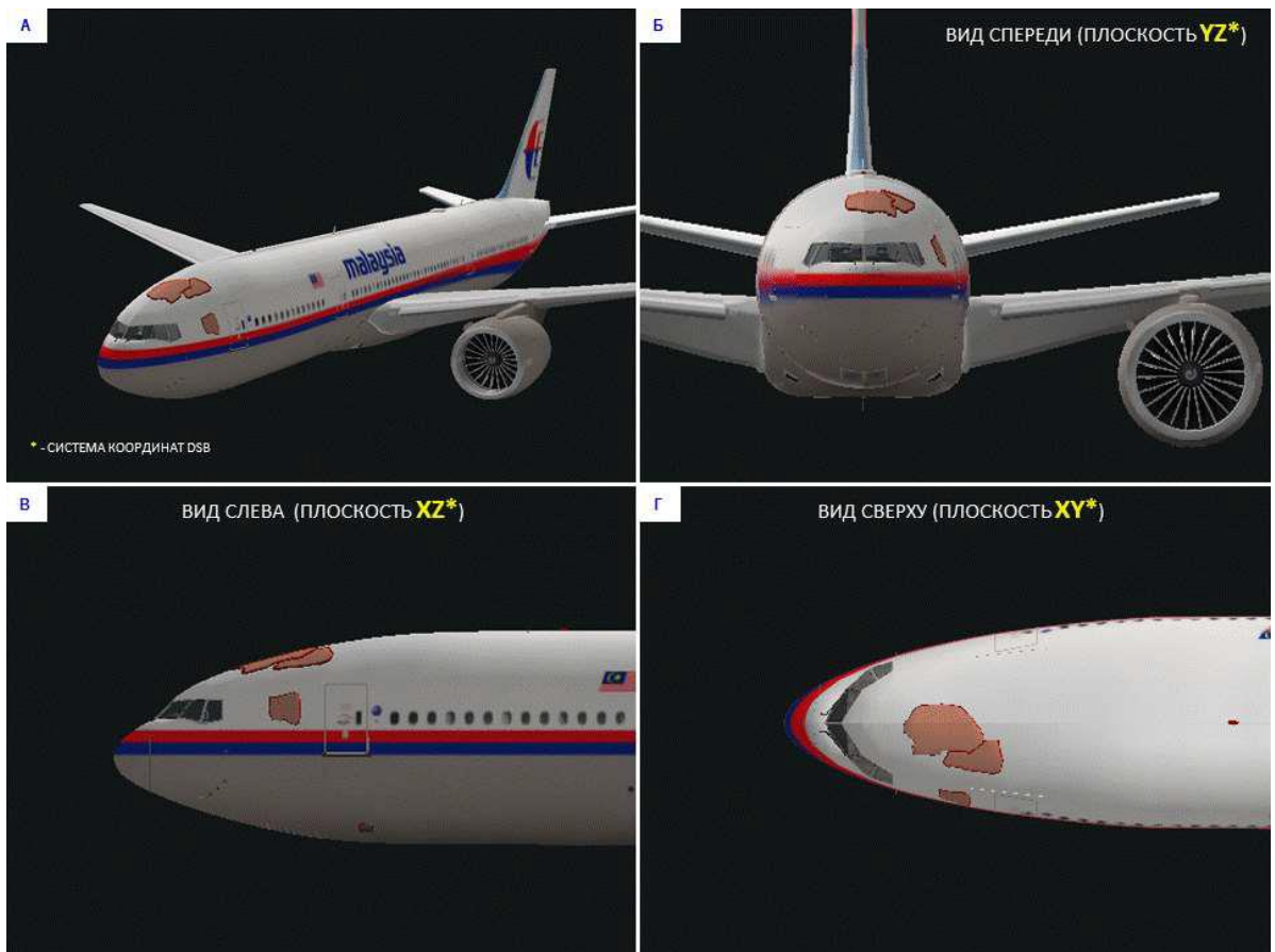
Figure A.1.14 – Distribution of fragments in the structure of MH17
