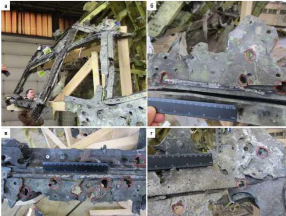
Figure A.1.2 - Exterior view of fragment "F.2" (a) and areas of the fragment with characteristic damage (b, c, d) highlighted in red
