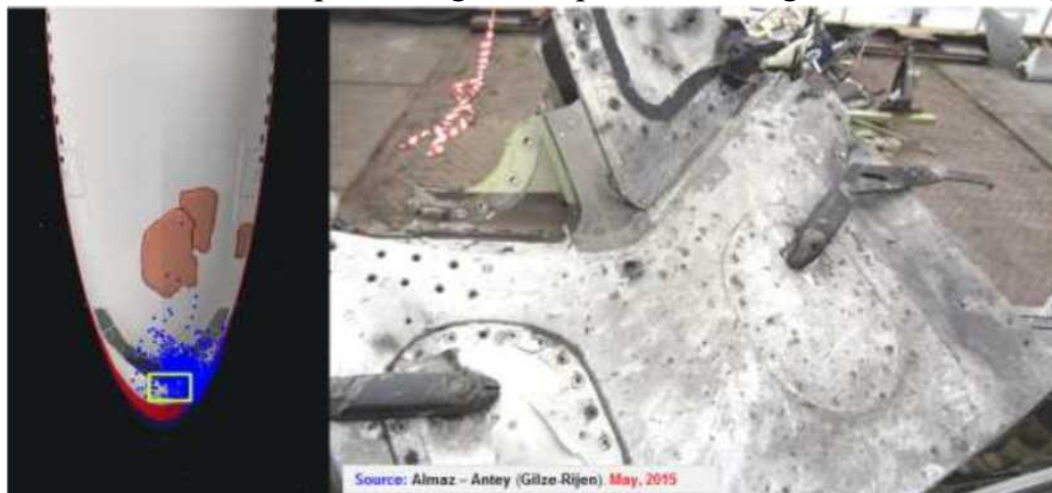
Figure F.9 - Inconsistency of damage in front of cockpit windshields: according to modelling results, the fragment should show multiple GPE damage (left); the fragment in front of windshields does not have a high density of damage (right)
