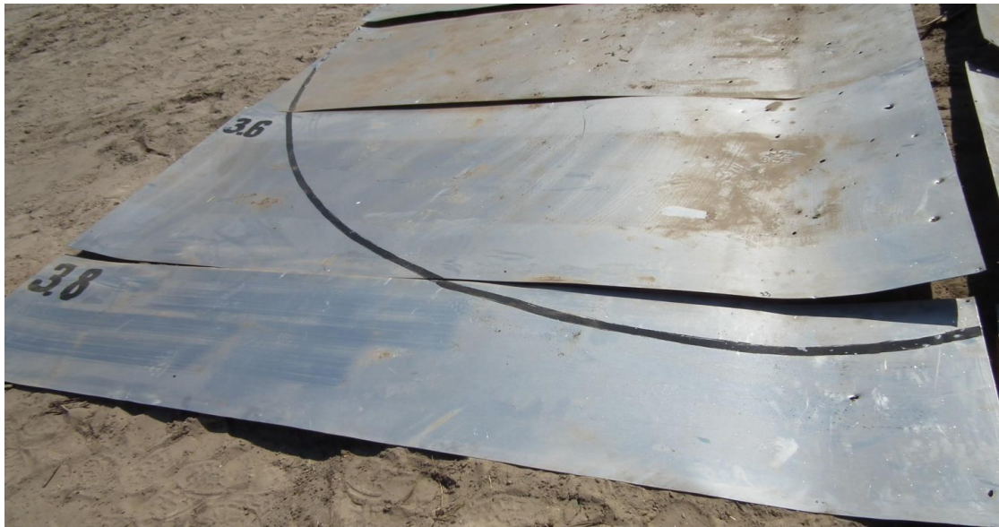
Figure A.103 - Fragments 3.4 (top), 3.6 and 3.8 (bottom) of target No. 3
