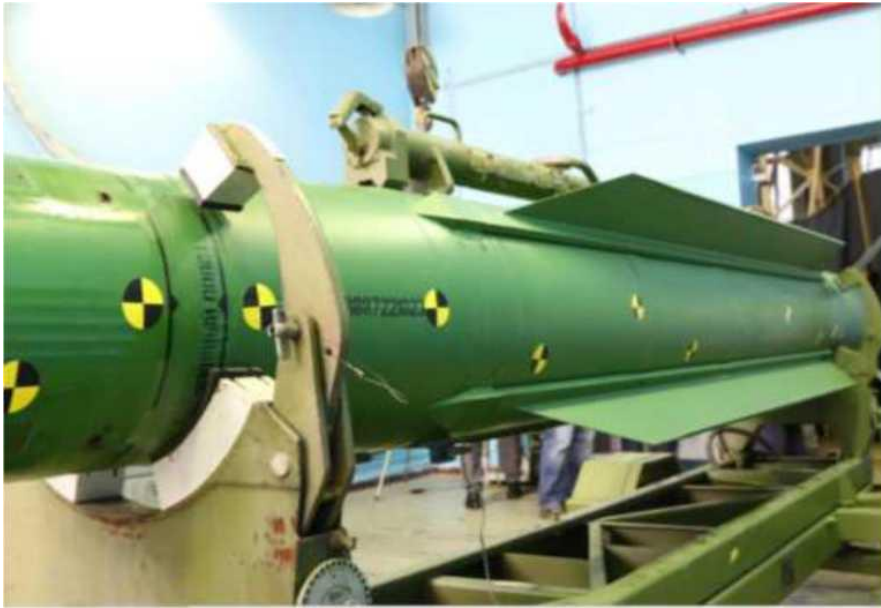
Figure E.4 - 9M38M1 missile delivered by Ukraine to the investigation (SBN materials). After installation of the wings, the process stamp "Assembling Date" is not visible - it is covered by the relevant wing
