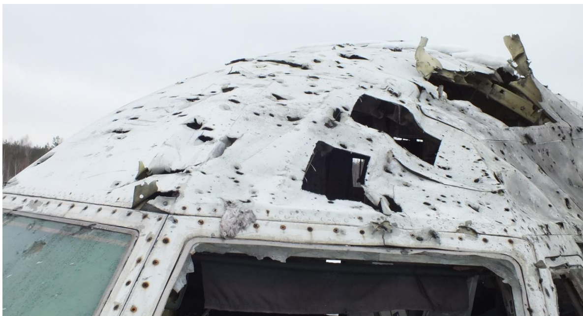
Figure 5.54 - Cockpit roof after removal of fragments (front view)
