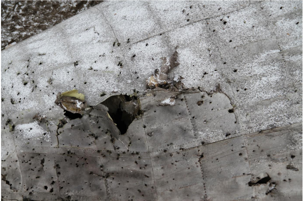
Figure 5.64 - Cockpit roof with aero-strike marks (overall view)
