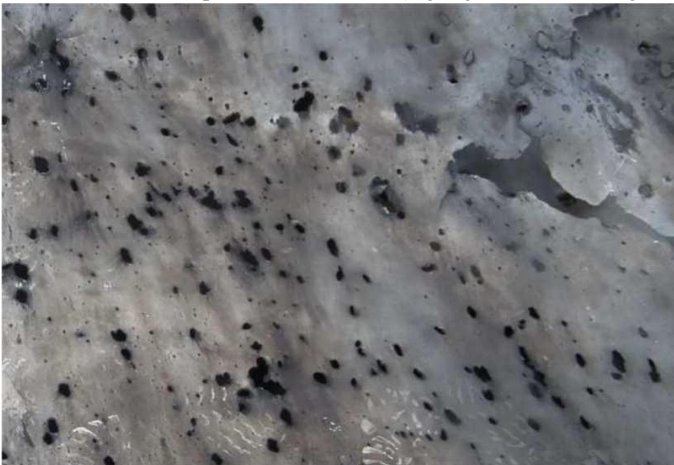
Figure A.4.22 - Fragment of target 1.1 (full-scale experiment in a shield target layout conducted on 31.07.2015)
