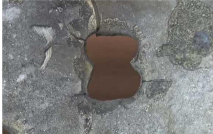
Figure G.4.9 - Characteristic hole in the outer skin of the IL-86 target aircraft (experiment 07.10.2015)
