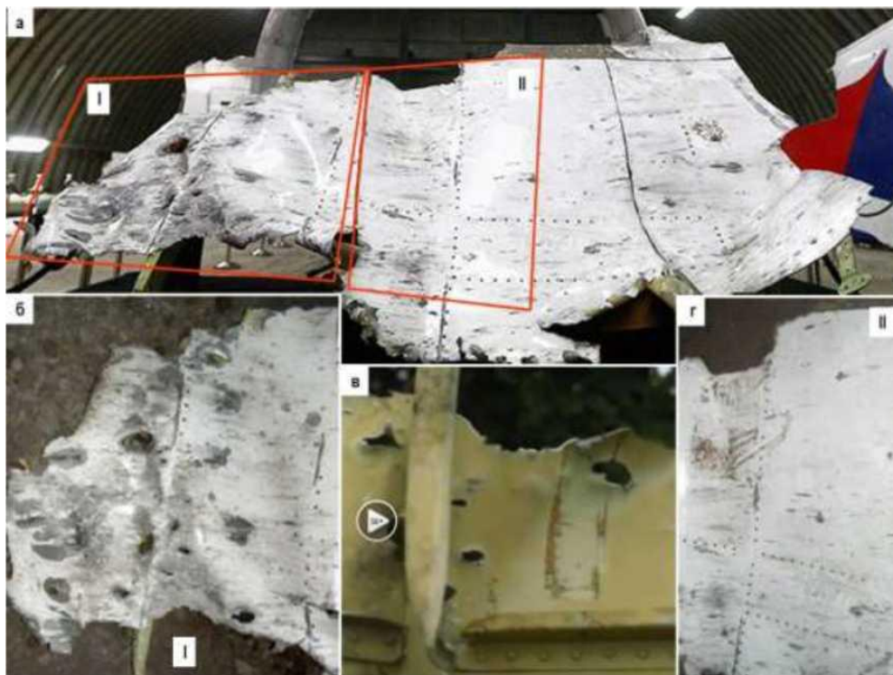
Figure A.1.7 - Exterior view of fragment "F.7" (a) and areas of fragment with characteristic damage from outside (b, d) and inside (c) the port side and roof behind the cockpit
