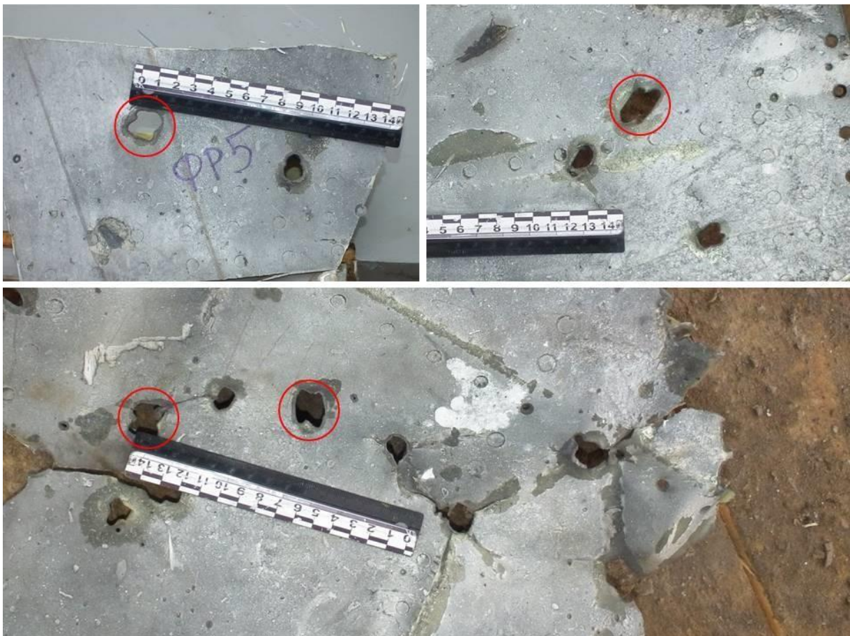
Figure 6.11 - Fragments of the port side and the cockpit roof
