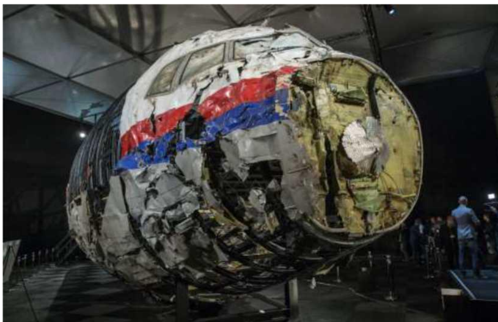
Figure 5.1.49 - Fragment of the right-hand side of the cockpit with part of the roof and retained transparency on the right-hand pilot's side
