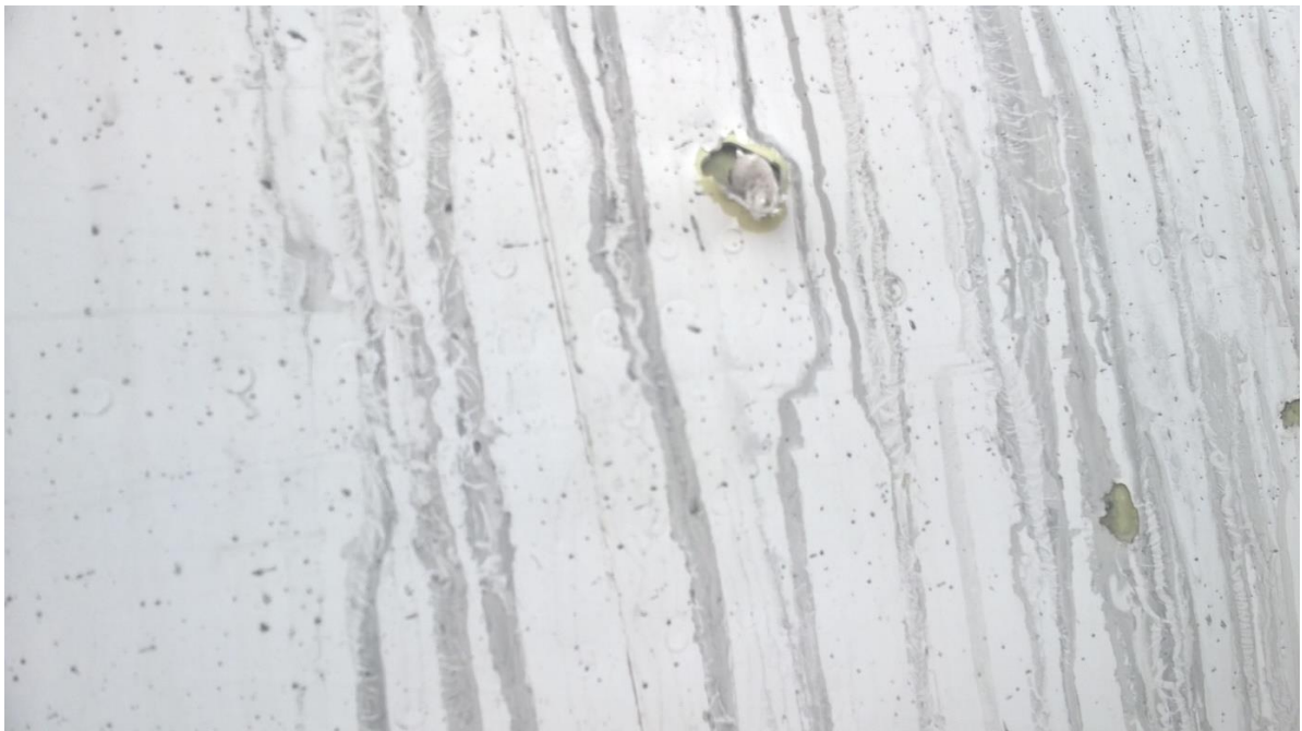
Figure 5.94 - Exit holes and non-penetrating damage
