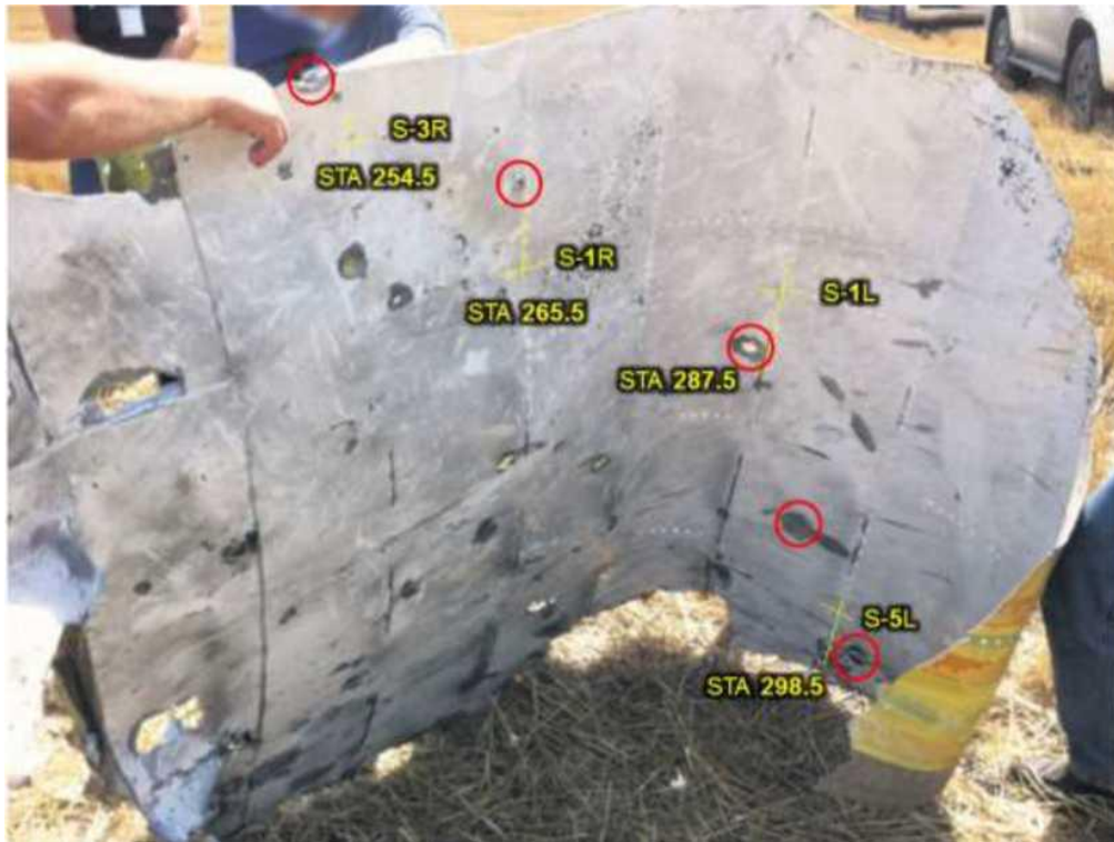
Figure 5.1.20 - A fragment of the cockpit roof objectively shows the boundary of the fragmentation field (photo - DSB resource)
