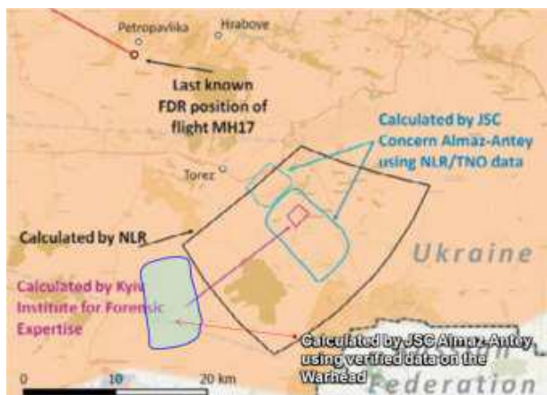
Figure G.3.3 - Launch area calculated using missile-aircraft encounter methodology, taking into account actual aircraft longitudinal axis orientation and verified warhead data
