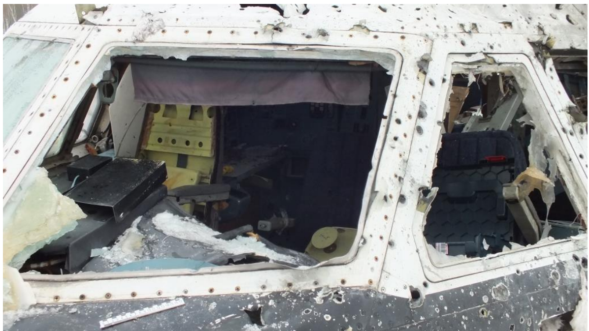
Figure 5.24 - Aircraft commander's windscreen and direct-vision window (left front view)
