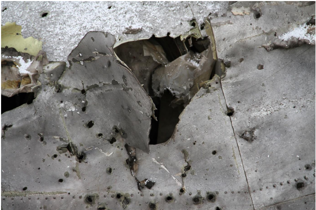
Figure 5.63 - Fragment of cockpit roof (close-up).
