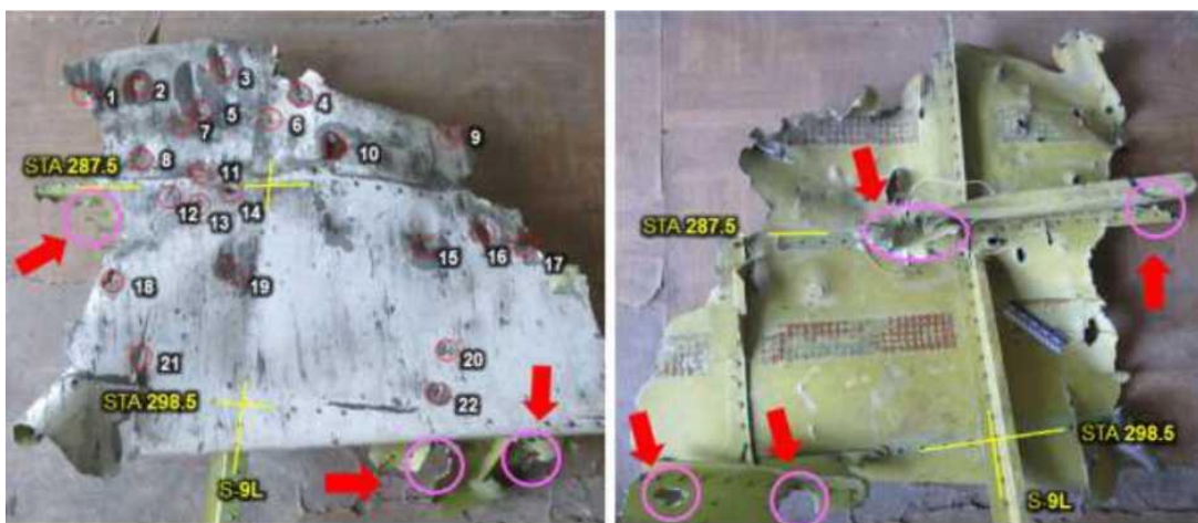
Figure A.3.5 - Fragment of the upper port side behind the cockpit: external (left) and internal (right) views. Multiple holes in the STA 287.5 and STA 298.5 bulkheads resulted in deformation and failure of the structural elements (red arrows indicate characteristic damage)
