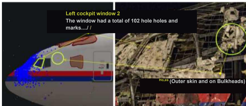
Figure F.12 - Inconsistency of damage in the area of the second and third windows on the left side of the cockpit
