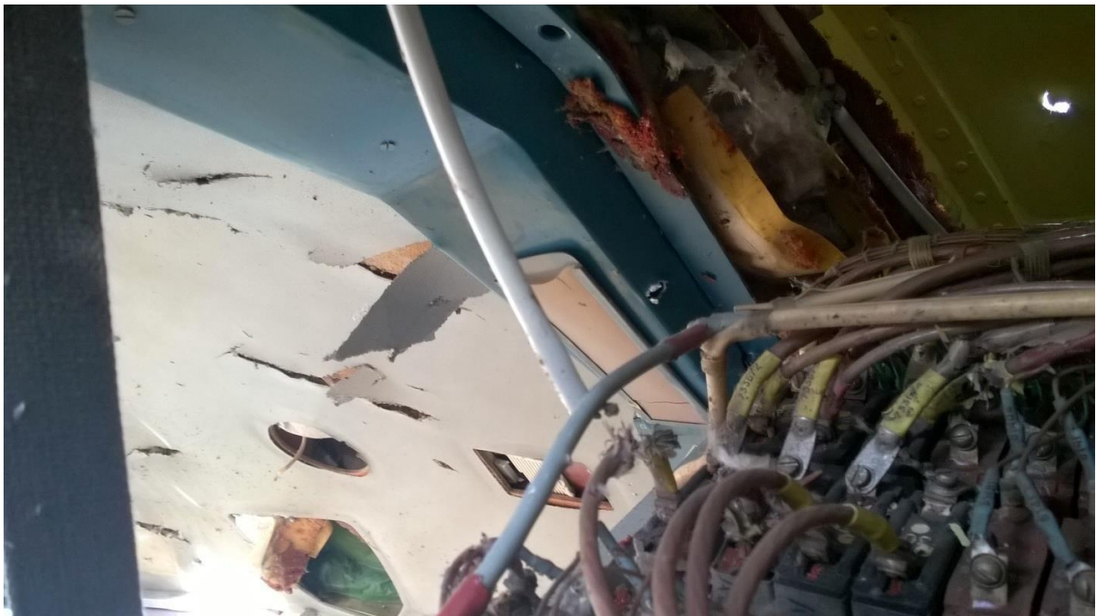
Figure 5.137 - Material-intensive components of the avionics equipment. Instrumentation panel in the top section of the starboard (in the top right corner, there is an exit hole in the right section of the cockpit roof)
