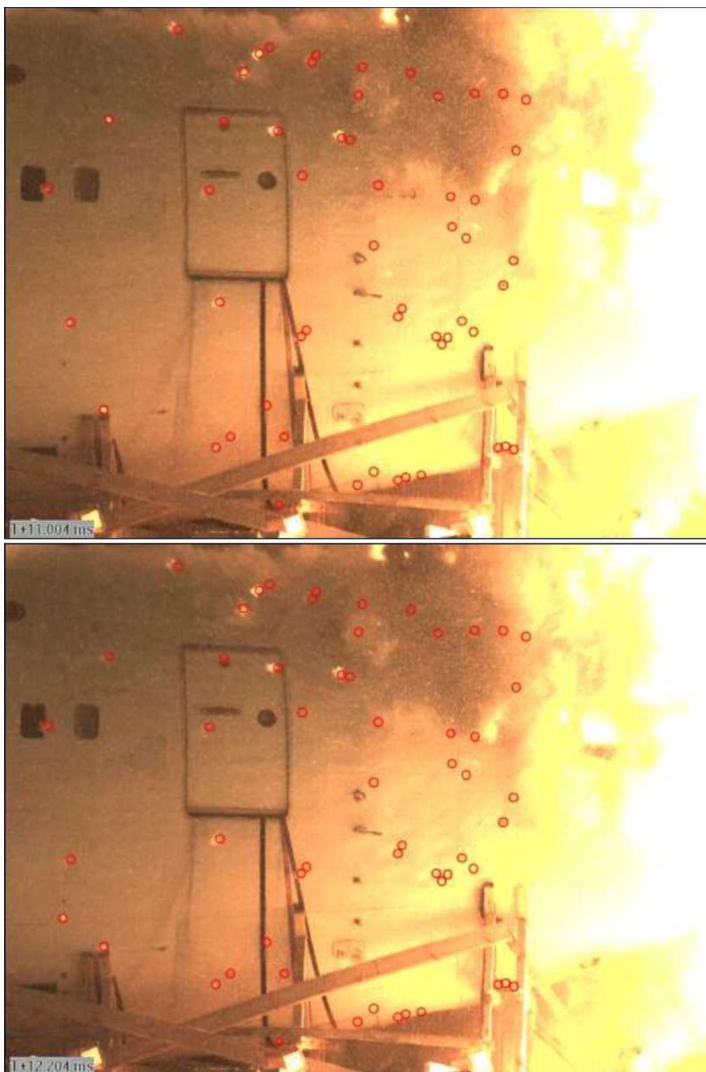
Figure B.3.16 - Puncturing the starboard side of target aircraft IL-86 (top - T+ 11.004 ms; bottom - T+ 12.204 ms)
