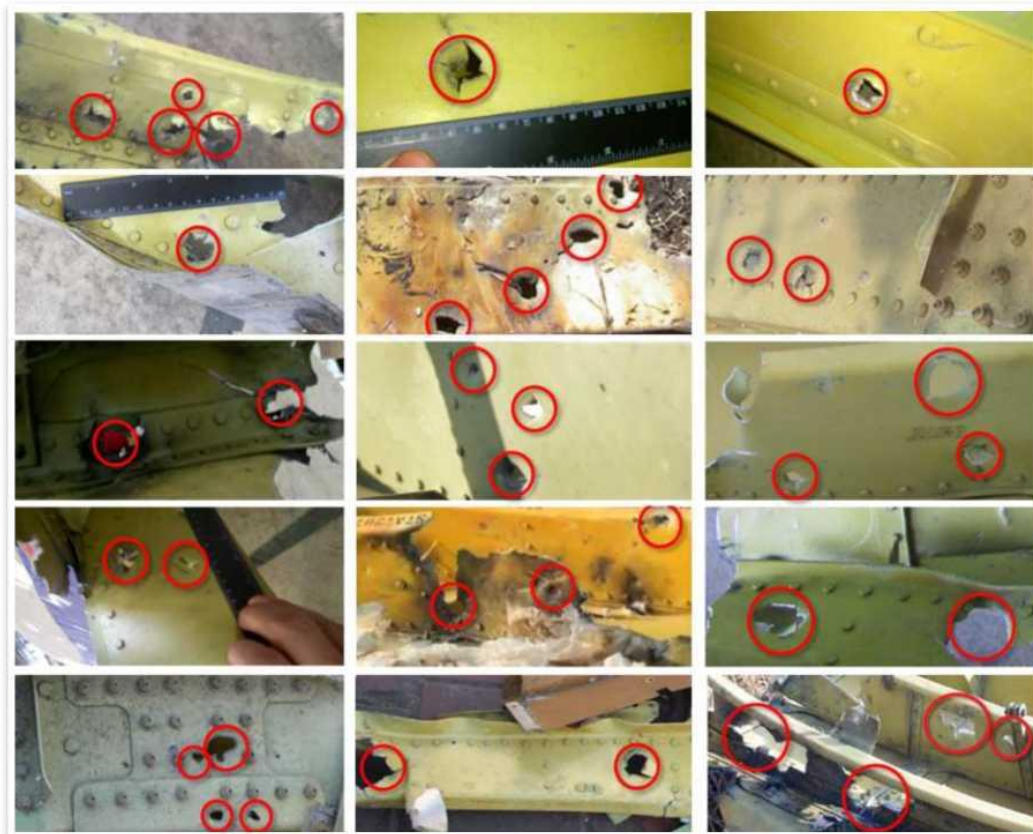
Figure A.3.11 - Examples of damage to bulkheads
