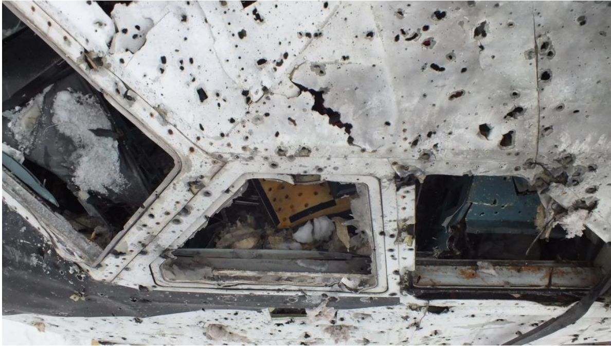
Figure 5.35 - Top of port side (overall view above the aircraft commander's windows). The fragment shows deformation and tearing of the outer skin
