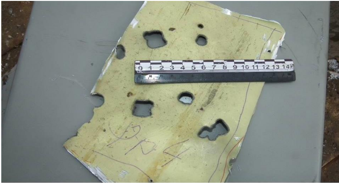
Figure 6.8 - Fragment of the left-hand side of the cockpit roof (inside view)
