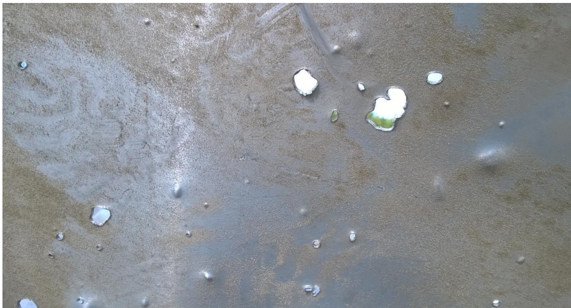
Figure A.196 - Exit holes and non-penetrating damage (view from the back of the shield)
