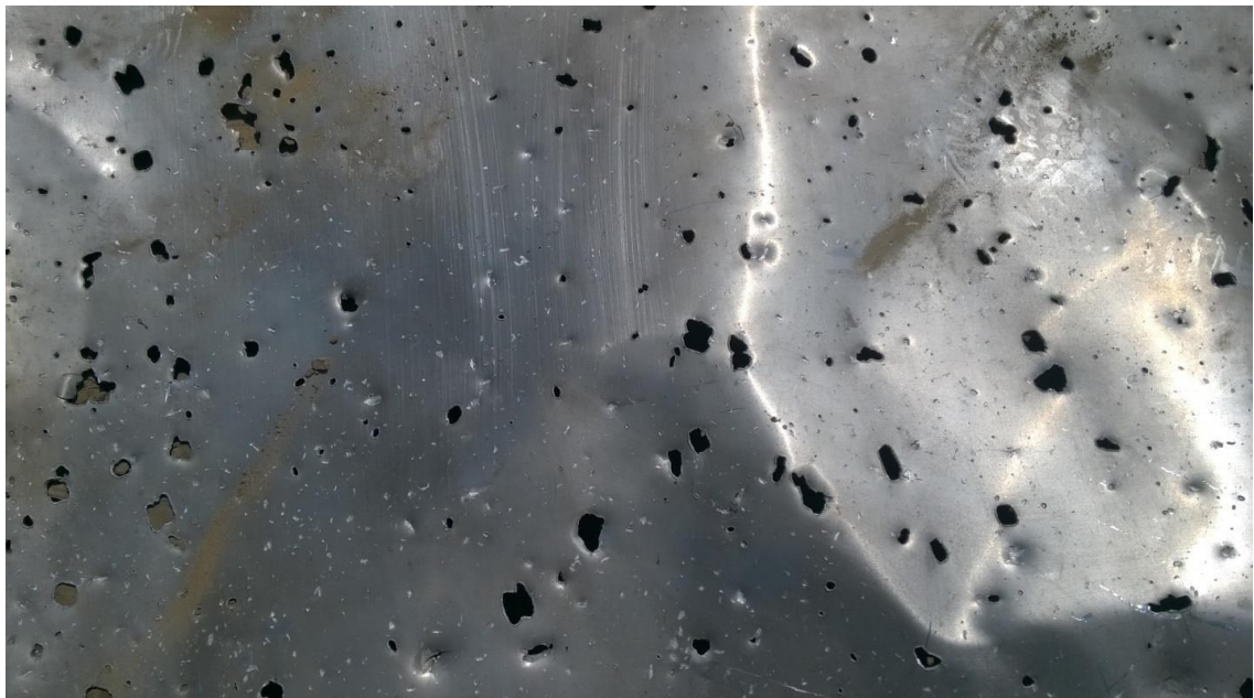
Figure A.170 - Characteristic "butterfly"-shaped holes
