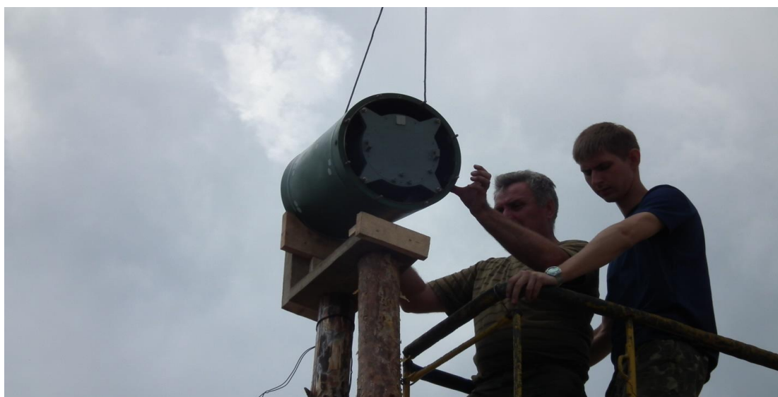
Figure A.9 - Mounting the 9H314M warhead in the second compartment hull the test bench
