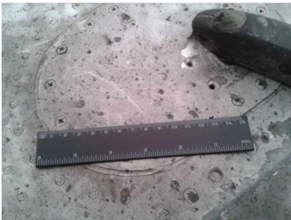
Figure 5.1.8 - Most of the fragment shows only clearly visible traces of close blast products: microcraters, thermal oxidation and soot (photo of February 2015)
