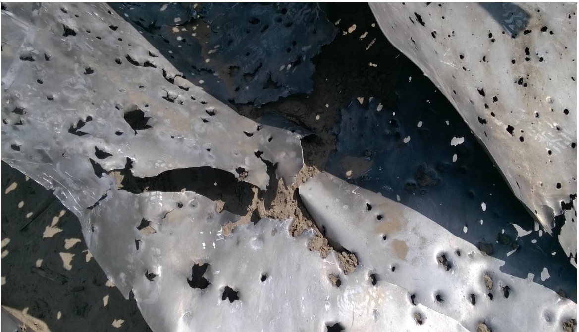
Figure A.185 - Target fragment with traces of compression, deformation and rupture of skin sheets
