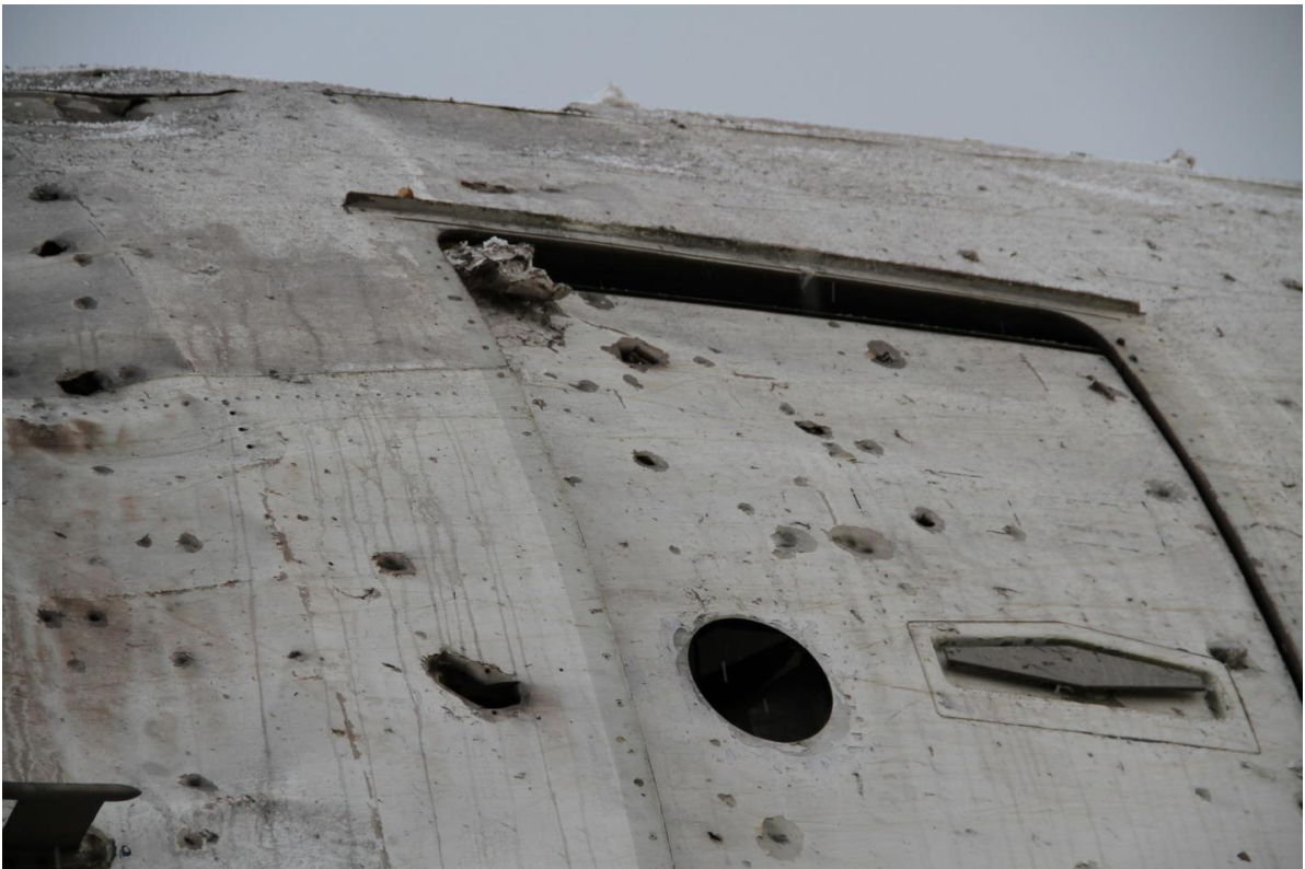
Figure 5.31 - Port side in L1 door area. Characteristic holes caused by hull fragments are seen the dimensions of which are significantly greater than those of holes caused by ready-made projectiles
