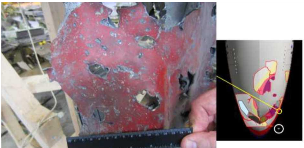
Figure 5.1.32 - Fragment of the port side below the cockpit window frame
