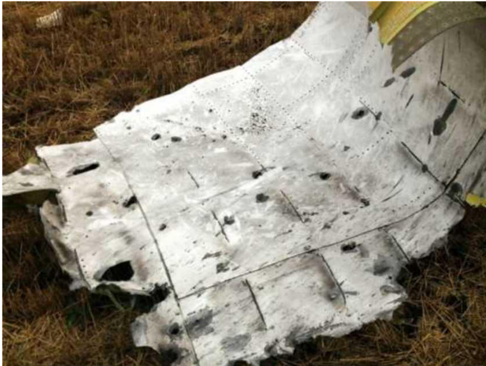
Figure A.1.6 - Exterior view of F.6 (roof behind the cockpit)
