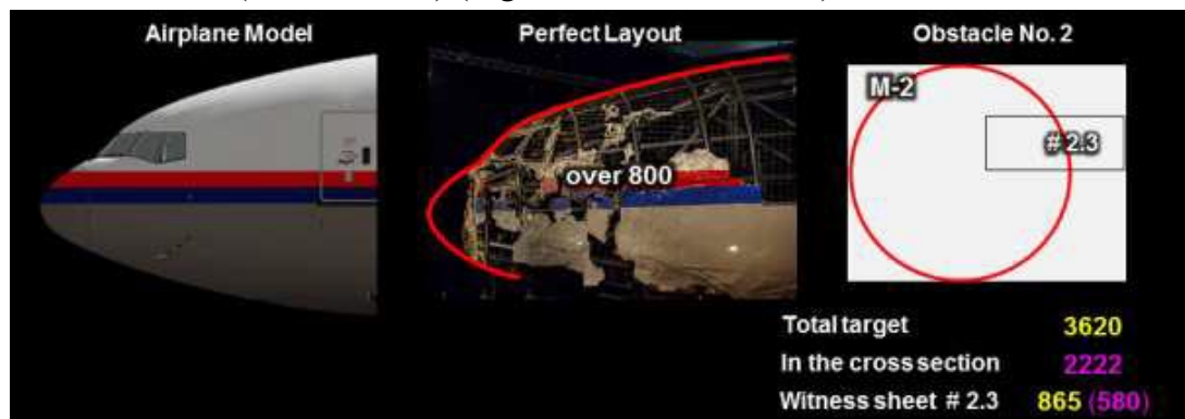
Figure G.2.5 - Comparison of target area No. 2 and its element No. 2.3 with the Boeing 777 aircraft model and final lay-out (scale observed)
