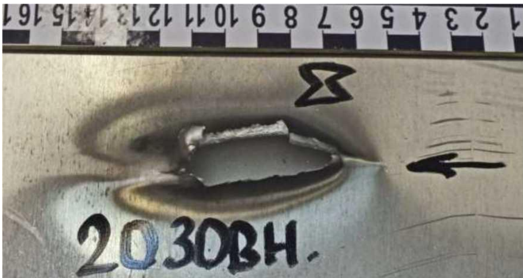
Figure B.4.14 - Experiment 2030. Exterior view of obstacle (inside view) after interaction with element No. 1 (9H314M 1-10) at an angle of 5^\circ to the firing line at 1640 m/s
