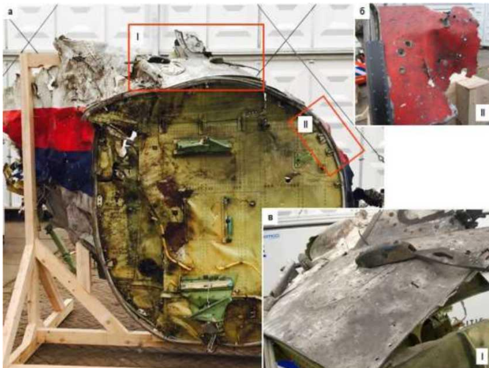
Figure A.1.3 - Exterior view of fragment "F.3" (a) and areas of the fragment with characteristic damage on the port side (b) and in front of the glazing (c)
