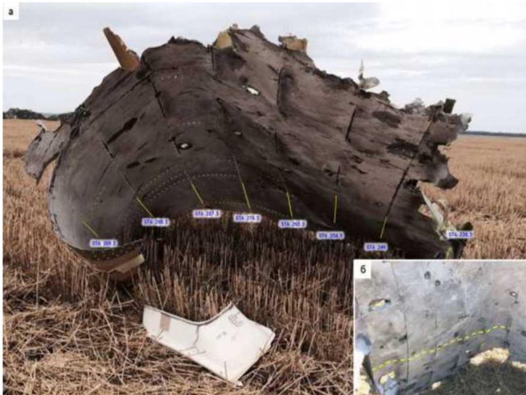
Figure 5.1.67 - Impact of blast on roof fragment above cockpit
