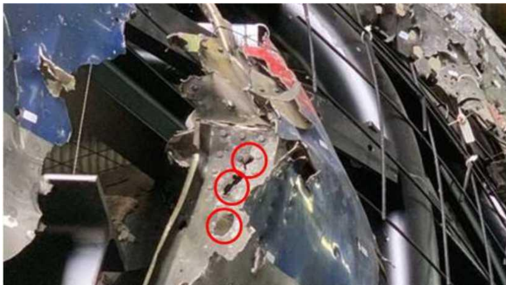
Figure 5.1.36 - Through-and-through holes in the bulkheads start from the forward boundary of the fragmentation field
