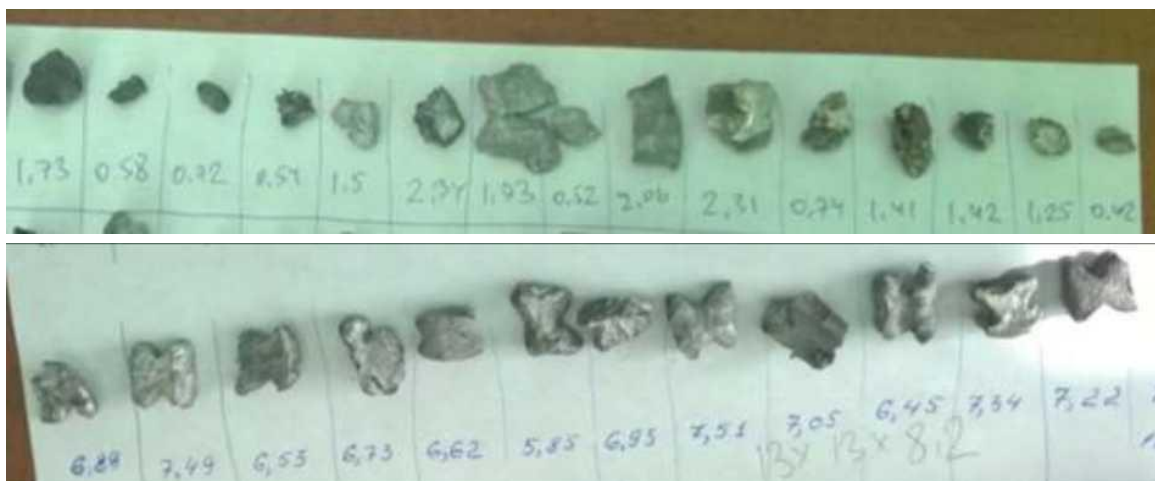
Figure 5.2.25 - Comparative linear dimensions and mass of hull fragments (top) and 9H314M heavy fraction preformed fragments 1-10 "doublet" (bottom)
