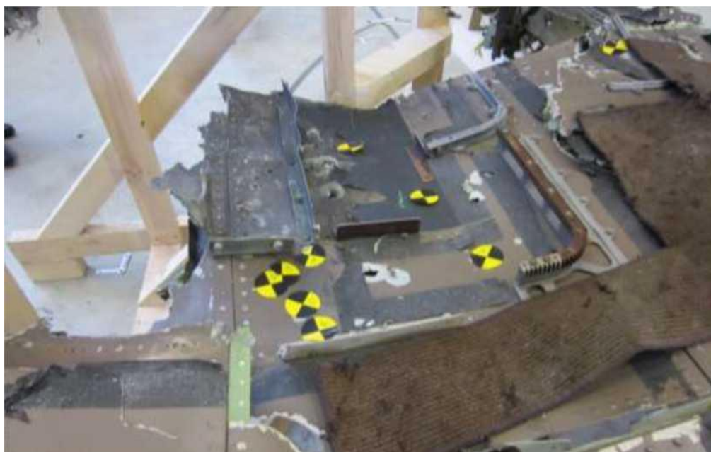
Figure 5.1.46 - Damage in the area of the commander's seat
