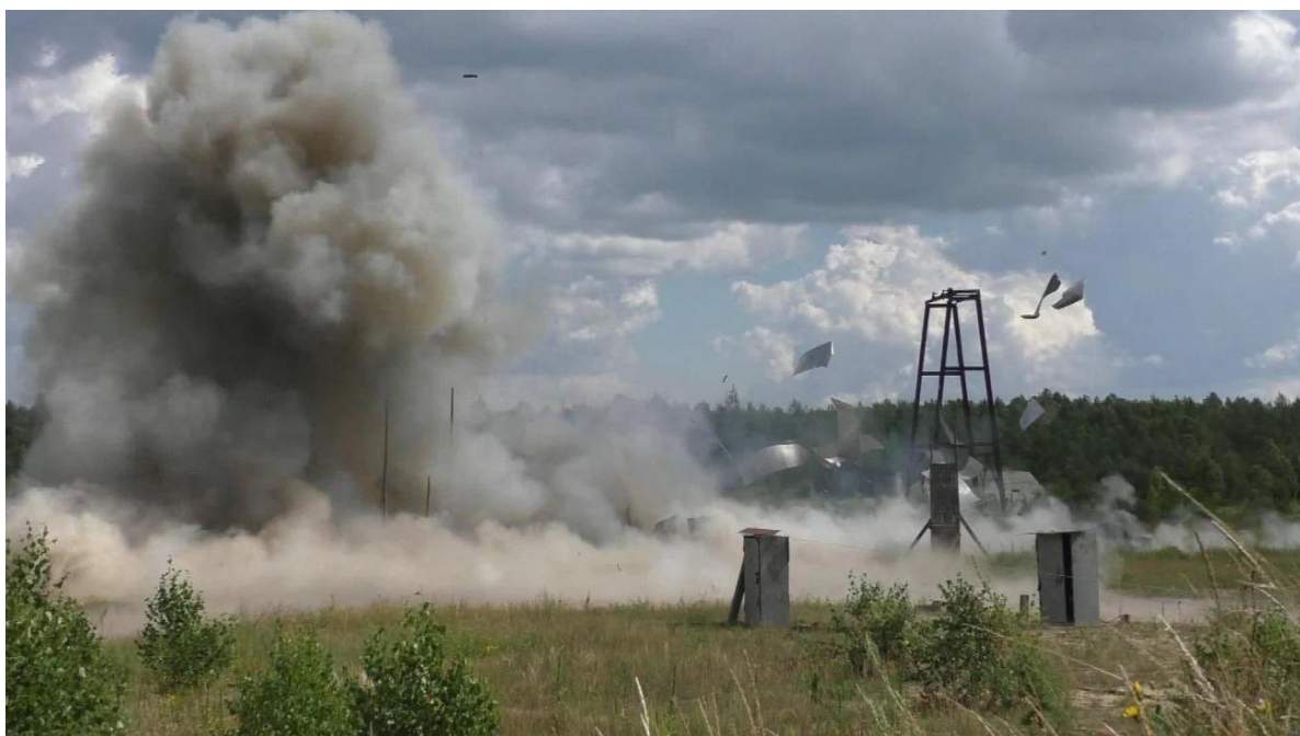
Figure A.17 - Camera No. 2P. The target layout destruction by high-explosive effect
