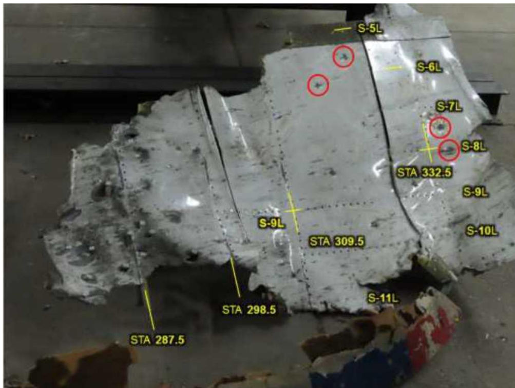
Figure 5.1.22 - Fragment of roof and top of port side behind cockpit. Through-and-through and part-through non-penetrating holes on the upper left side of the rear boundary of the coverage field are between the bulkheads STA 309.5 and STA 332.5
