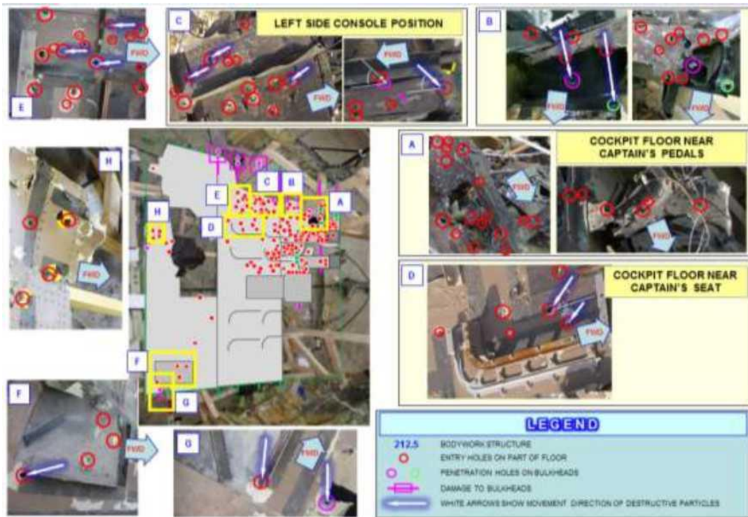
Figure 5.1.44 – Diagram showing distribution of cockpit floor and structure damage with examples of characteristic damage
