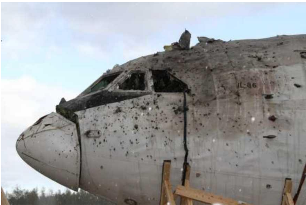
Figure A.4.18 - Thermal influence marks on the left side of the IL-86 target aircraft
