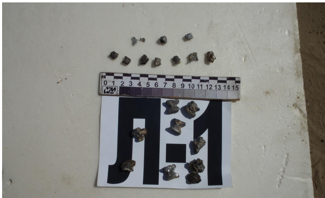
Figure A.50 – Ready-made projectiles of three fractions extracted from trap L1
