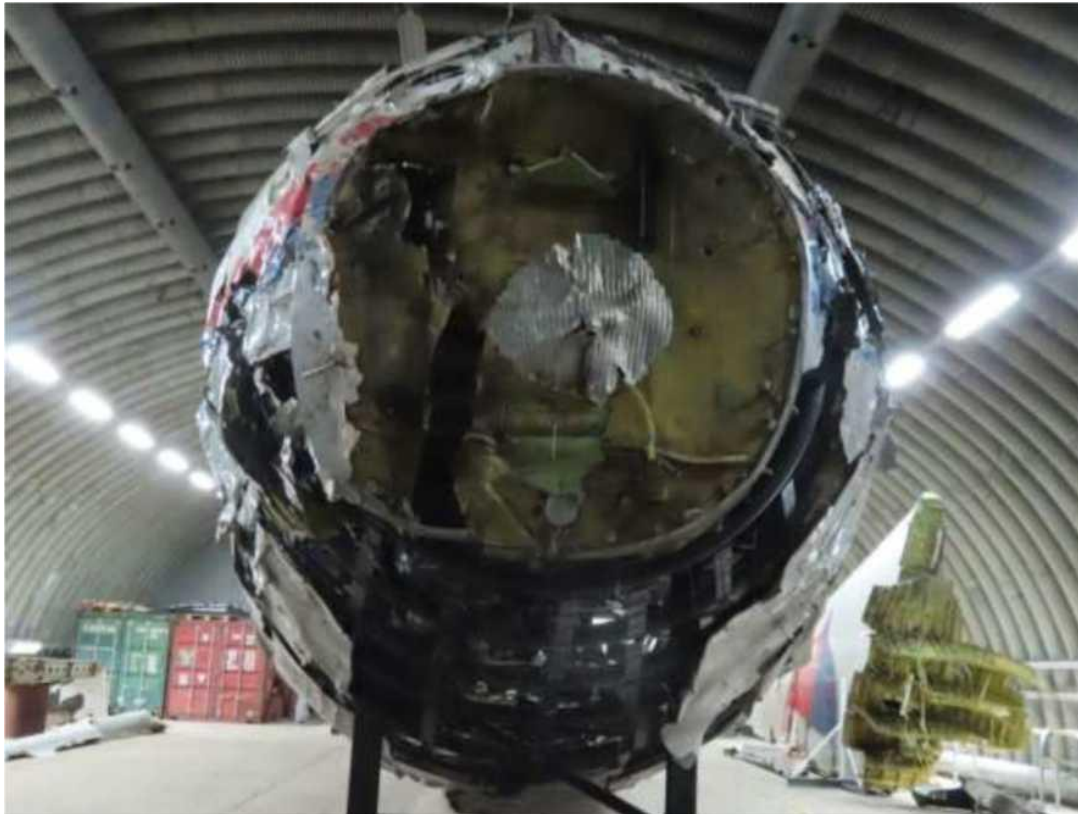
Figure 5.1.6 - Forward pressure bulkhead has no traces of fragmentation damage
