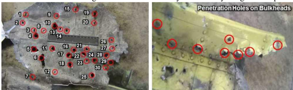
Figure F.2 - Fragment of the port side planking from the top at the rear of the third window of the Crew Commander with evidence of multiple holes in the outer planking (left) and in the bulkhead (right)
