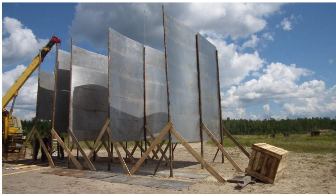
Figure A.7 - Mounting of a trap (bottom right) to collect striking elements. Rear view.
