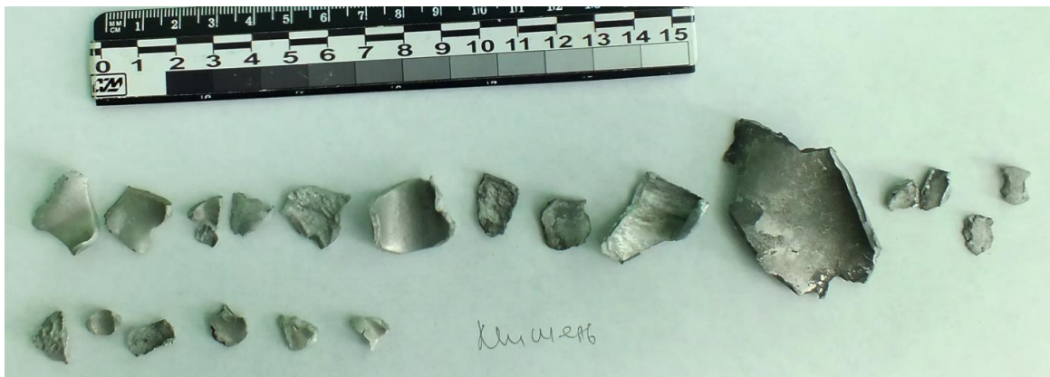
Figure A.193 - Secondary striking elements ("plugs" from target sheets)
