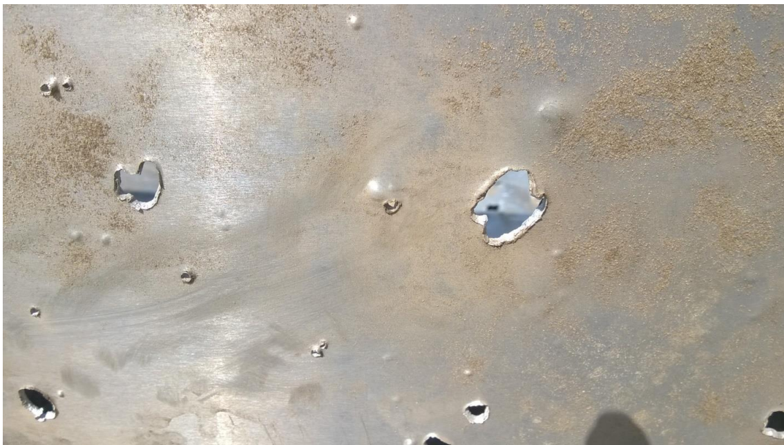
Figure A.198 - Exit holes and non-penetrating damage (view from the back of the shield)
