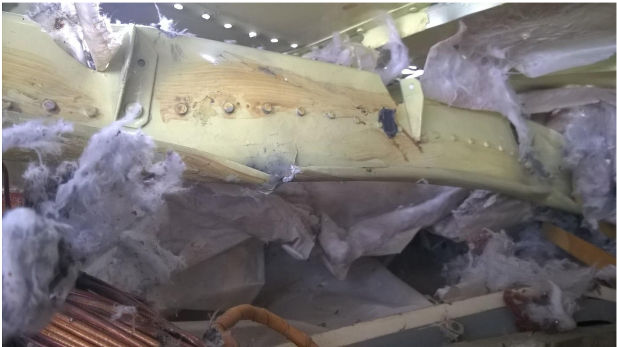
Figure 5.148 - Through-and-through hole in L-shaped frame reinforcement on the left side of the cockpit
