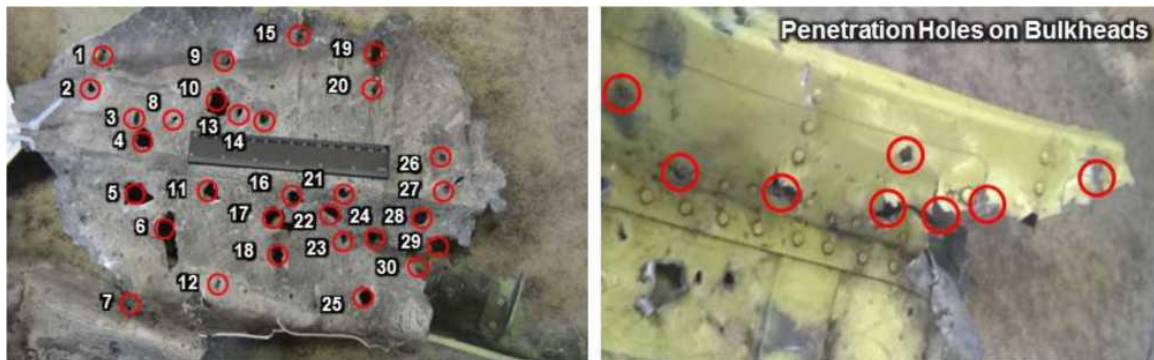
Figure F.16 - Fragment of port side no 3 actually has multiple damage to the outer skin and force element, indicating that the fragment was in a dense fragmentation stream
