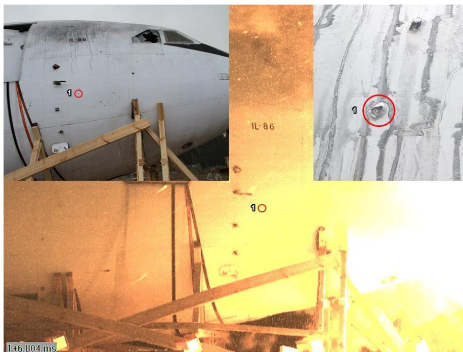
Figure 7.11 - Through-and-through hole in the starboard side made by a projectile
