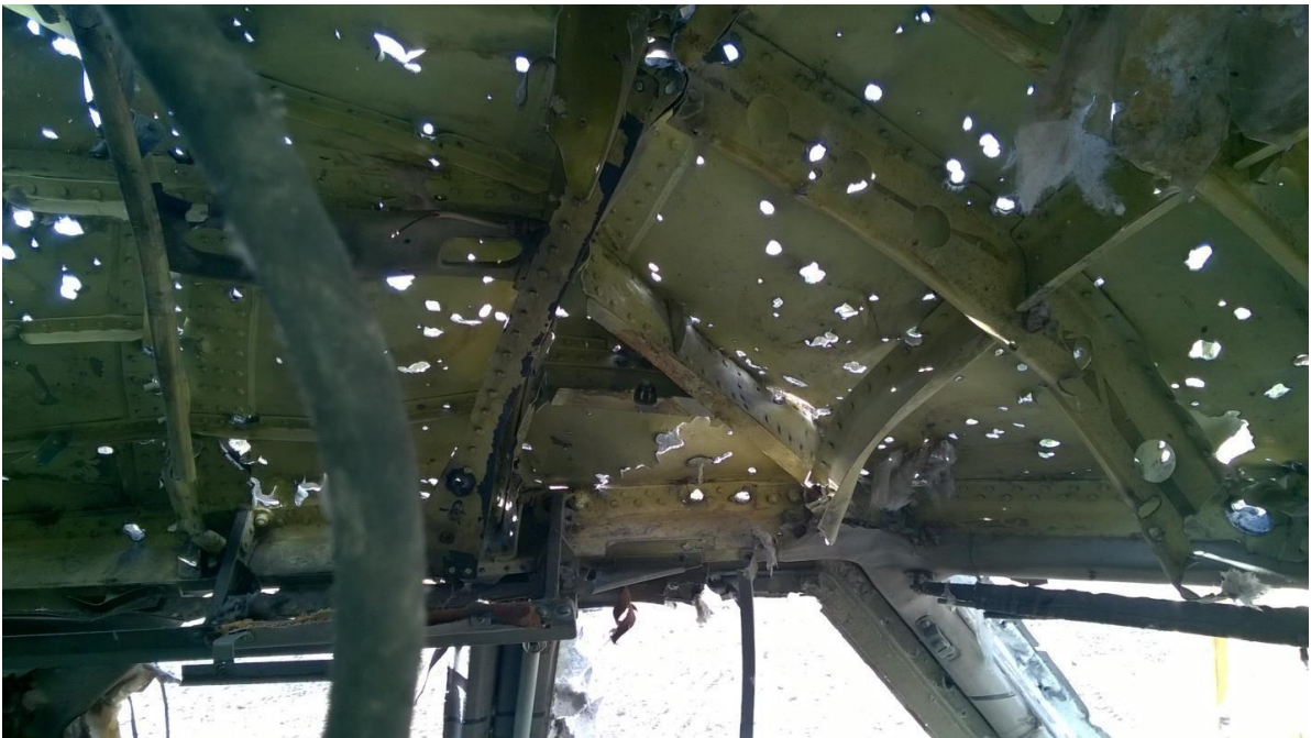
Figure 5.68 - Characteristic butterfly-shaped through-and-through holes in a fragment of the cockpit roof
