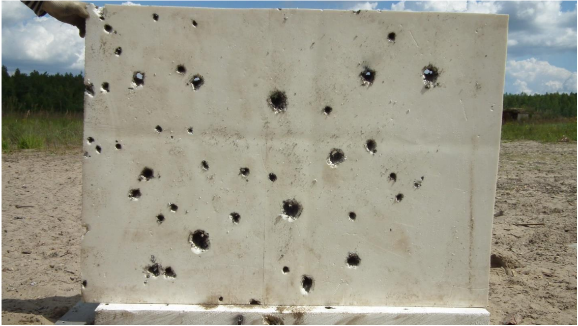
Figure A.35 - Second barrier of trap L1 (second layer of foam plastic PS-1-150) after the testing
