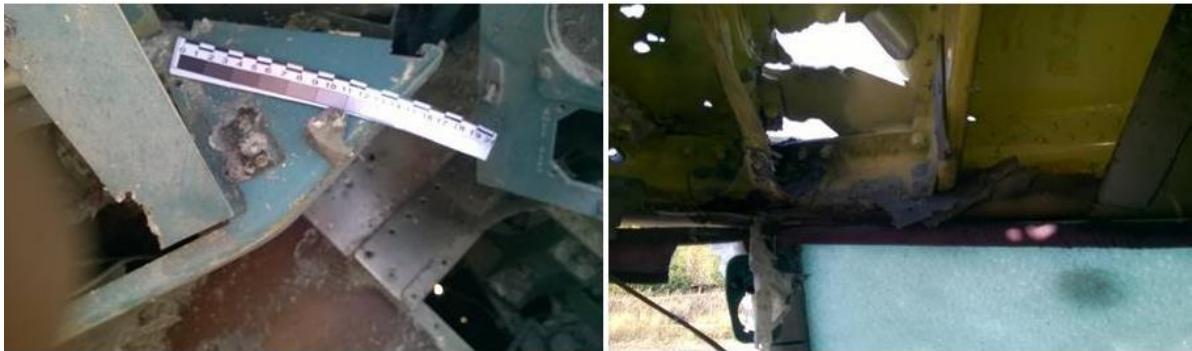
Figure 5.78 - Missile compartment hull fragments (left) and holes caused by them (right)
