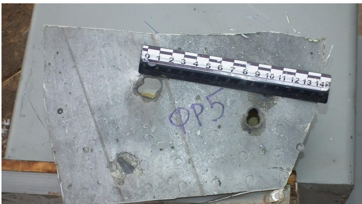
Figure 5.169 - Fragment No. 5 before extraction (internal view). The blue bar shows the trajectory of entry of a projectile of 9H413M 1-10, which, after piercing the outer skin, penetrated the L-shaped reinforcement of a frame
