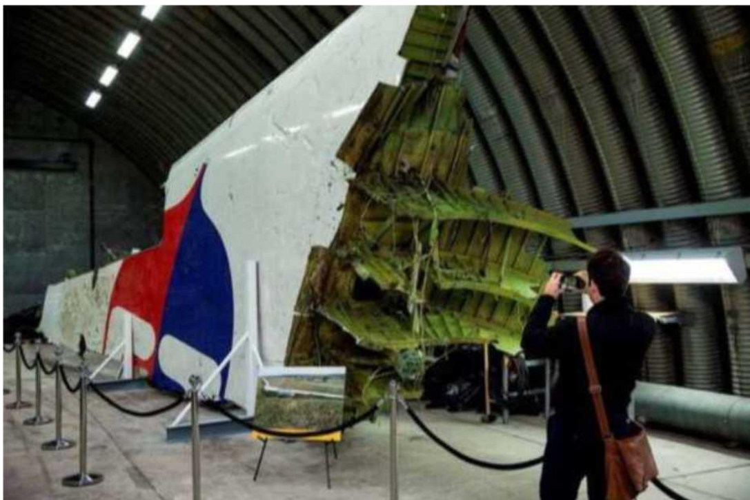
Figure G.1.7 - Vertical stabiliser in final reconstruction
