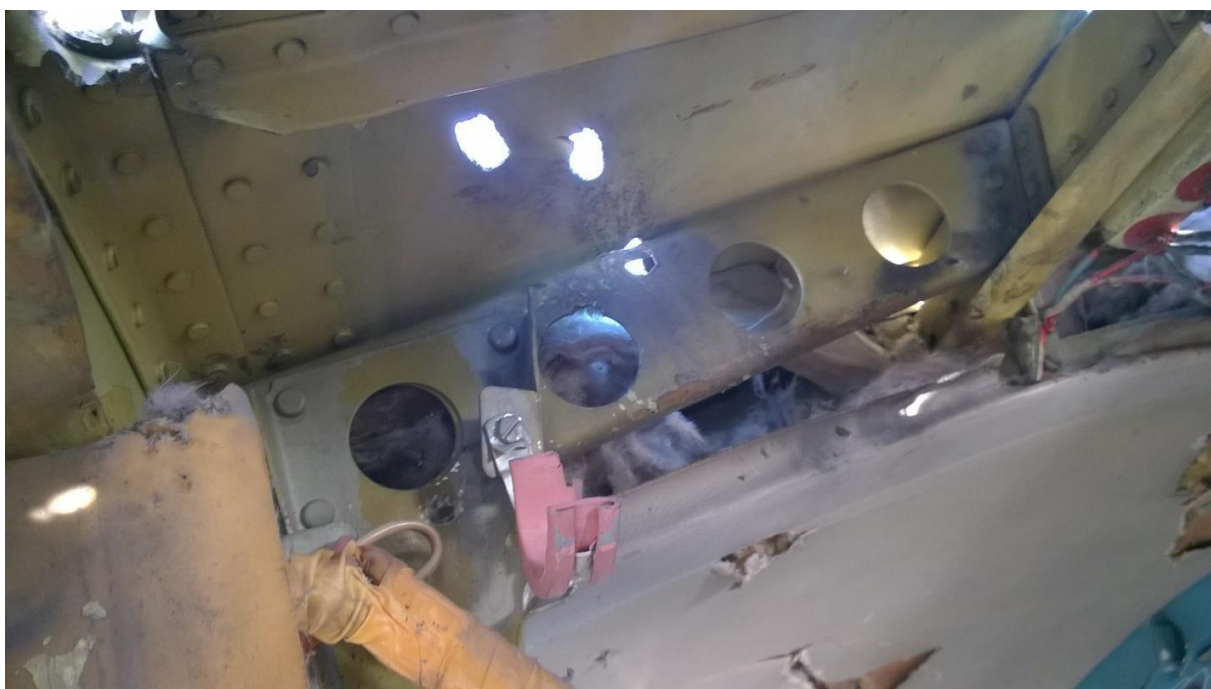
Figure 5.146 - Through-and-through holes in the roof and cockpit stringer (right side)
