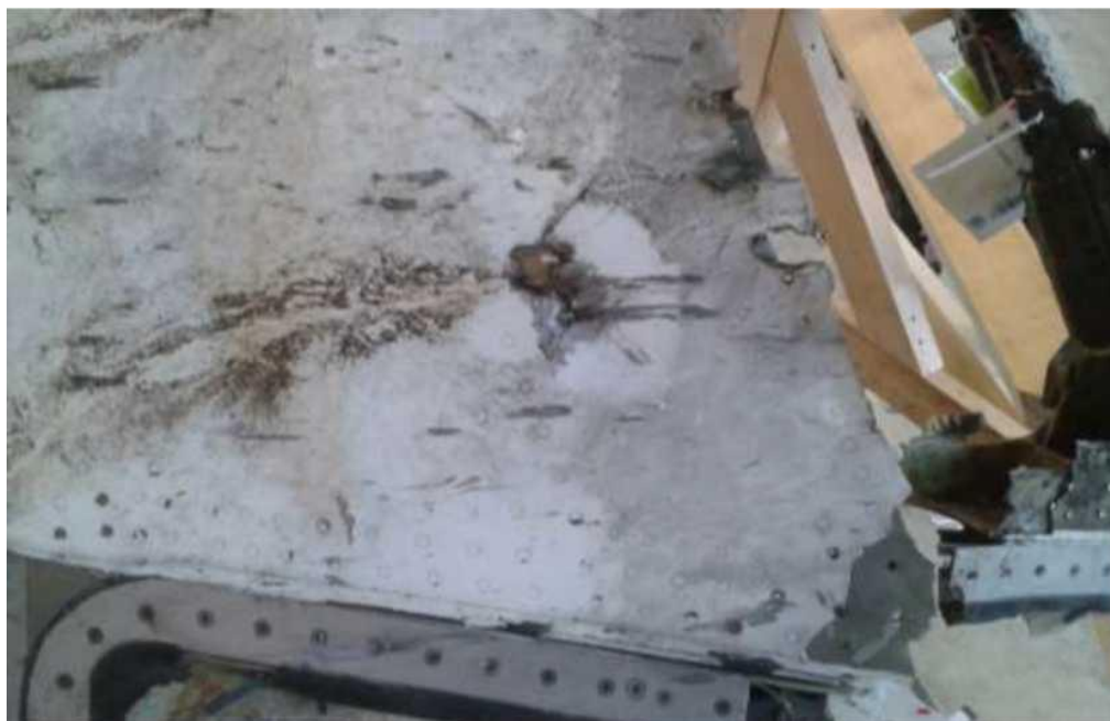
Figure 5.1.17 – Damage near the right boundary of the coverage field corresponds to the level of the upper right-hand corner of the right-hand pilot's front window
