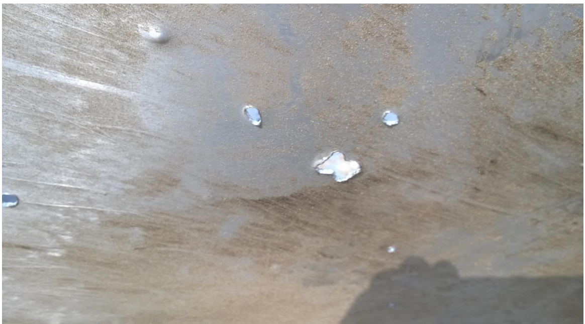
Figure A.200 - Exit holes with jagged edges and non-penetrating damage on target No. 4 (view from the back of the shield)
