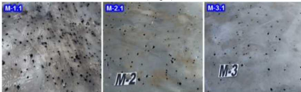
Figure G.1.31. Variation of the fragmentation field density as a function of the distance of the target elements from the detonation point. In the shield target layout created for the full-scale experiment, target No. M-3.1 (right) was placed approximately twice as far from the detonation point as target No. M-1.1 (left)
