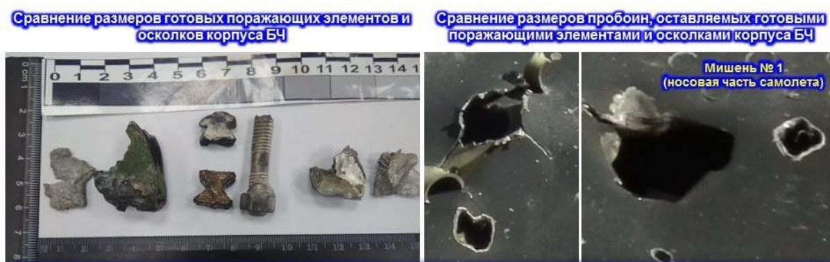
Figure 9.1 - Second compartment (warhead compartment) hull fragments
