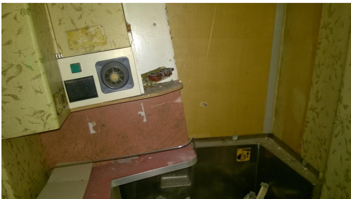
Figure 5.138 – Exit holes in the lower right section of the first passenger compartment (rear view)
