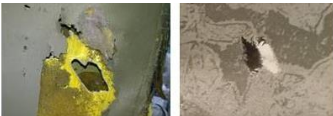
Figure 5.140 - Characteristic butterfly-shaped holes in the fragments of the cockpit's interior
