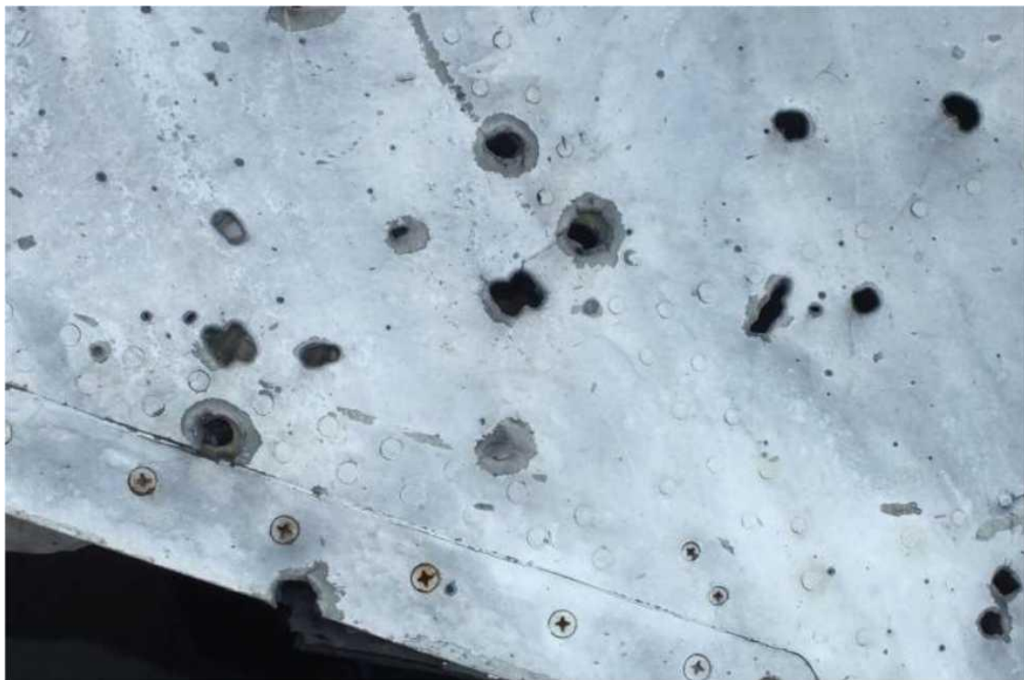
Figure A.4.8 - Fragment of the outer skin above the glazing of the aircraft commander (IL-86 target aircraft)
