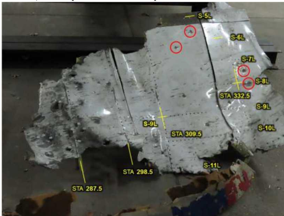
Figure G.1.6 - Fragment of roof and upper part of the port side behind the cockpit. The fragmentation damage is located between bulkheads STA 309.5 and STA 332.5, which is almost 3 metres further than the DSB 'reference'
