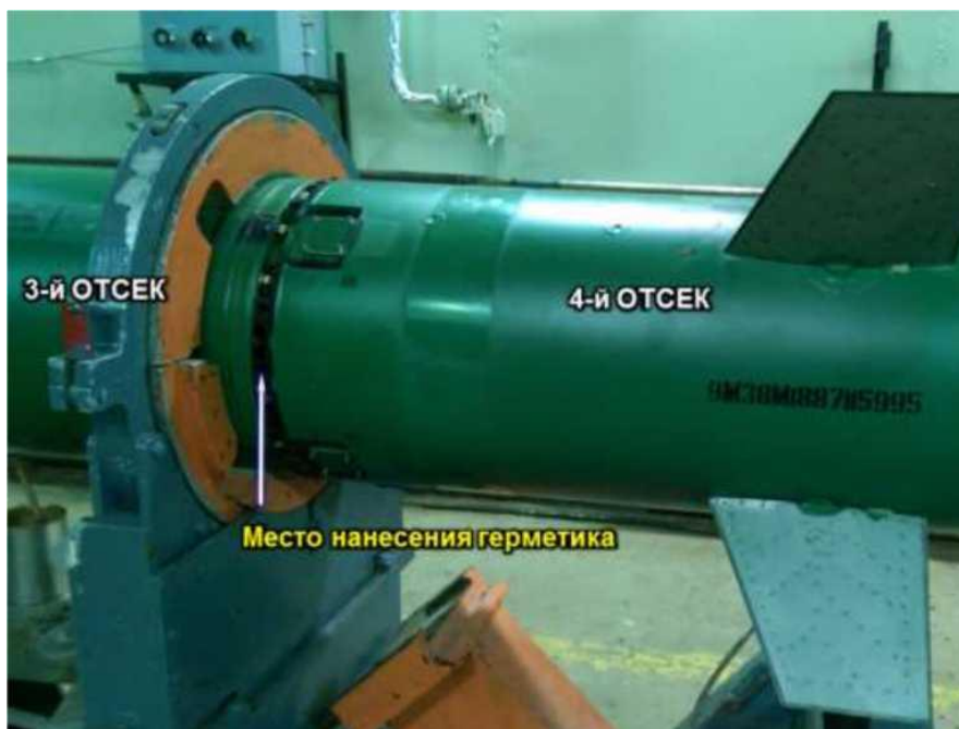
Figure E.5 - Docking of the third and fourth compartments. At the front of the fourth compartment there is also a wing attachment point: before the fourth compartment is docked to the engine, the wing cannot be installed on the rocket (resource - preparation materials for the second field experiment)
