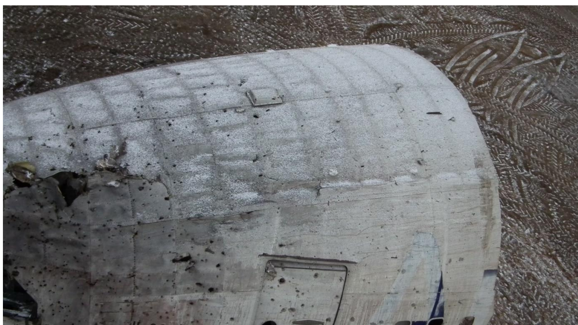
Figure 5.45 - Port side skin with characteristic butterfly-shaped holes caused by 9H314M 1-10 projectiles (close-up)
