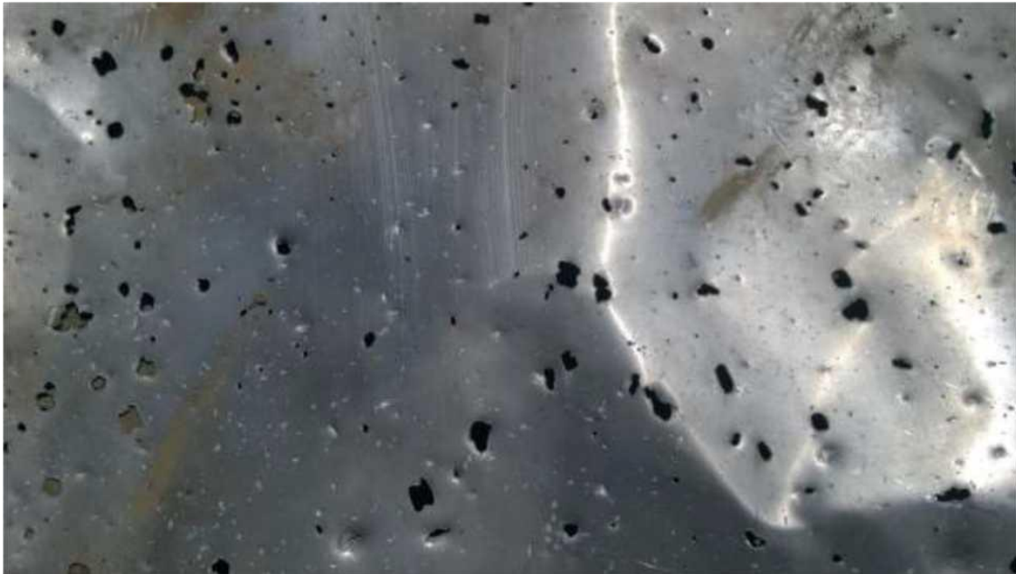
Figure A.4.10 - Characteristic "butterfly" shaped holes in shielded target sheets
