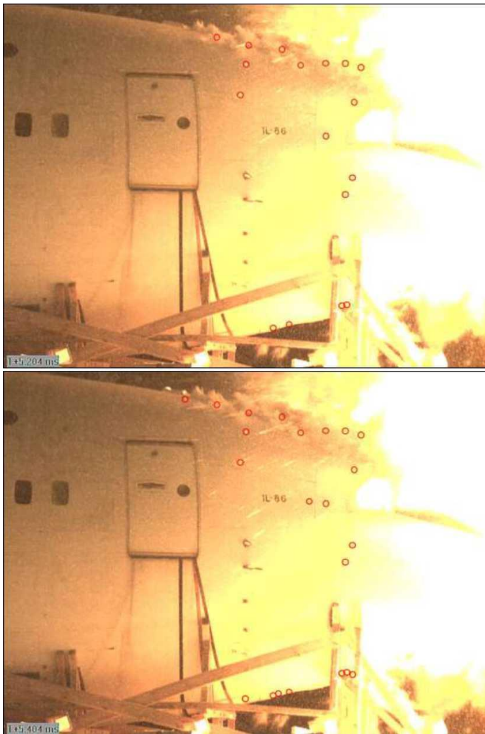
Figure B.3.12 - Puncturing the starboard side of the target aircraft IL-86 (top - T+ 5.204 ms; bottom - T+ 5.404 ms)
