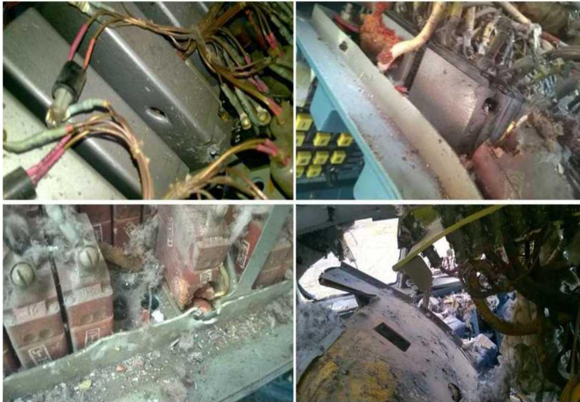
Figure C.6 - Material-intensive components of on-board avionics equipment of the IL-86 target aircraft (starboard and starboard side of the roof)
