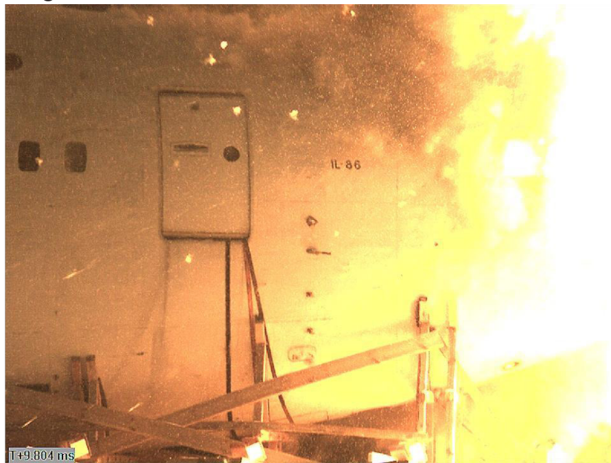
Figure 4.21 - Detonation of the 9H314M warhead
