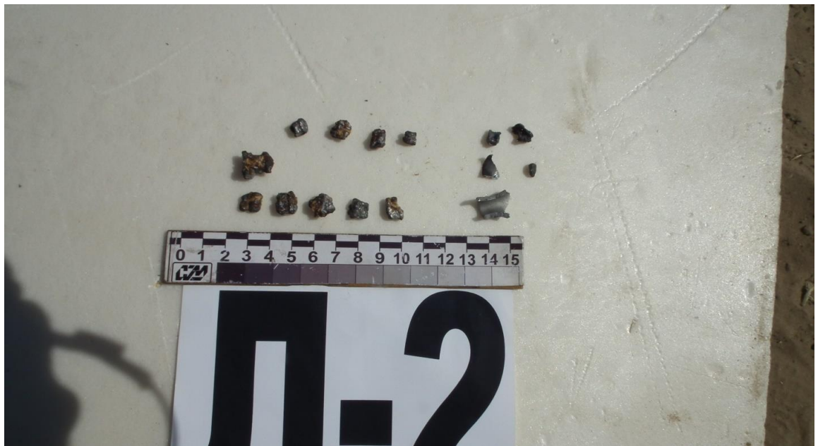
Figure A.52 - Ready-made projectiles and hull fragments (those of the compartment hull) removed from trap L2
