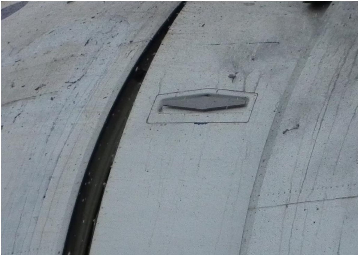
Figure 5.104 - Exit holes in R1 door area
