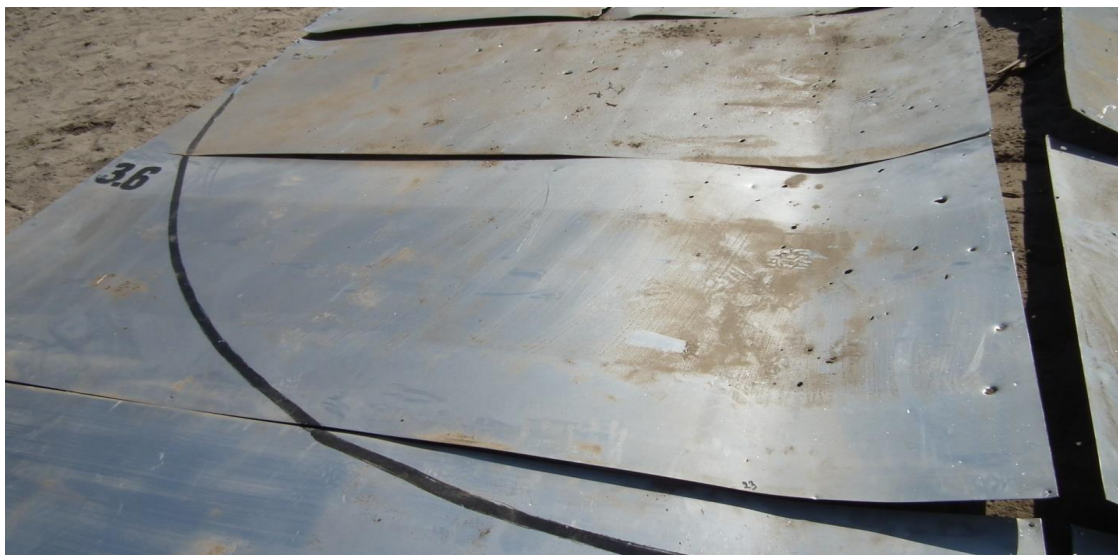
Figure A.104 - Fragments 3.4 (top), 3.6 and 3.8 (bottom) of target No. 3
