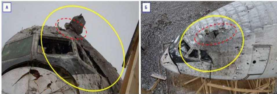
Figure A.4.17 - Destruction of the target aircraft's load-bearing structure of the IL-86
