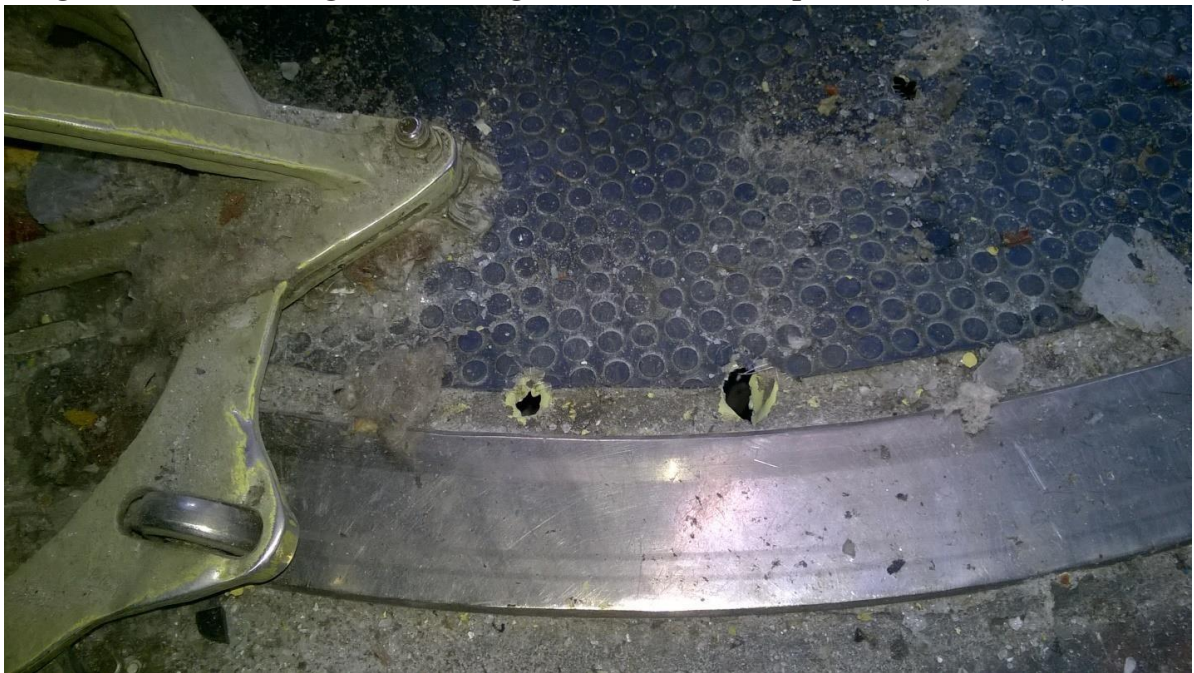
Figure 5.125 - Through-and-through holes in the cockpit floor (central part of the cockpit)
