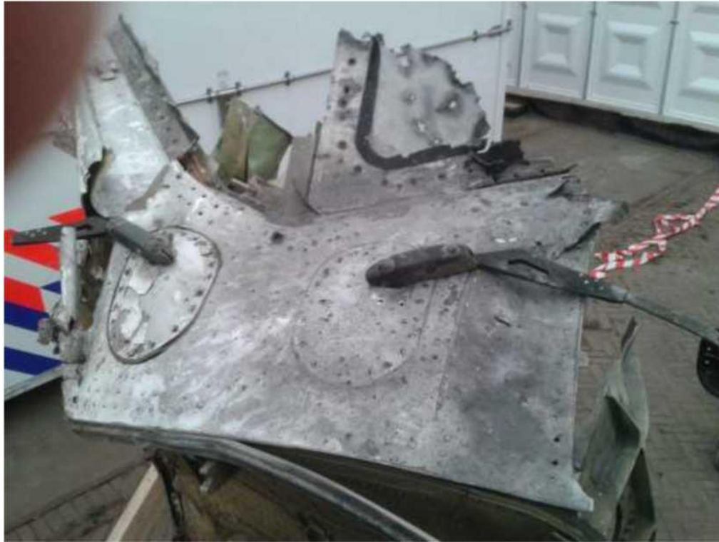
Figure 5.2.34 - Fragment of the nose of a Boeing 777, adjacent to the front bulkhead from above (photo February, 2015)
