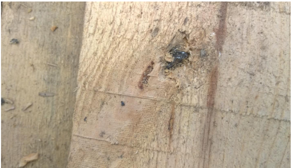
Figure A.45 - General view of a projectile lodged in trap L1
