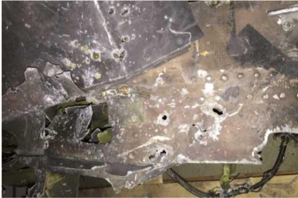
Figure 5.1.47 - Damage density in cockpit floor to the left of the aircraft commander's seat (along the port side)
