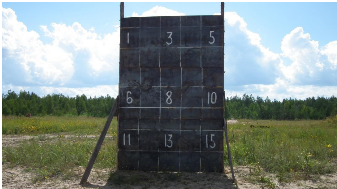
Figure A.6 - Additional shield target (target No. 6M.D) imitating the left engine of a Boeing 777-200 aircraft
