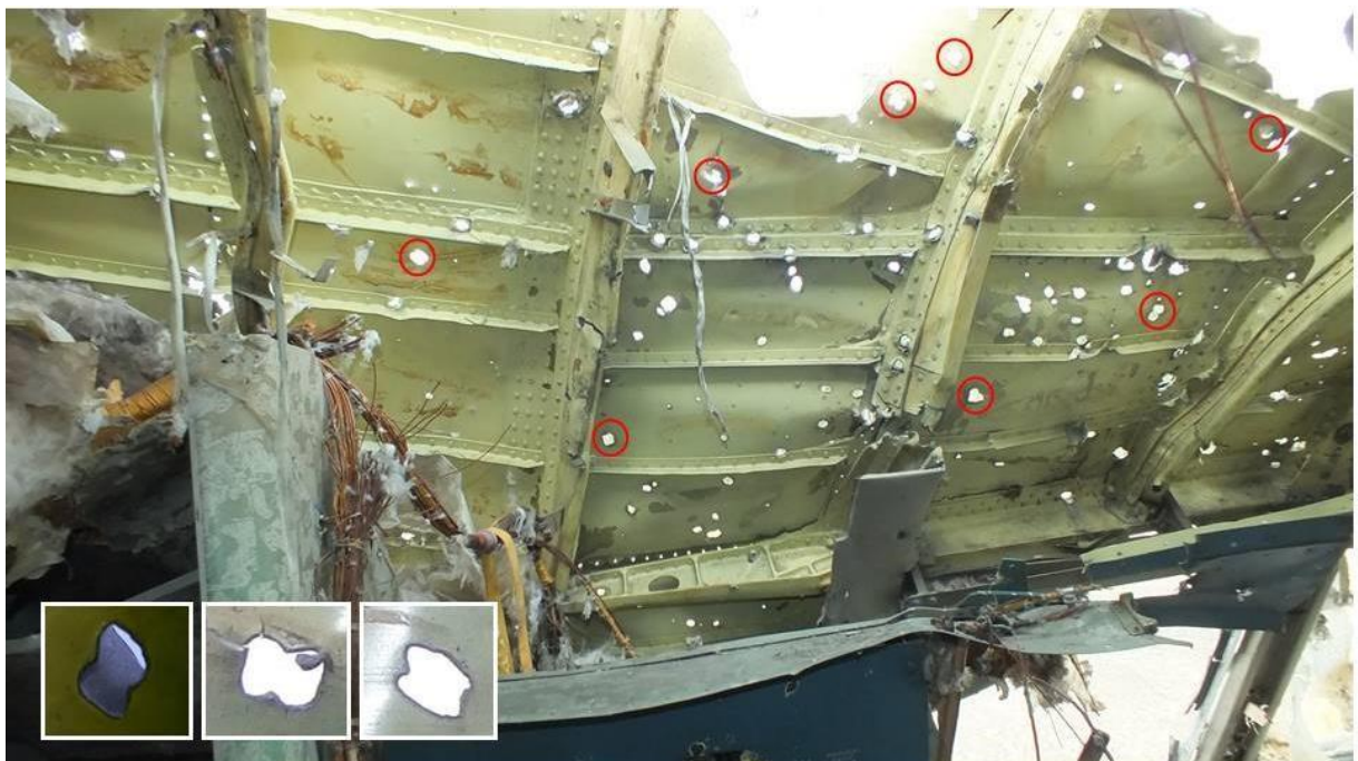
Figure 6.3 - Port side of the cockpit (inside view)
