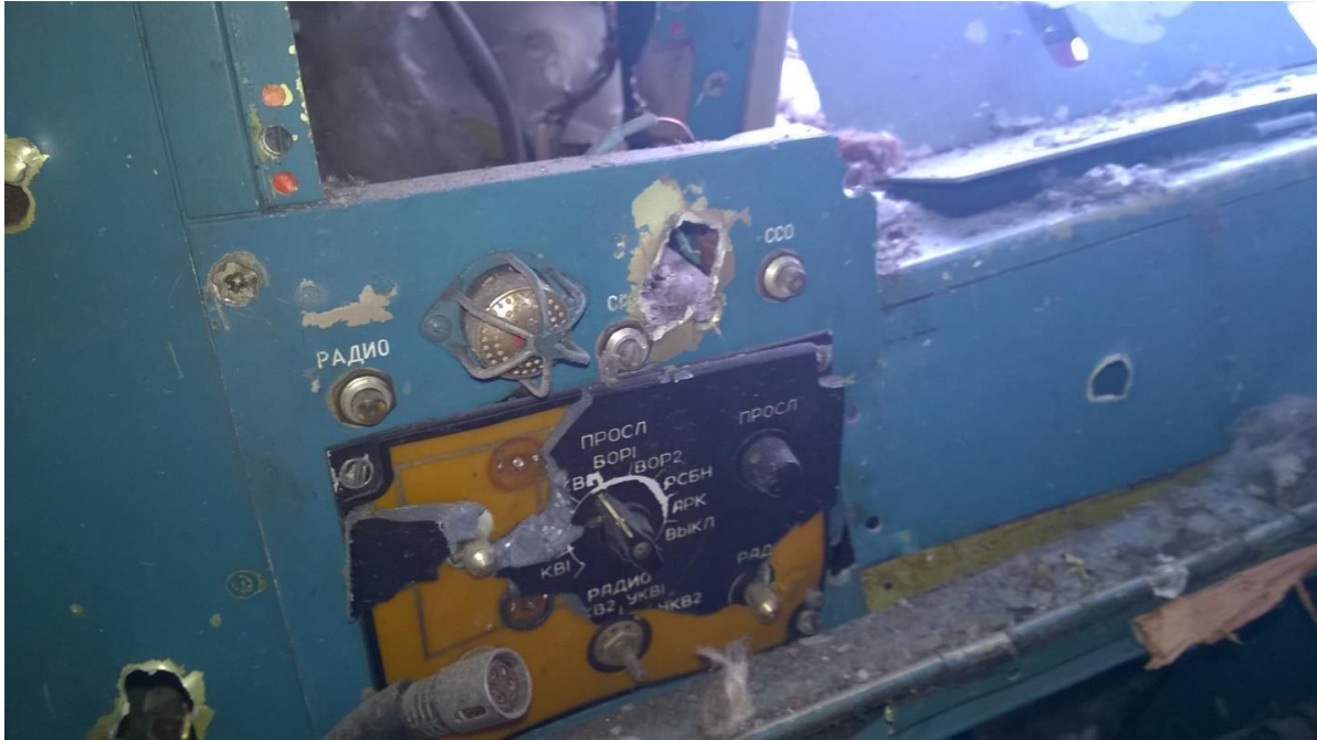
Figure 5.113 – Exit holes in the instrumentation cabinet on the port side (view from inside the cockpit)
