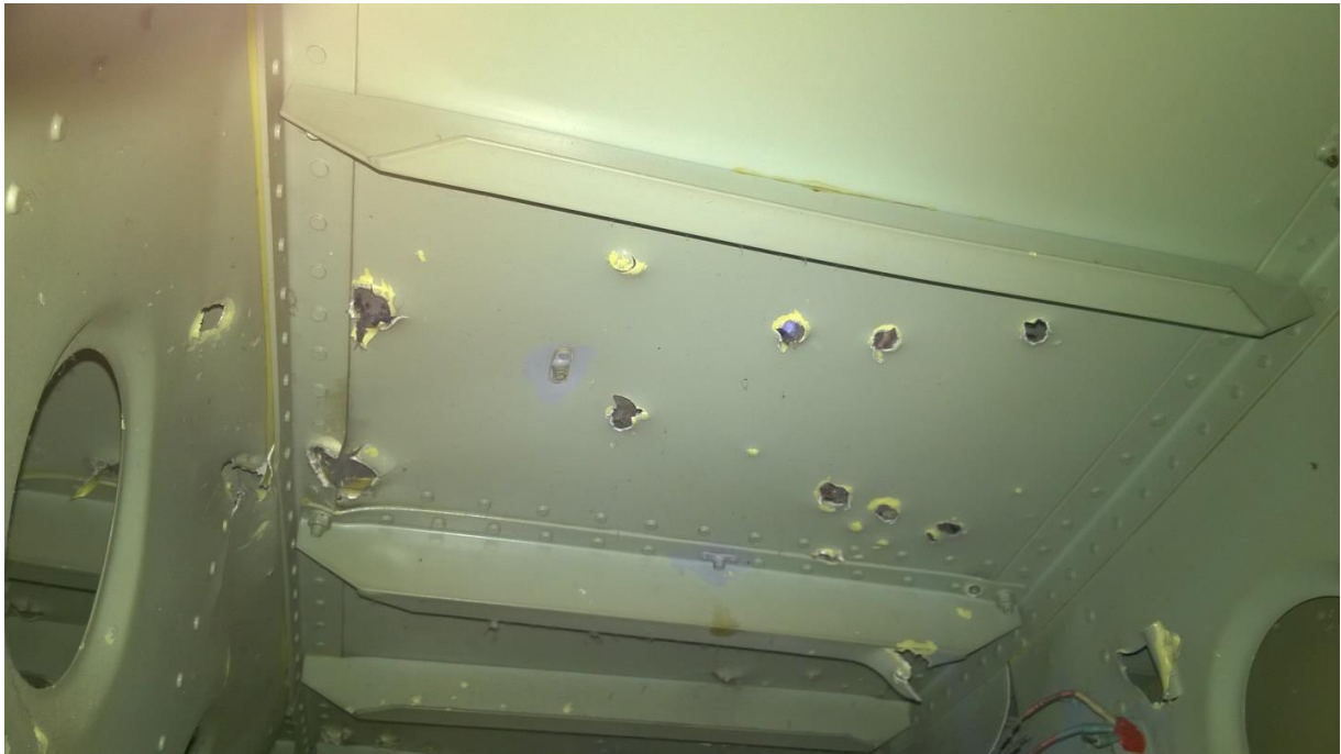
Figure 5.132 - Through-and-through holes in the cockpit floor (bottom view)
