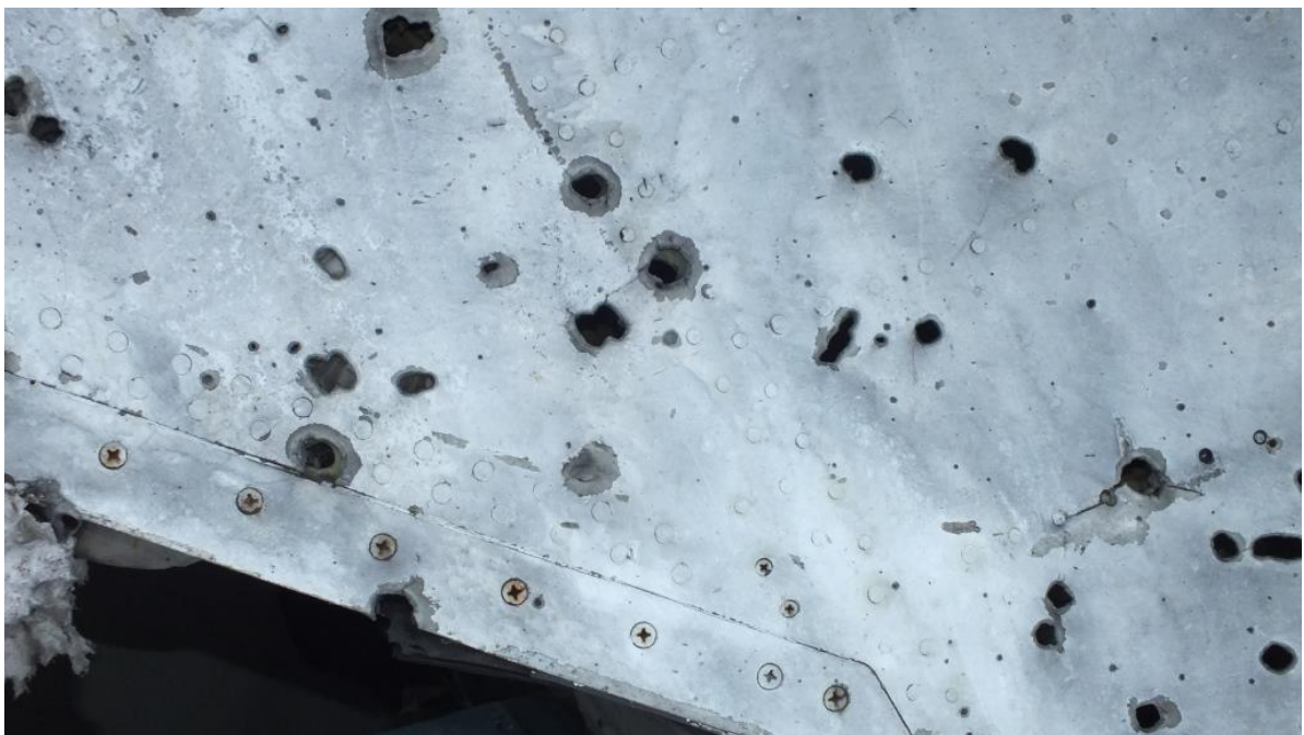
Figure 5.44 - Port side skin with micro-crater marks and characteristic butterfly-shaped holes caused by 9H314M 1-10 projectiles (close-up)
