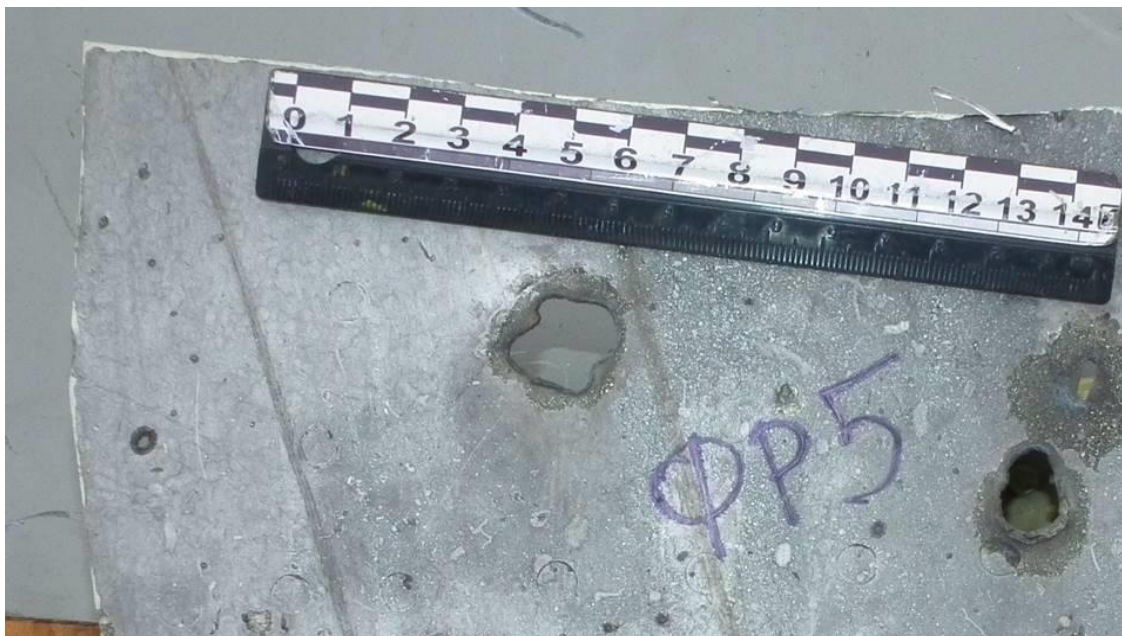
Figure 6.13 - Appearance of a characteristic butterfly-shaped hole in the outer skin of the target aircraft (external view)
