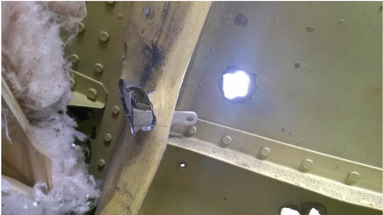
Figure 5.148 - Through-and-through hole in L-shaped frame reinforcement on the left side of the cockpit
