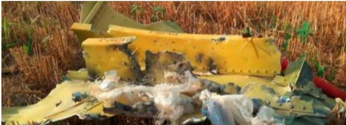
Figure 5.1.41 - Fragment of the centre port side behind the cockpit. Holes in the STA 287.5 and STA 298.5 bulkheads and traces of compression, deformation, tearing and breaking of structural elements are objectively observed
