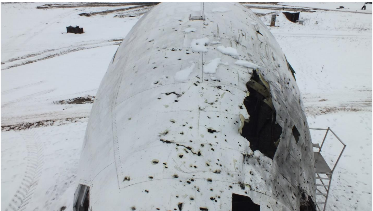
Figure 5.60 - Cockpit roof after removal of fragments (top front view)
