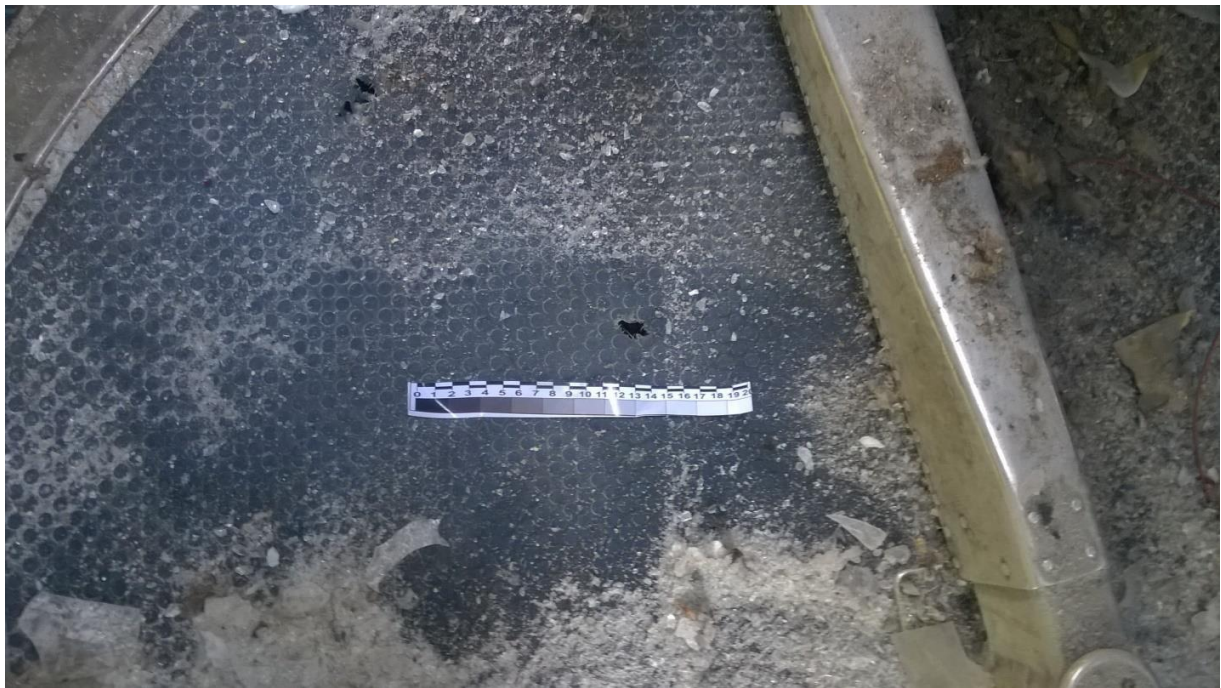
Figure 5.126 - Through-and-through holes in the cockpit floor
