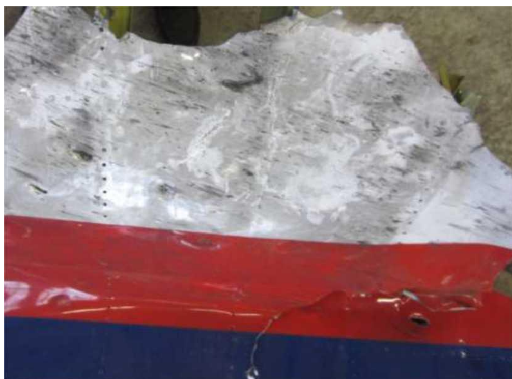
Figure 5.1.15 - Though-and-through and part-through non-penetrating damage at the lower boundary of the coverage field between bulkheads STA 276.5 (left), STA 287.5 (centre) and STA 298.5 (right)
