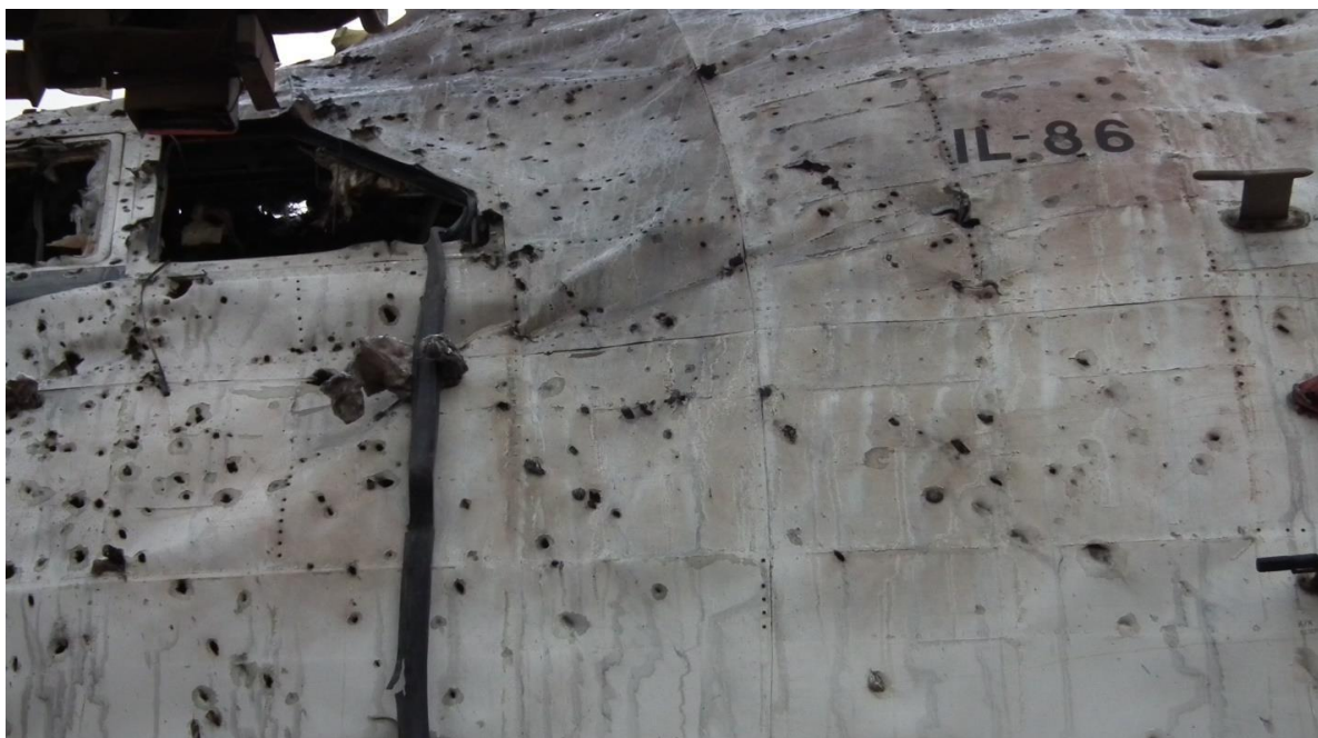
Figure 5.37 - Fragment of the outer skin of the port side (overall view). The fragment shows deformation of the outer skin in the direction from outside to inside, exposing the contours of the framework and detachment of outer skin elements
