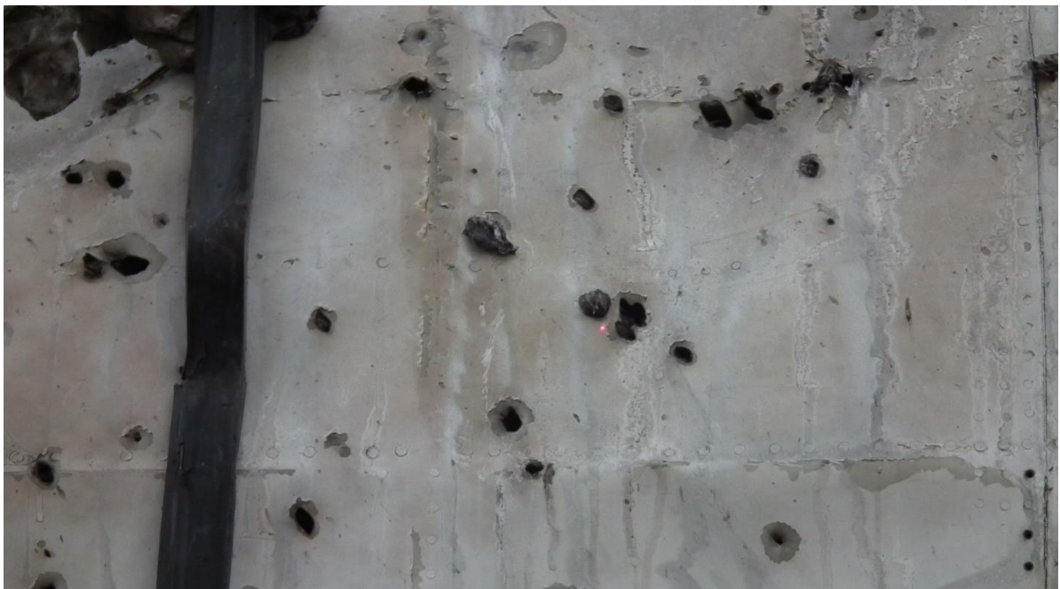
Figure 5.40 - Port side skin (close-up). No traces of non-penetrating damage (ricochets) caused by preformed fragments on the port side of the target aircraft
