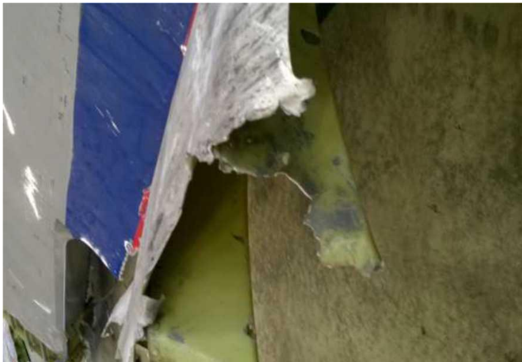
Figure A.3.6 - Destruction of port side bulkheads by perforation
