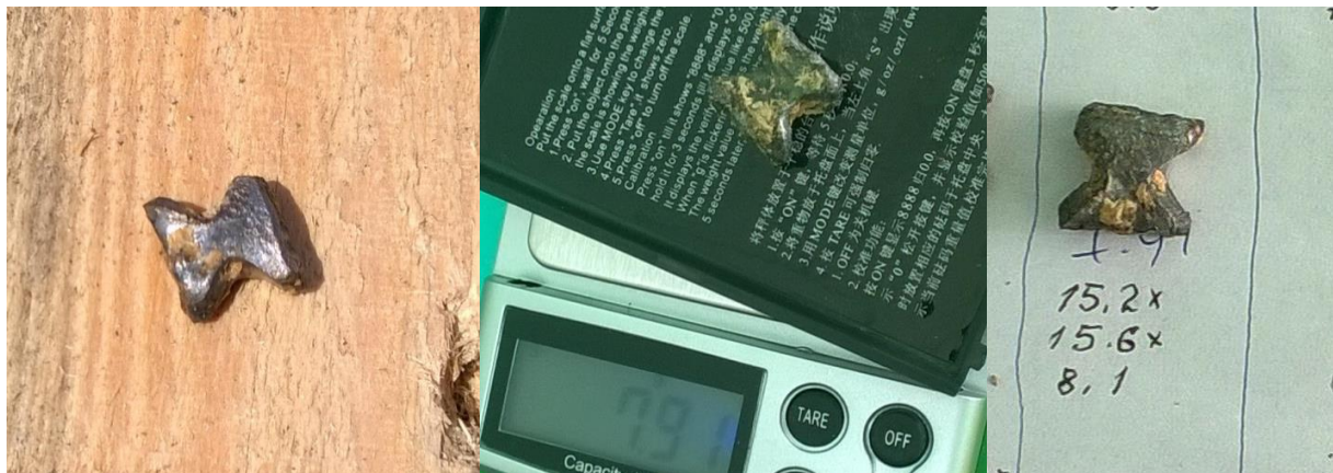
Figure 8.10 - 9H314M 1-10 projectile: after removal from the trap (left), at weighing (centre) and after dimensional measurements (right)
