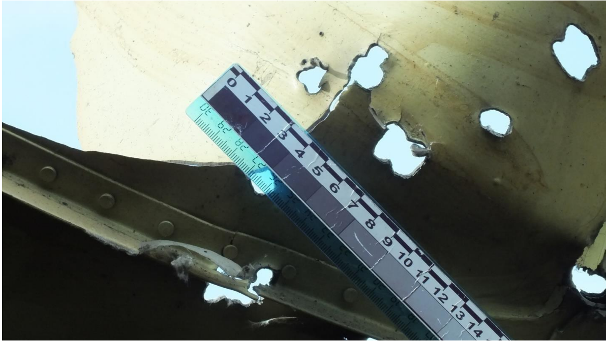
Figure 5-77 - Characteristic butterfly-shaped holes (inside view)
