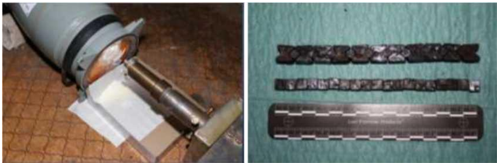
Figure J.1.18 - Test samples of a bursting charge (left) and three fractions of projectiles (right). Materials of Ukraine
