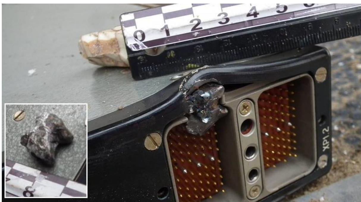
Figure 8.6 - Removing a 9H314M 1-10 projectile from avionics equipment
