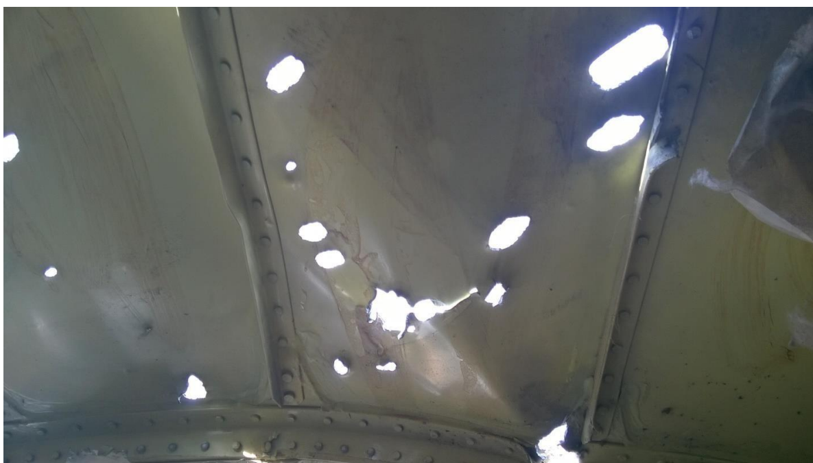
Figure 5.75 - Through-and-through holes in the central and right sections of the cockpit roof (inside view)
