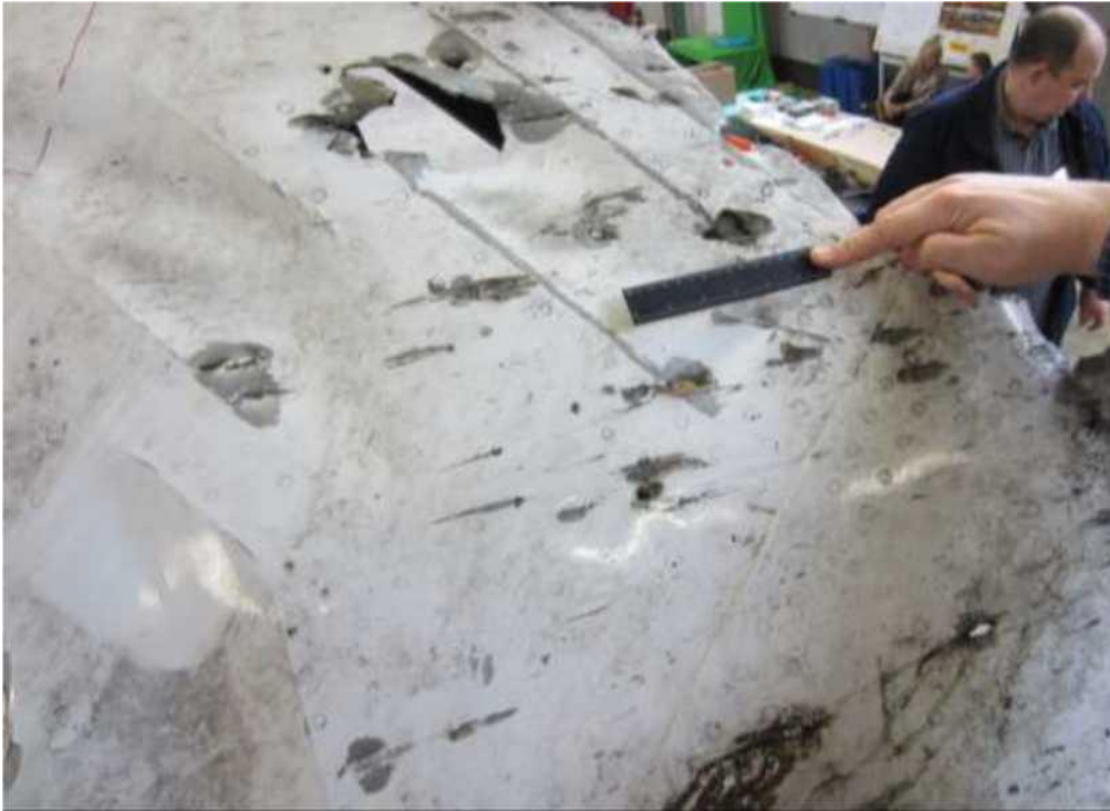
Figure 5.1.18 - Boundary damage to the right side of the cockpit
