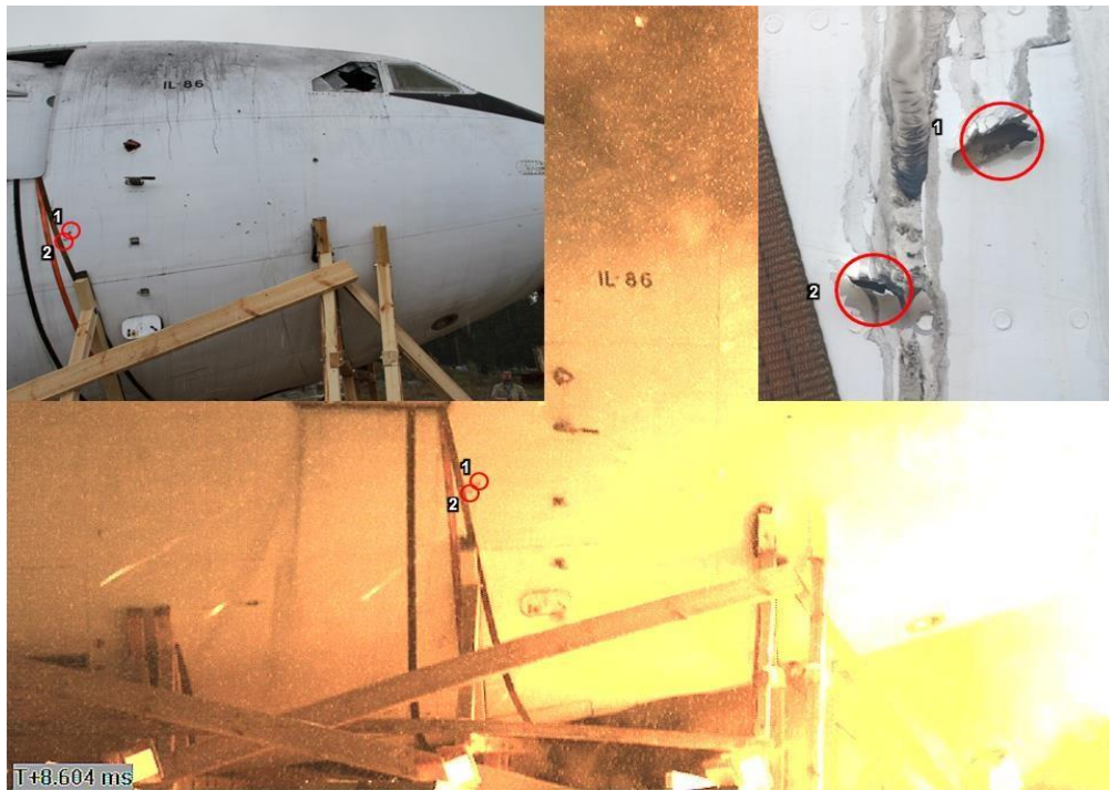
Figure 7.12 - Through-and-through hole in the starboard side made by projectiles
