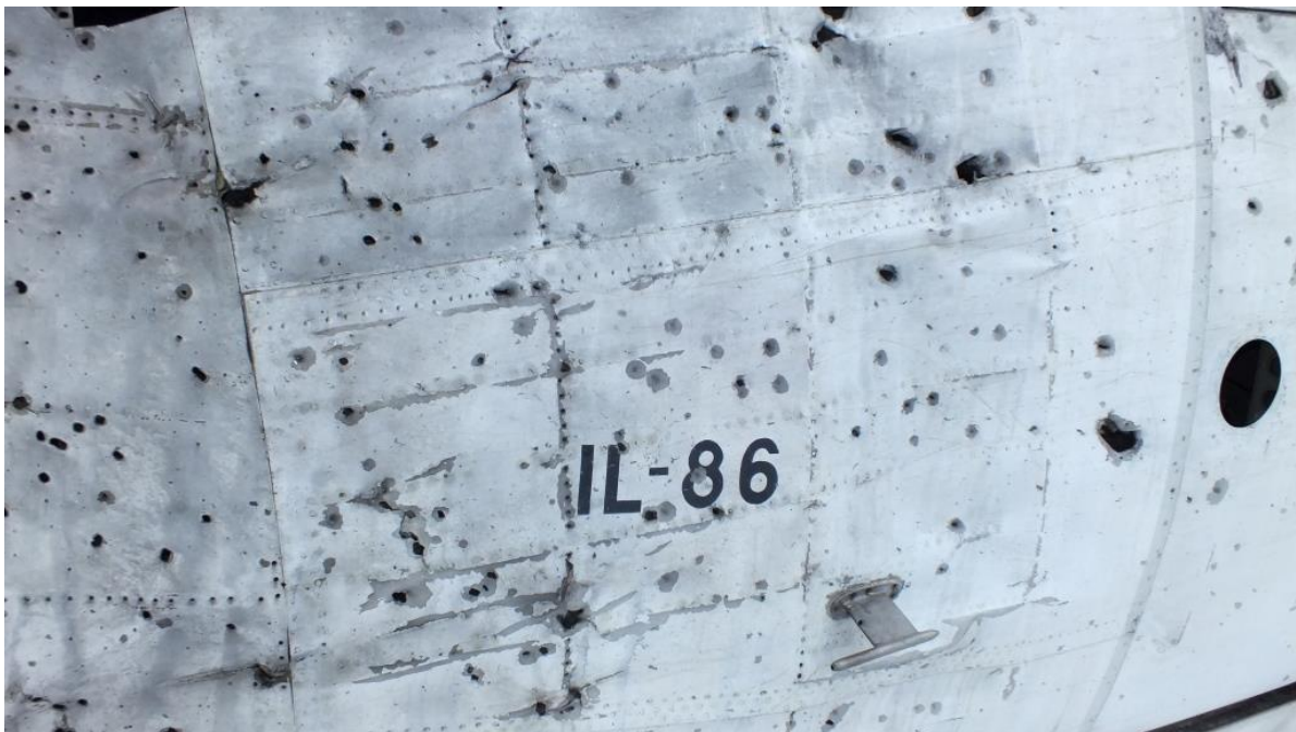
Figure 5.36 - Port side skin (overall view). The fragment shows detachment of the outer skin from the framework resulting from the detachment of rivet heads
