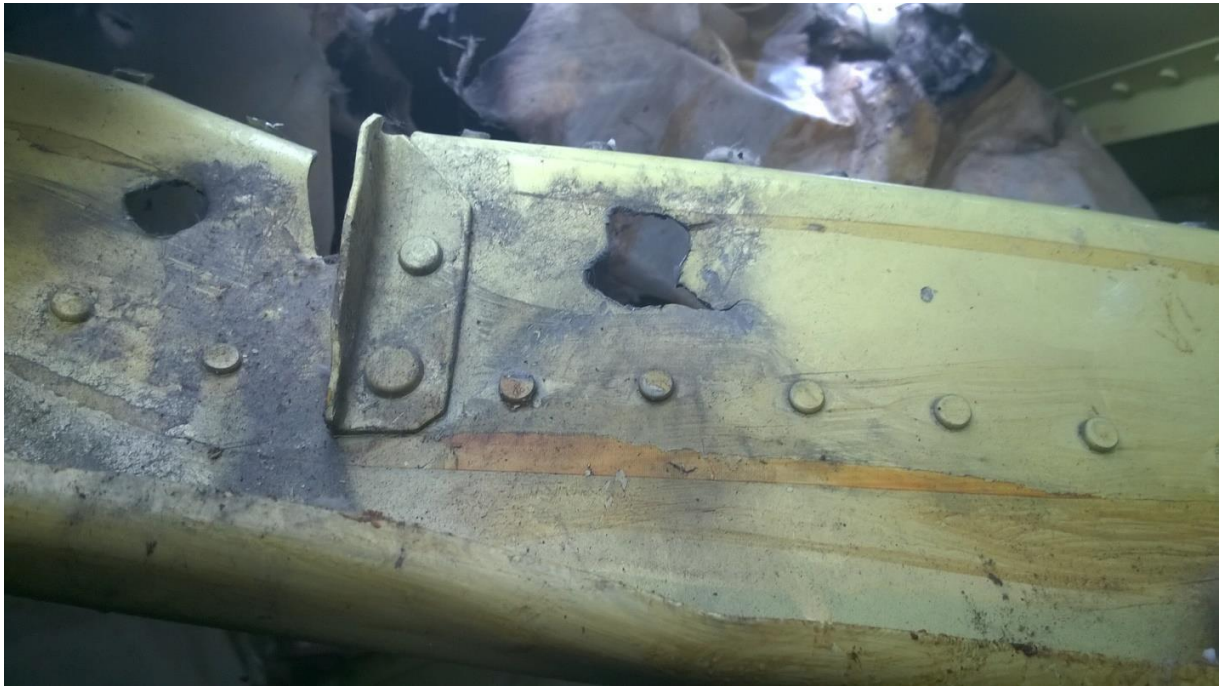
Figure 5.144 - Through-and-through holes in a power kit element
