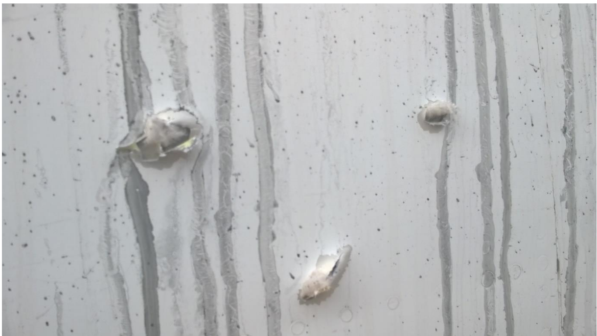
Figure 7.7 - Exit holes on the starboard side
