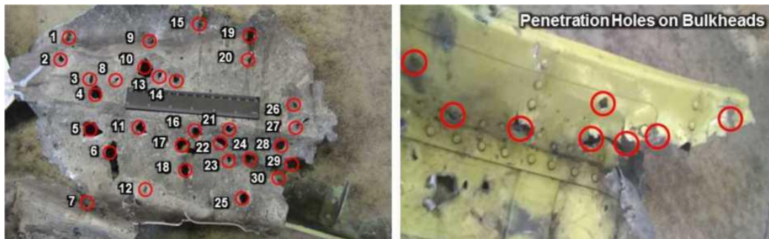
Figure A.3.3 - Fragment of the port side skin from the top behind the third window of the crew commander. Multiple holes in the bulkhead led to deformation and failure of the force element (photo right), indicating that this fragment was exposed to maximum density (mass and kinetic energy) of the projectiles and factors accompanying a close explosion
