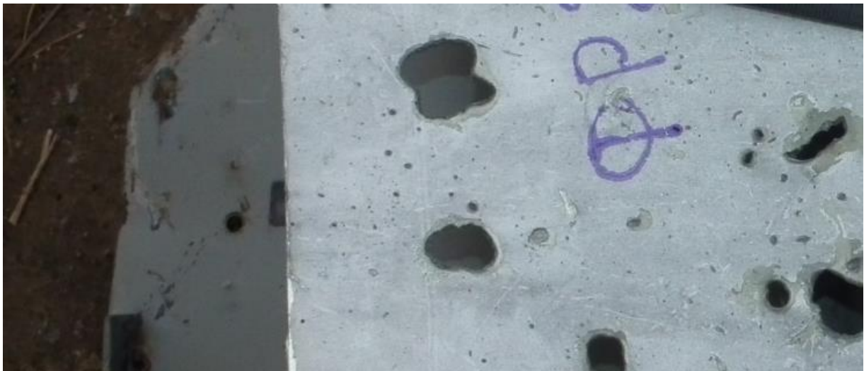
Figure 6.7 - Appearance of a characteristic butterfly-shaped hole in a fragment of the cockpit roof (external view)
