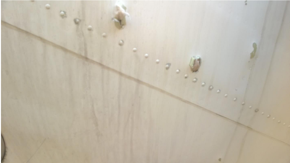
Figure 5.87 - Exit holes and non-penetrating damage
