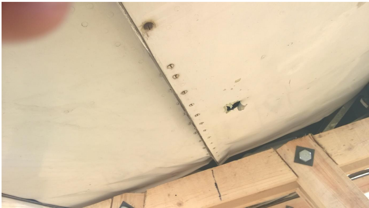
Figure 5.89 - Exit holes and non-penetrating damage
