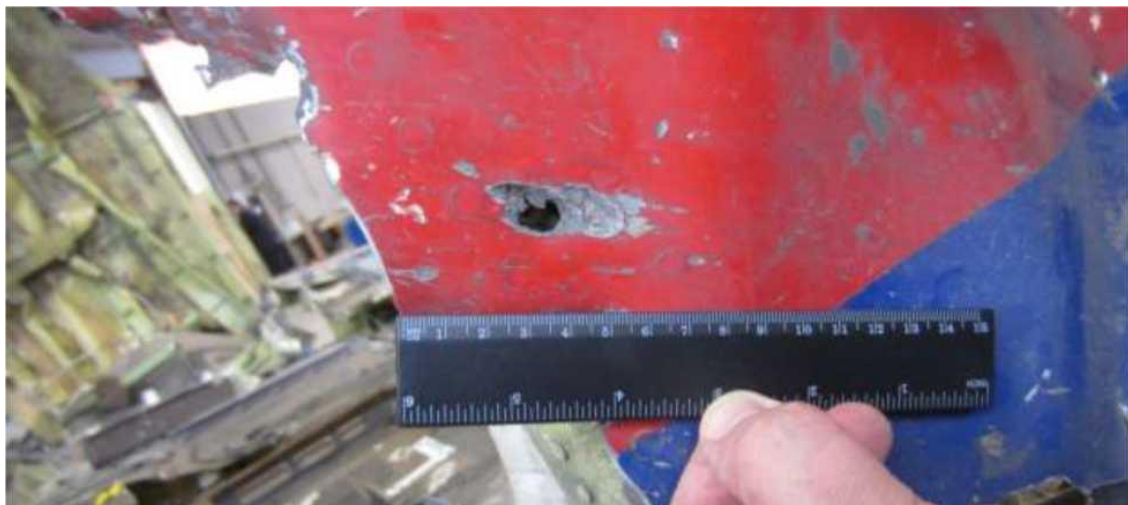
Figure A.2.2 - Exterior view of non-penetrating damage to the port side of the Voinp-777: the damage is under the cockpit glazing
