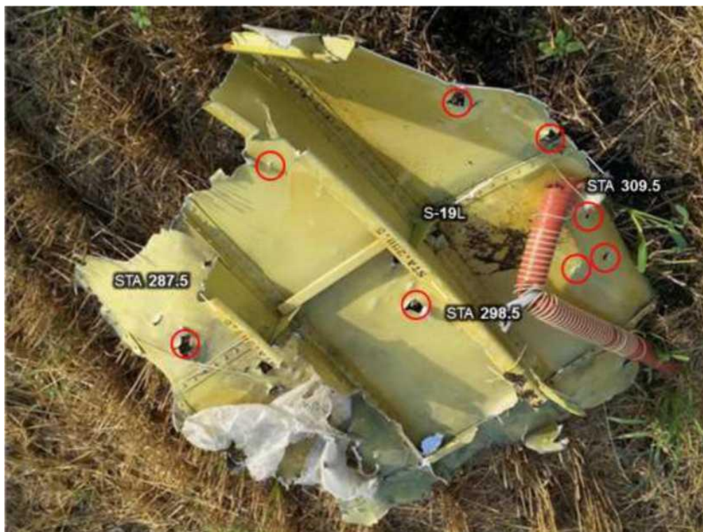
Figure 5.1.24 - Fragment of the central part of the port side behind the cockpit. Figure shows examples of through-and-through and part-through damage between the STA 287.5 and STA 309.5 bulkheads
