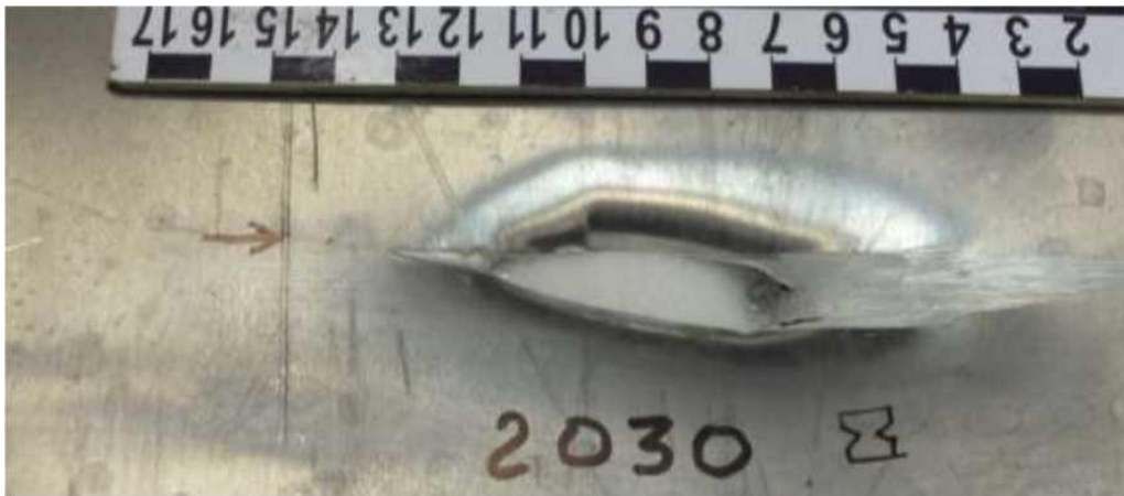
Figure B.4.13 - Experiment 2030. Exterior view of obstacle (Exterior view) after interaction with element no. 1 (9H314M 1-10) at an angle of 5^\circ to the firing line at 1640 m/s
