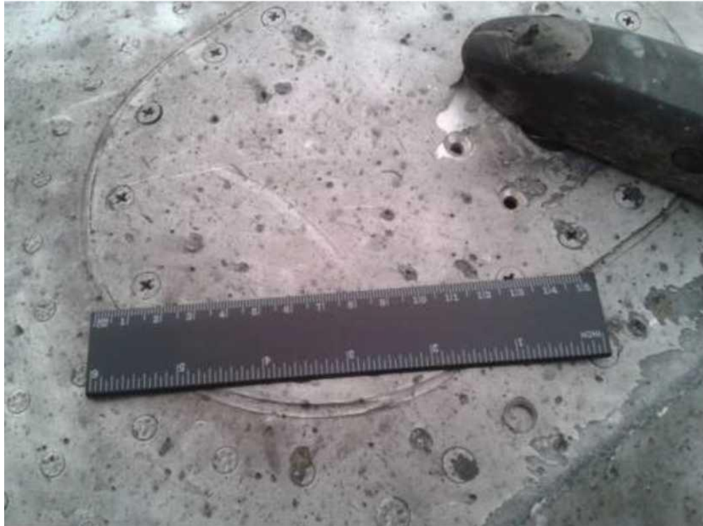
Figure 5.2.35 - Most of the fragment shows only clearly visible traces of close blast products: microcratification, thermal oxidation and soot (photograph February 2015)
