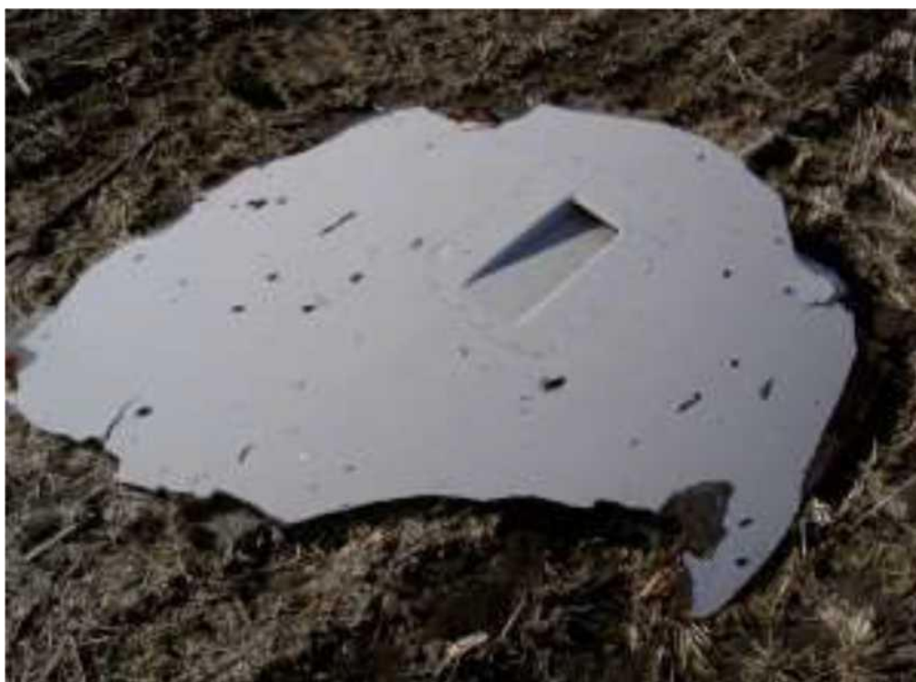
Figure 5.1.59 - Fragment of composite body of left engine nacelle (presumably) with traces of fragmentation damage
