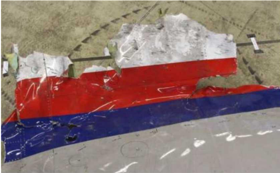
Figure F.3 - Fragment of the underside of the port side with fragmentation damage at the edge of the covering field
