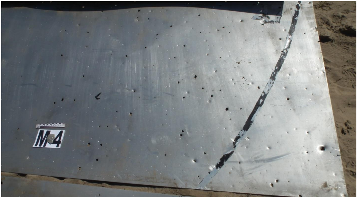
Figure A.141 - Right side of fragment 4.7 of target No. 4
