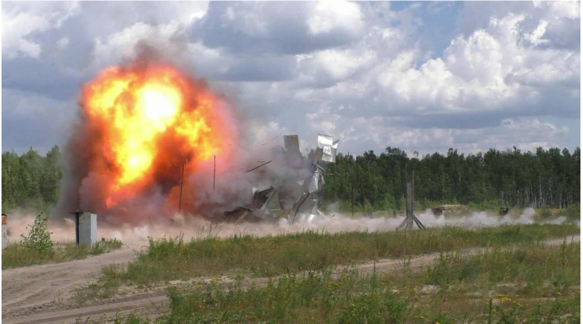
Figure A.27 - Camera No. 4P. The target layout destruction by high-explosive effect
