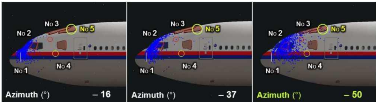
Figure 5.2.18 - Comparison of left side damage modelling results of Boeing 777 for three values of crossing angle
