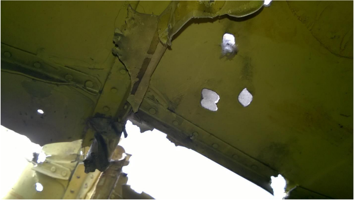
Figure 5.68 - Characteristic butterfly-shaped through-and-through holes in a fragment of the cockpit roof
