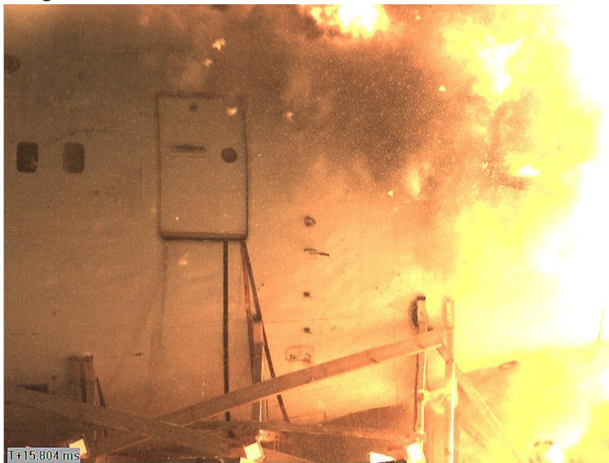
Figure 4.29 - Detonation of the 9H314M warhead
