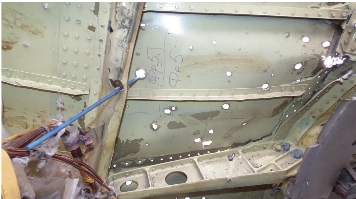
Figure 5.169 - Fragment No. 5 before extraction (internal view). The blue bar shows the trajectory of entry of a projectile of 9H413M 1-10, which, after piercing the outer skin, penetrated the L-shaped reinforcement of a frame
