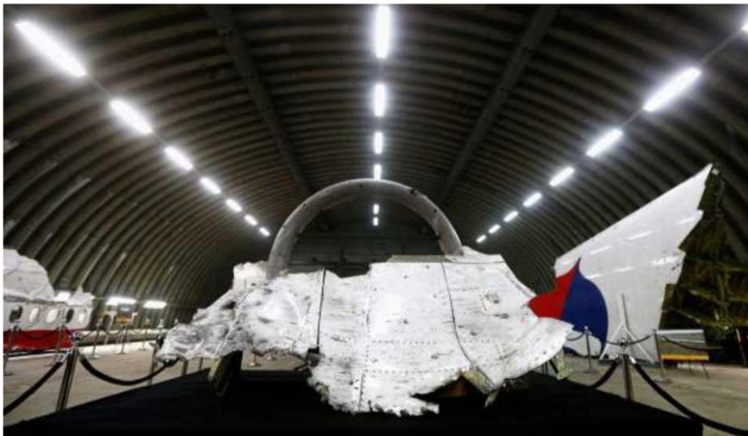
Figure A.1.13 - Exterior view of upper port side and roof fragment behind the cockpit (fragment "F.7")
