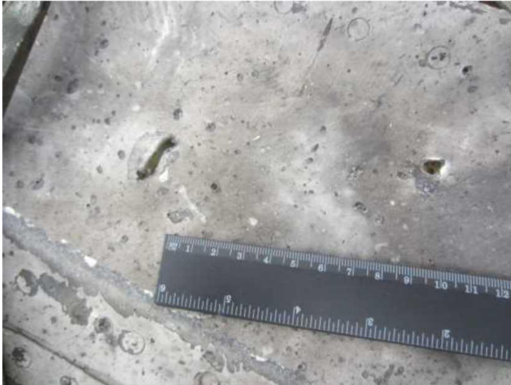
Figure 5.1.9 - There are four through-and-through holes in the fragment. It is most likely that these through-and-through holes are the result of impact of secondary fragments rather than prefabricated projectiles, as evidenced by the shape, appearance and linear dimensions of the holes (photo of May 2015)
