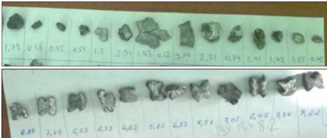
Figure 5.2.8 - Comparative linear dimensions and mass of hull fragments (top) and preformed fragments (bottom)
