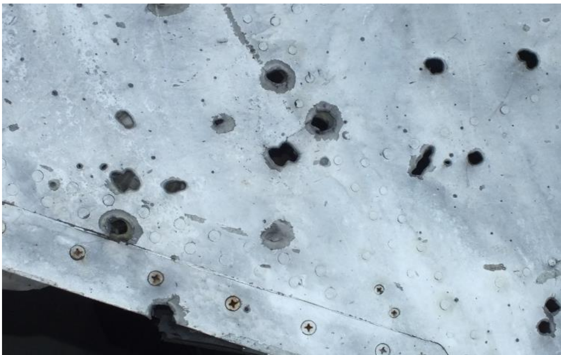
Figure 6.16 - Fragment of the outer skin above the aircraft commander's window
