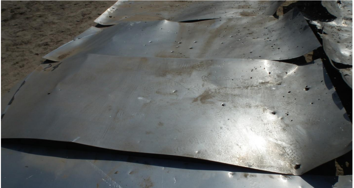
Figure A.77 - Fragments 2.0 (top), 2.2, 2.4 and 2.6 (bottom) of target No. 2
