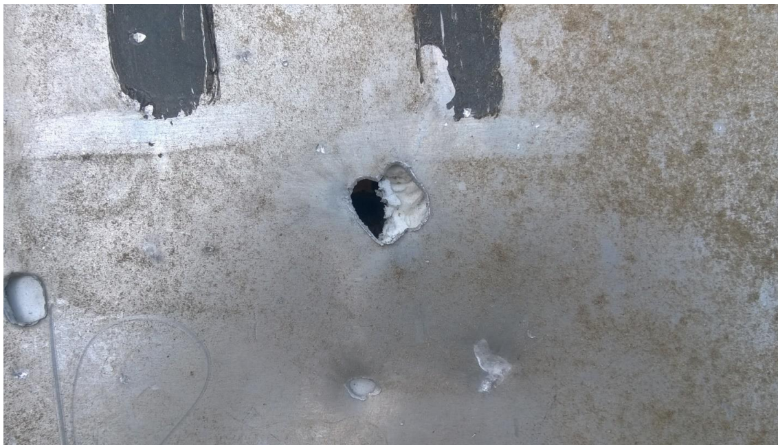
Figure A.33 - Example of a "butterfly"-shaped hole in the first barrier of trap L1 after the testing
