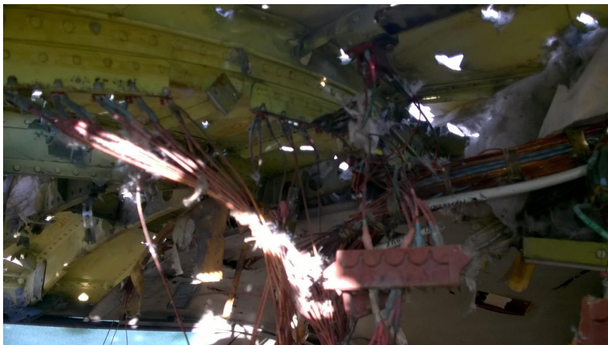
Figure 5.70 - Through-and-through holes on the right side of the cockpit roof (inside view)
