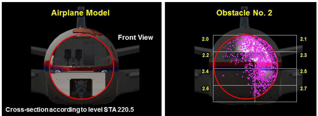
Figure 5.2.33 - Distribution of target coverage density combined with Boeing 777 contour across the STA 220.5 level cross section
