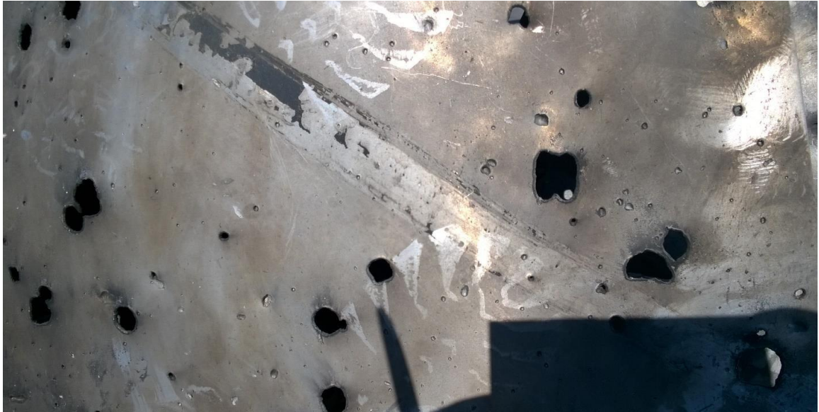
Figure A.180 - Target fragment with micro-crater marks and thermal oxidation
