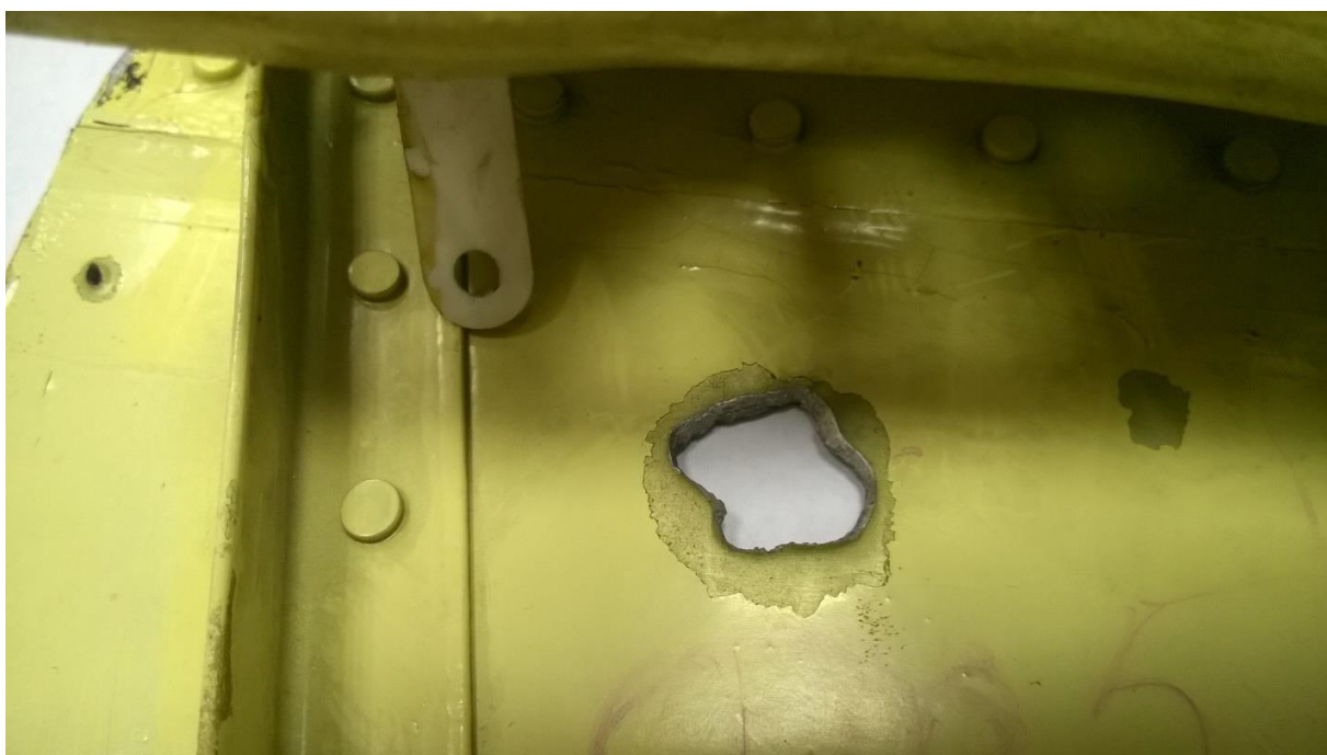
Figure 6.17 - Characteristic butterfly-shaped hole in the outer skin of the port hull caused by a preformed fragment 9H314M 1-10 (inside view)
