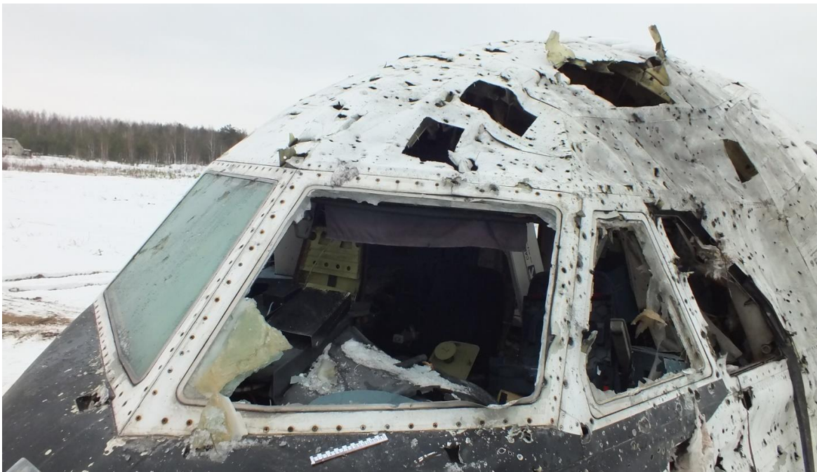
Figure 5.178 - Locations of extracted fragments (external view)
