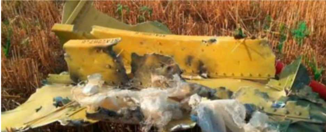
Figure A.3.4 - Fragment of the centre port side behind the cockpit. Objectively observed holes in the STA 287.5 and STA 298.5 bulkheads, traces of compression, deformation, rupture and destruction of structural members
