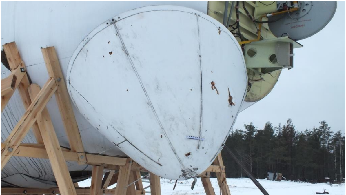
Figure 5.13 - Output holes in the radiotransparent radome
