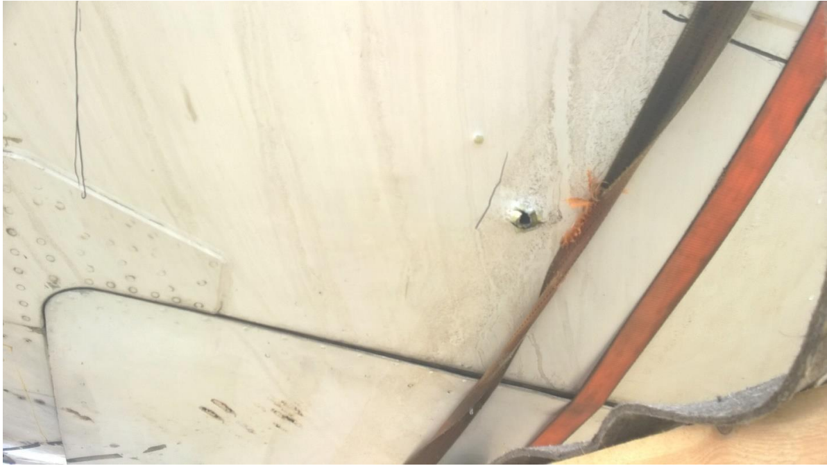
Figure 5.103 - Exit holes and non-penetrating damage
