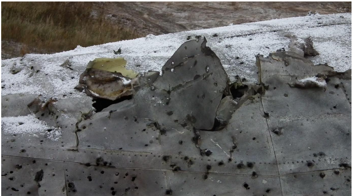
Figure 5.62 - Left side of cockpit roof before removal of fragments (top left view)
