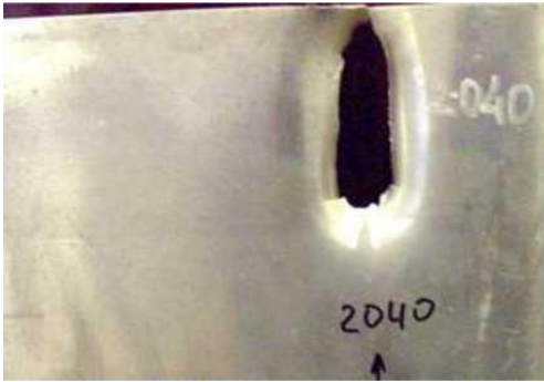
Figure B. 4.12 - Experiment 2040. Exterior view of obstacle after interaction with element no. 1 at an angle of 10^\circ to the firing line at 1688 m/s
