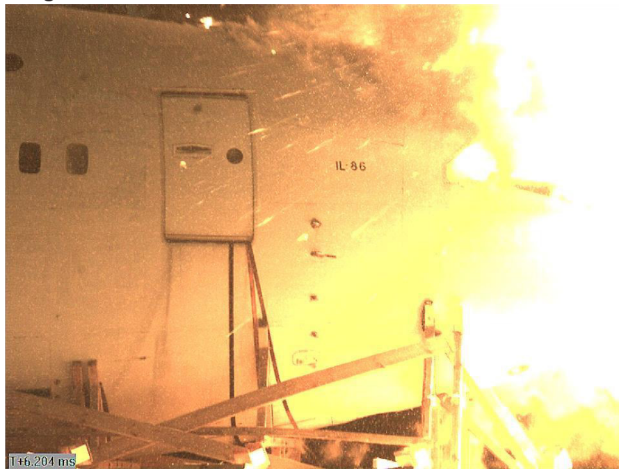
Figure 4.11 - Detonation of the 9H314M warhead
