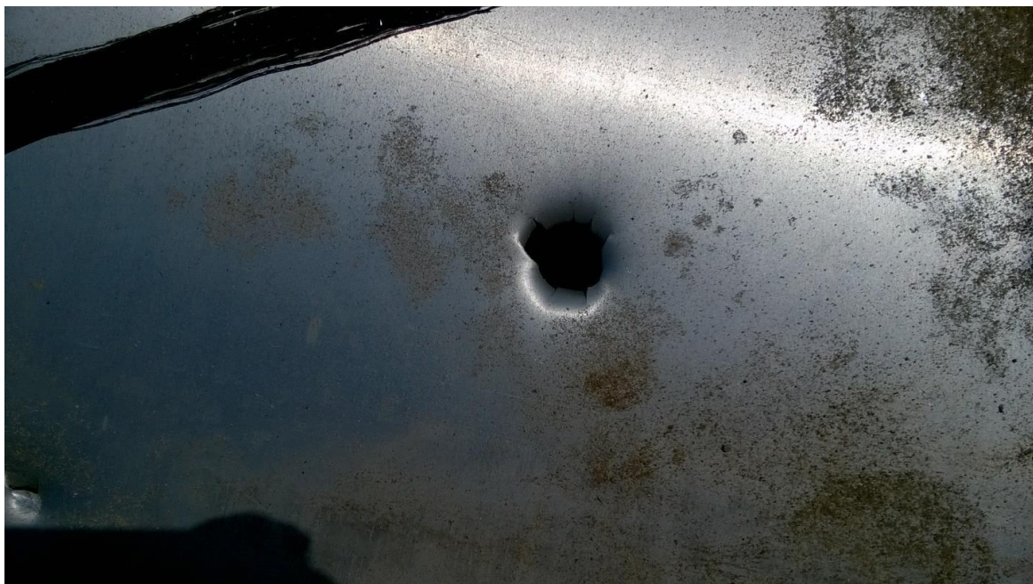
Figure A.175 – Holes left by hull fragments
