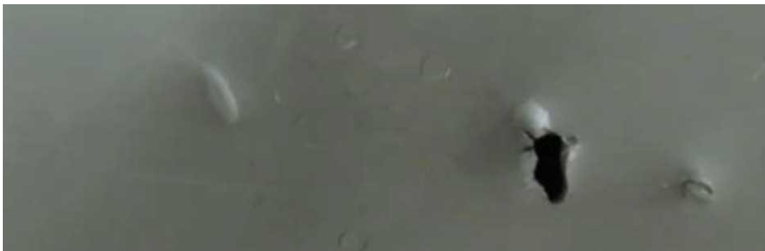
Figure A.4.5 - Close-up of inside-outside exit damage: non-clearance damage (left) and through-hole damage (right)
