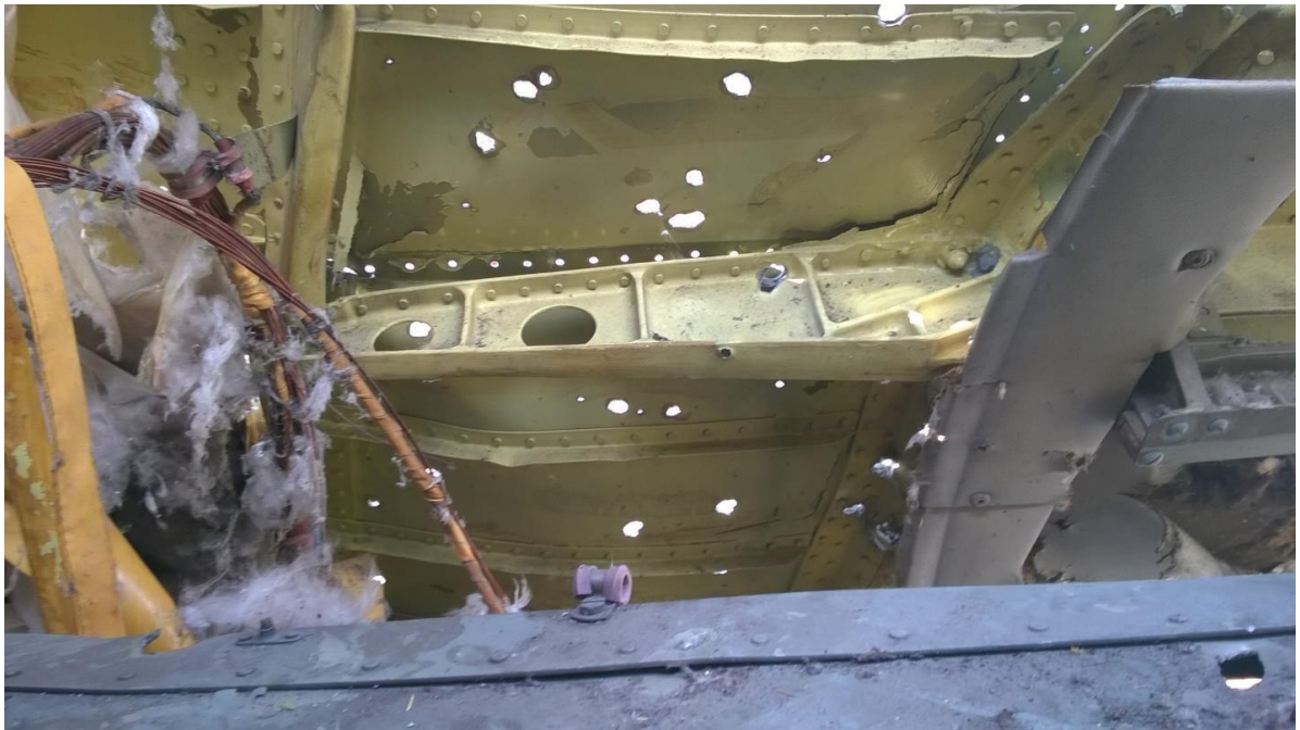
5.51 - Fragment of the port side behind the aircraft commander's seat (overall view, inside view)
