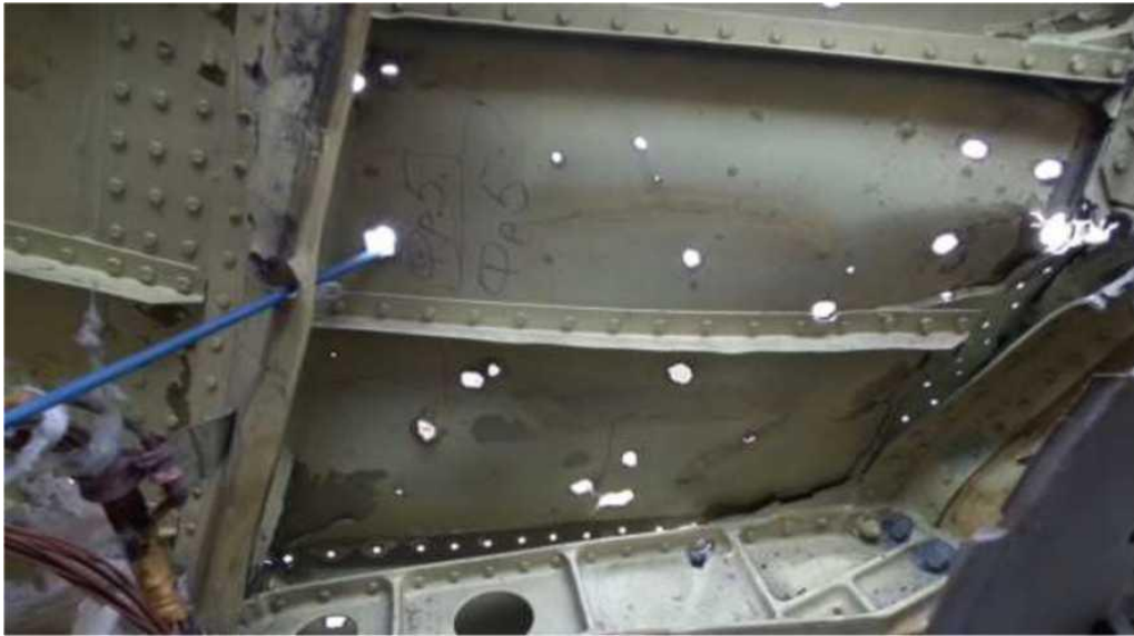
Figure A.4.14 - Direction of motion of the projectiles through the outer skin fragment and the port side bulkhead
