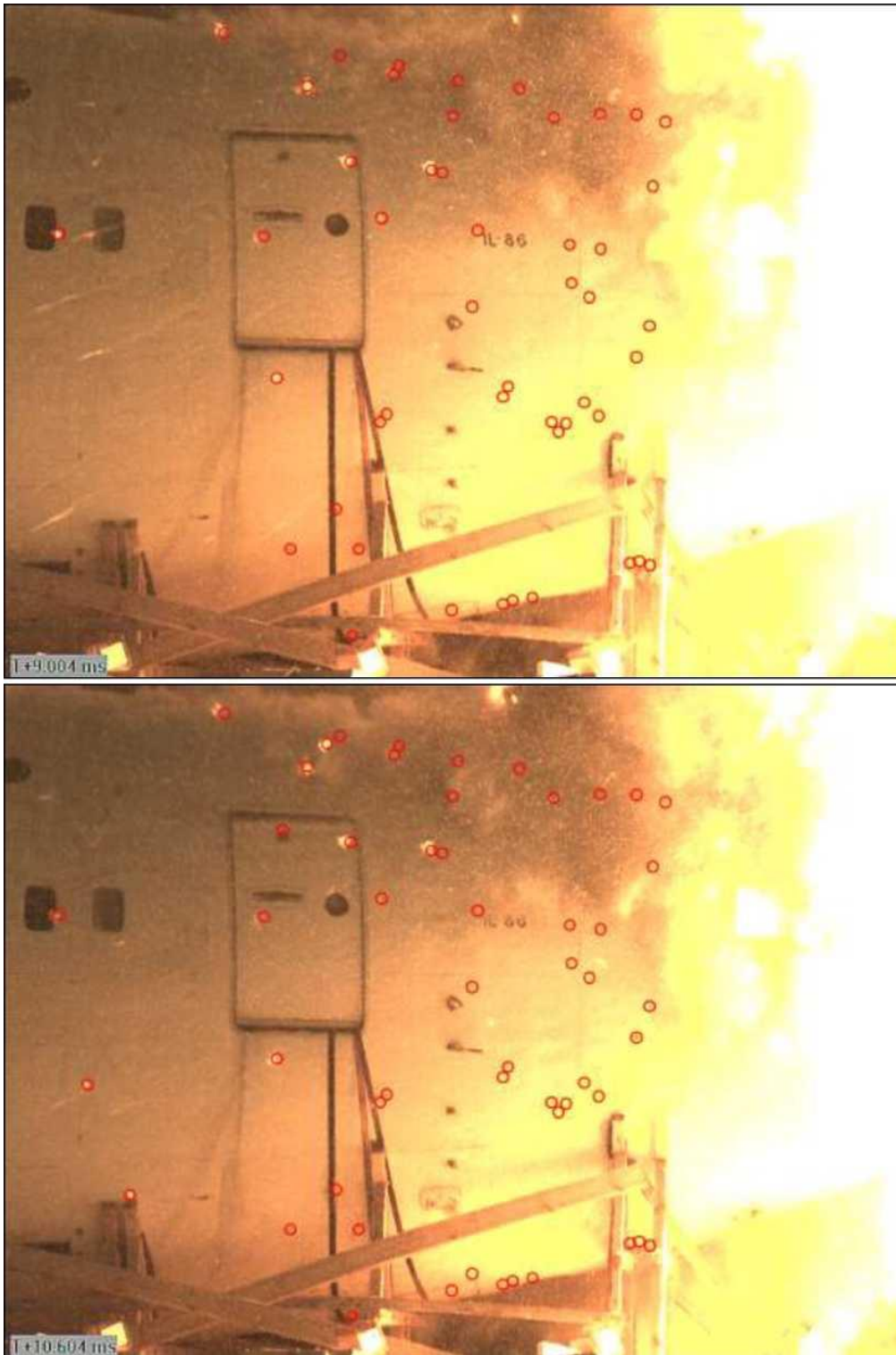
Figure B.3.15 - Puncturing the starboard side of the target aircraft IL-86 (top - T+ 9.004 ms; bottom - T+ 10.604 ms)
