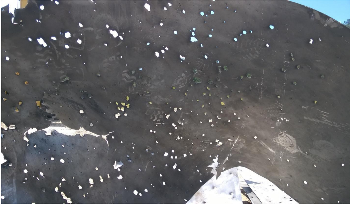
Figure A.186 - Target fragment with traces of deformation and rupture of skin sheets
