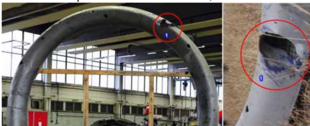
Figure 5.1.55 - Example of secondary damage to the left engine air intake edge
