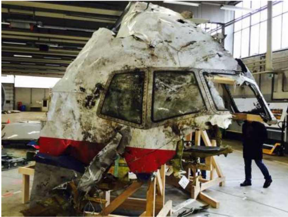
Figure 5.1.16 - Fragment of the right-hand side of the cockpit with part of the roof and preserved transparency on the right-hand side
