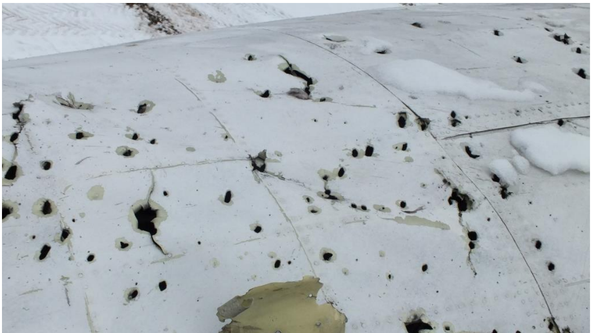
Figure 5.65 - Cockpit roof near the centre (axial) line of the aircraft. The fragment shows traces of damage caused by ready-made projectiles to both the left and right sides of the roof
