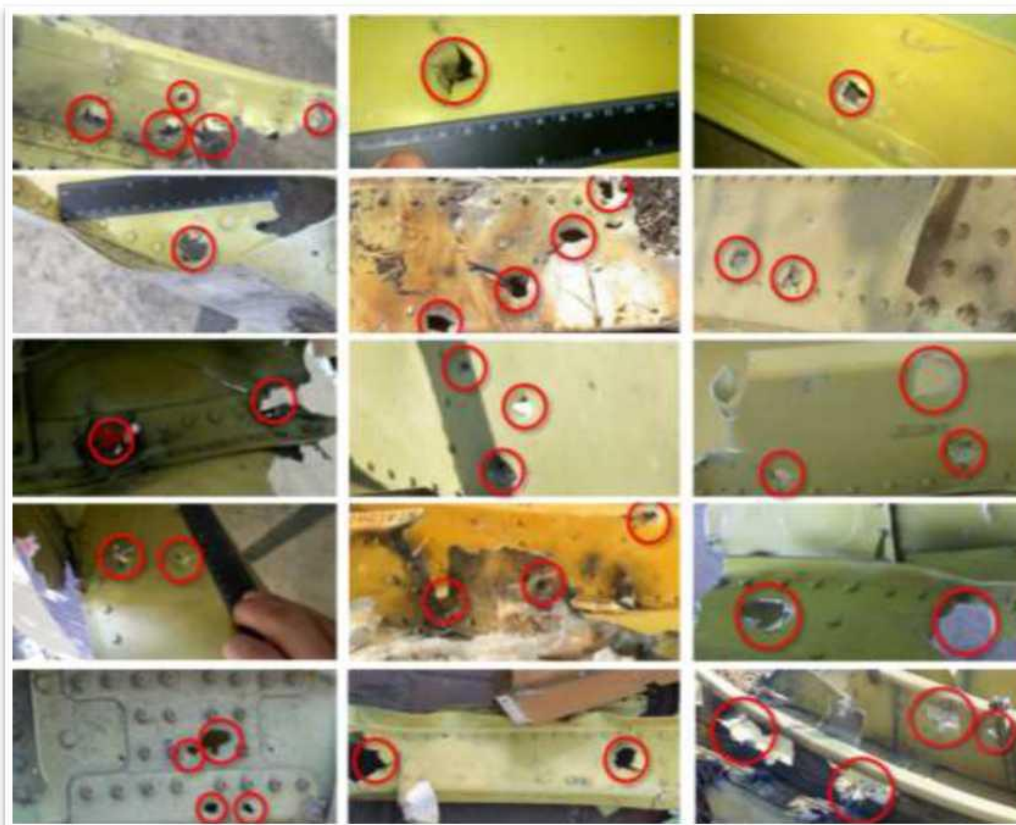
Figure 5.1.37 - Examples of damage to bulkheads
