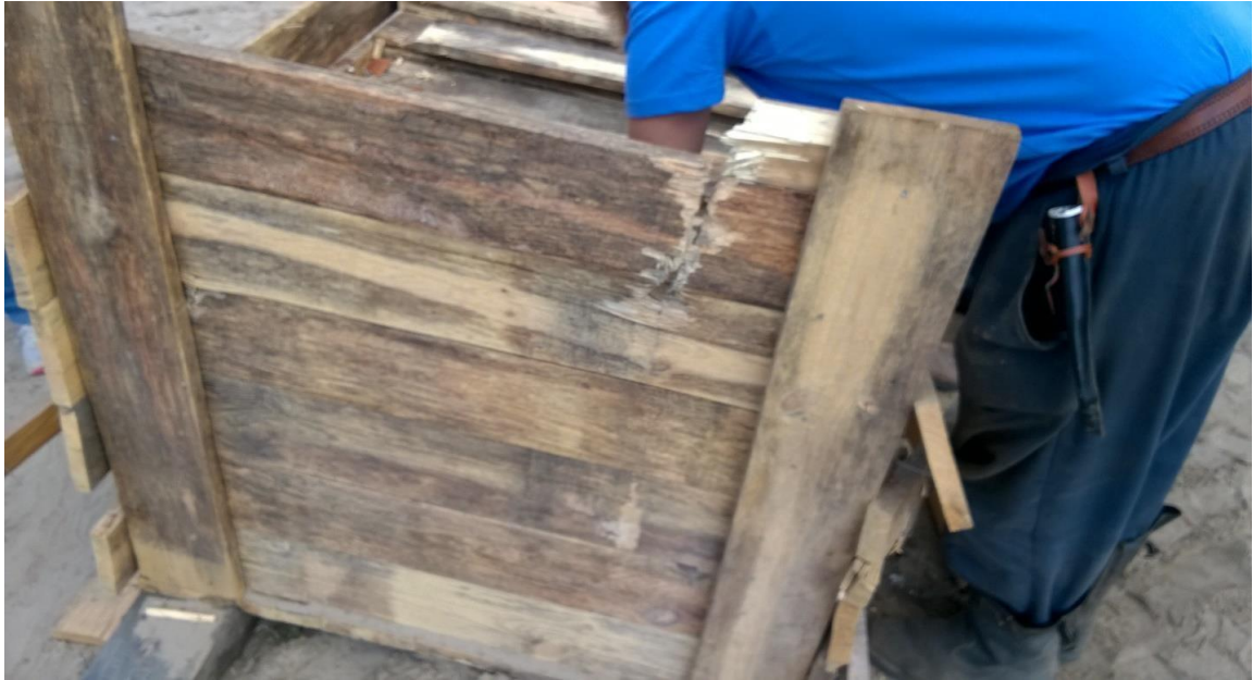
Figure A.43 - Disassembling trap L1 to remove fragments
