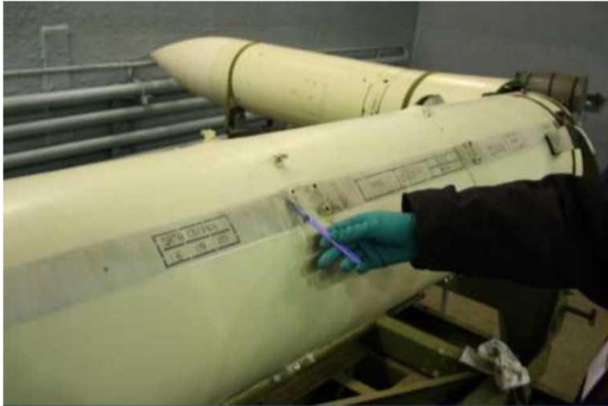
Figure E.3 - Stamp "ASSEMBLY DATE" on the 9M38 missile delivered by Ukraine to the investigation. The expert shows with his hand the attachment point of the wing on the shell of the third compartment. In order to see the stamp "Assembly date", the wing must be dismantled (resource - materials of KNIISE)
