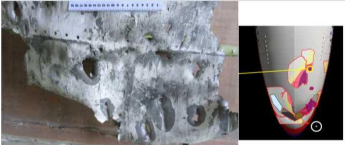
Figure 5.1.34 - Fragment of roof and upper port side (not included in final 3D reconstruction)
