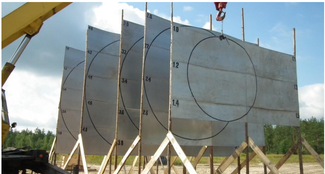
Figure A.5 - Target layout imitating the contours of the nose of a Boeing 777-200 aircraft
