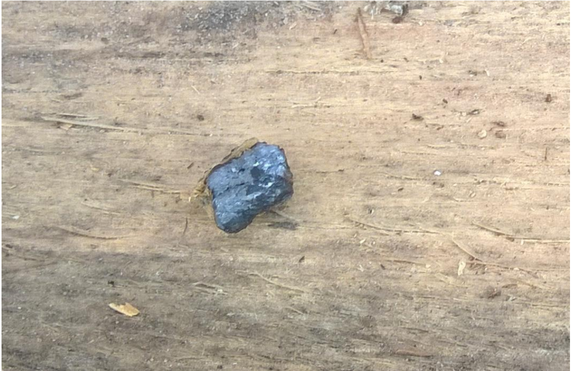
Figure A.205 - 9H314M 1-9 projectile ("parallelepiped")
