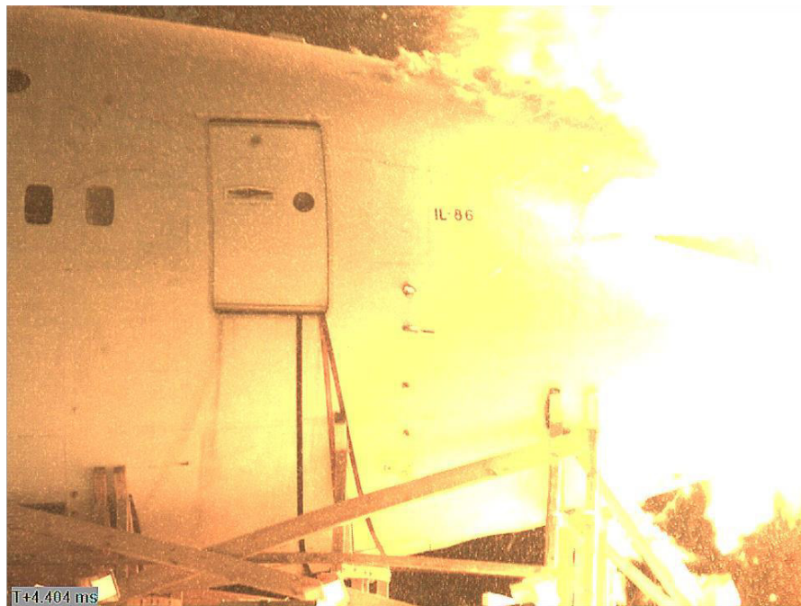
Figure 4.7 - Detonation of the 9H314M warhead
