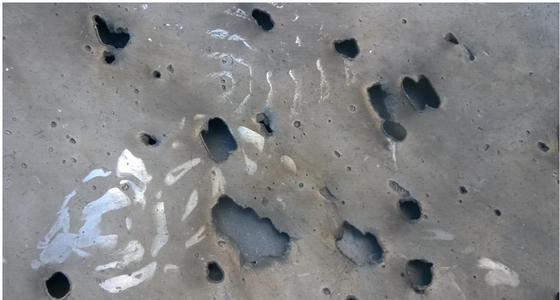
Figure A.181 - Target fragment with micro-crater marks and thermal oxidation
