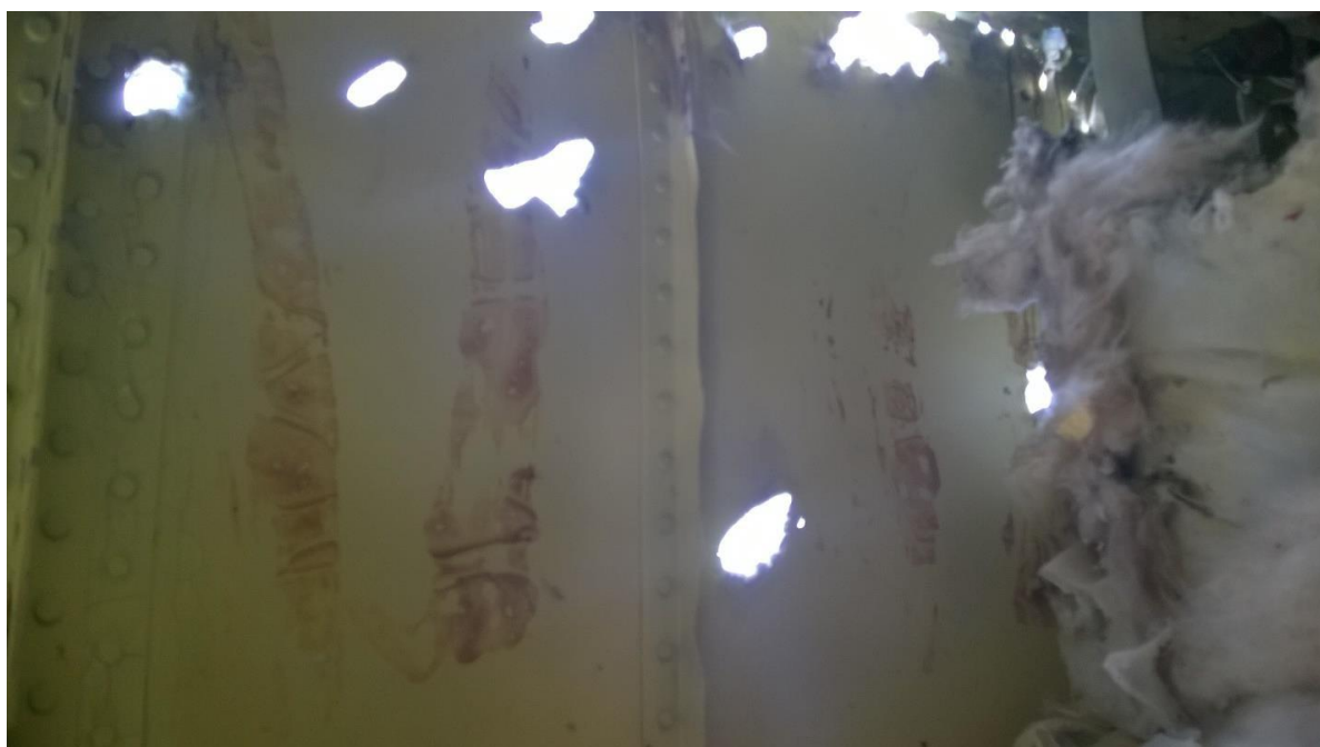
Figure 5.70 - Through-and-through holes on the right side of the cockpit roof (inside view)
