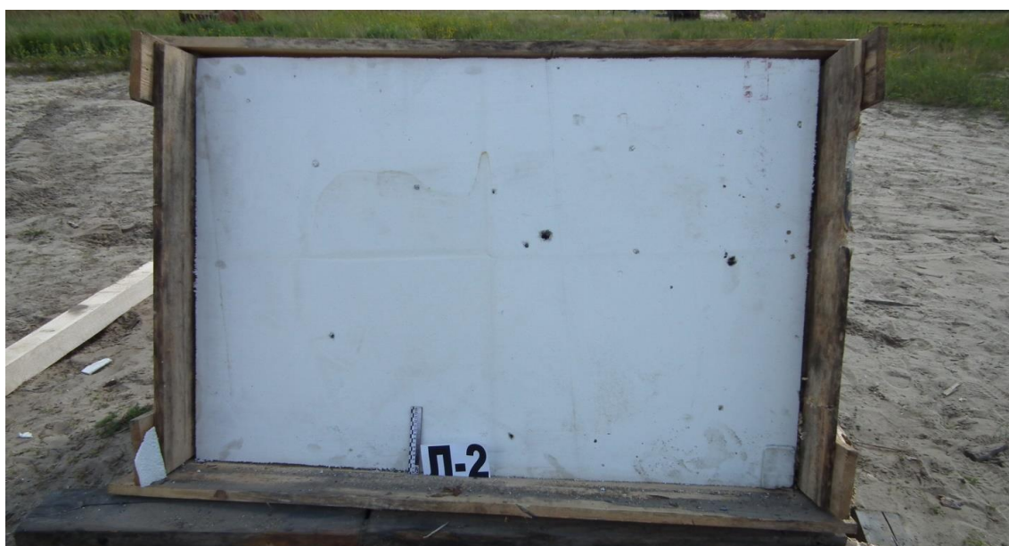
Figure A.41 - Second barrier of trap L2 (second layer of foam plastic PS-1-150) after the testing
