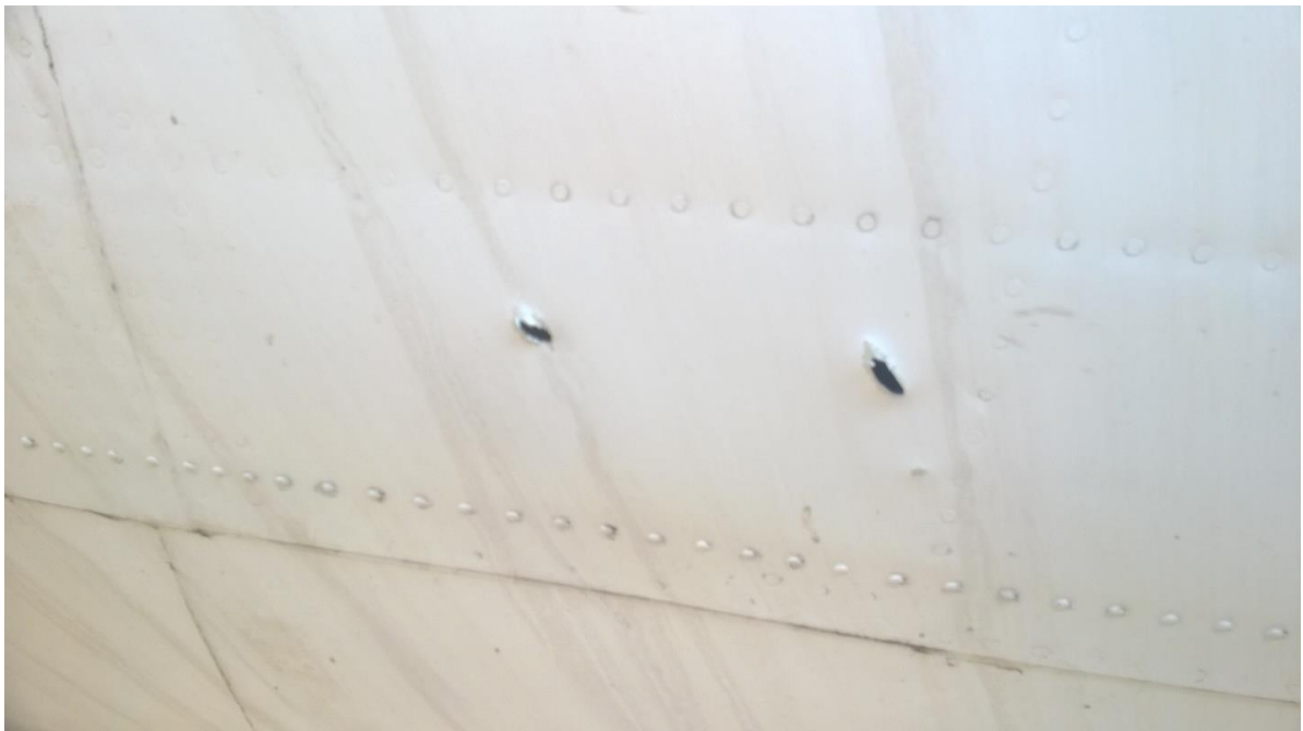
Figure 5.100 - Exit holes and non-penetrating damage
