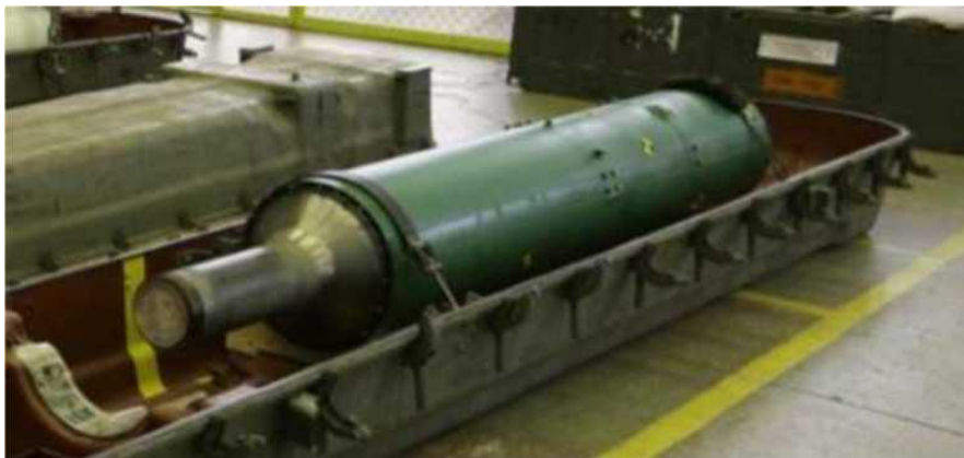
Figure E.4 - 9M38M1 missile engine provided by Ukraine to the investigation (resource - materials of KRISE)
