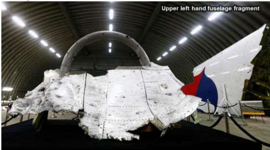
Figure 5.1.4 - Fragment of the top of the port side (front) and the nose of the left engine air intake (rear) were located elsewhere in the final reconstruction (open-source photo)
