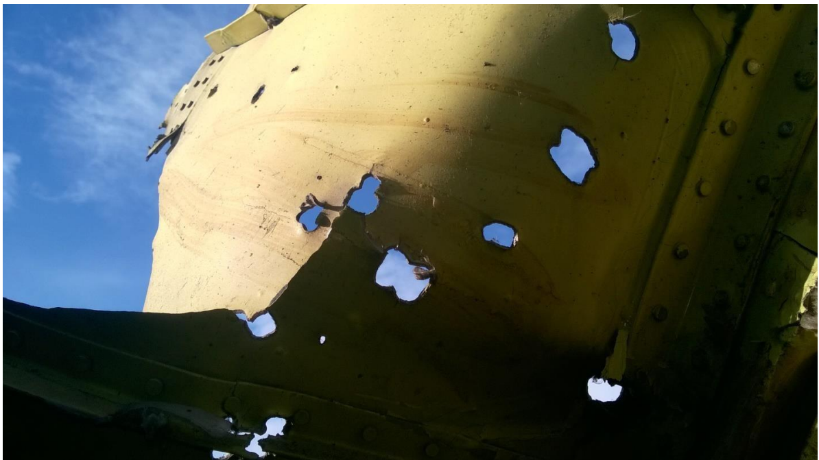
Figure 5.48 - Fragment of upper part of the port with characteristic butterfly-shaped holes caused by 9H314M 1-10 ready-made projectiles (inside view)
