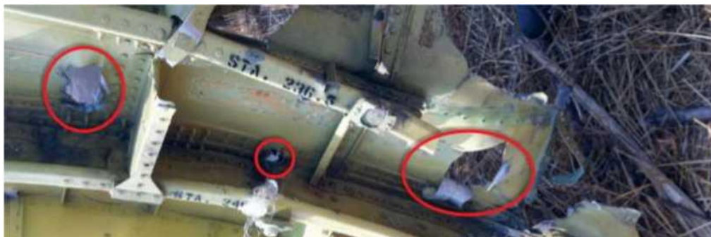
Figure 5.1.21 - Factory markings on the front bulkhead STA 236.5 and the bulkhead STA 246 which is behind it (rear cockpit wall) can be seen
