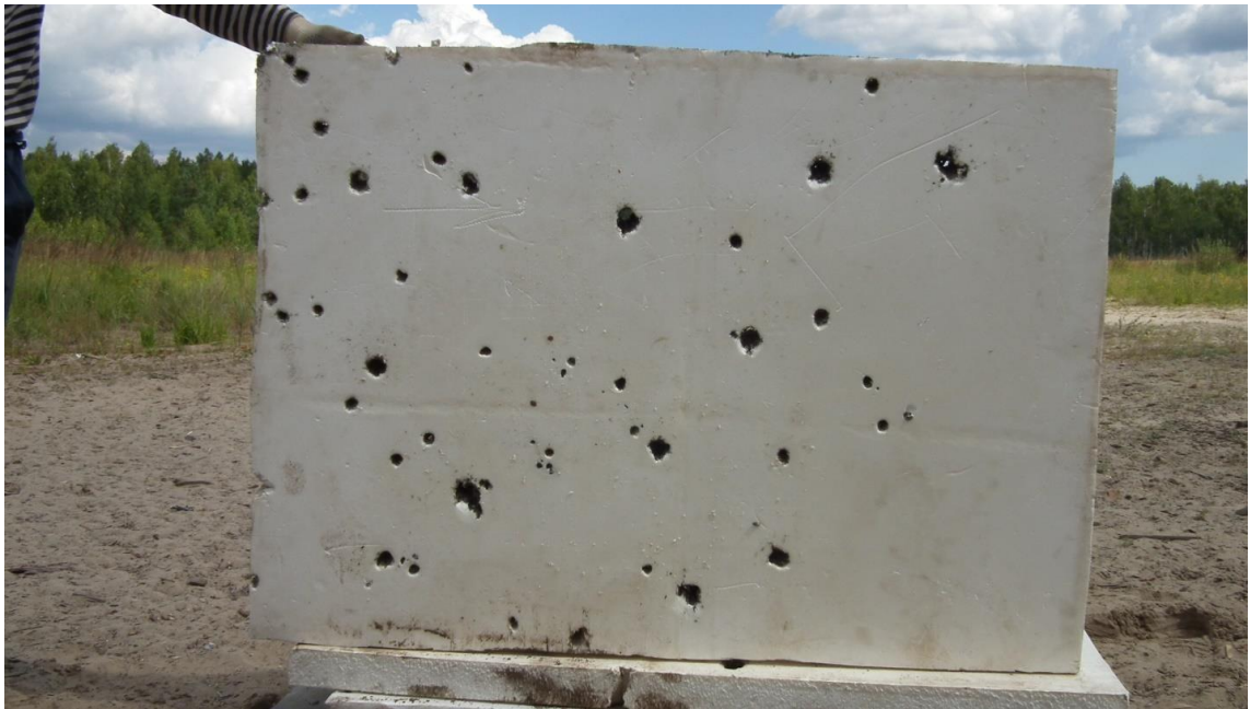
Figure A.36 - Second barrier of trap L1 (third layer of foam plastic PS-1-150) after the testing
