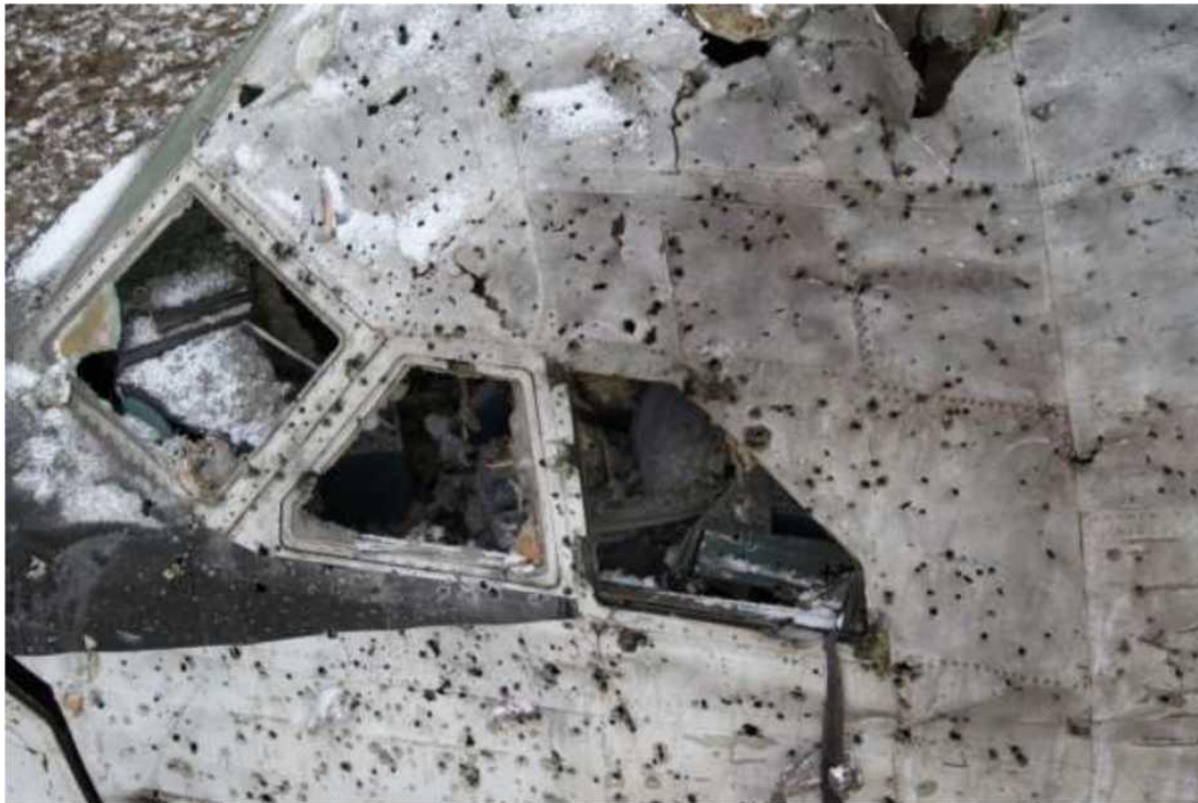
Figure B.3.18 - No non-penetrating damage (ricochets) from preformed fragments on the port side of target aircraft b-86
