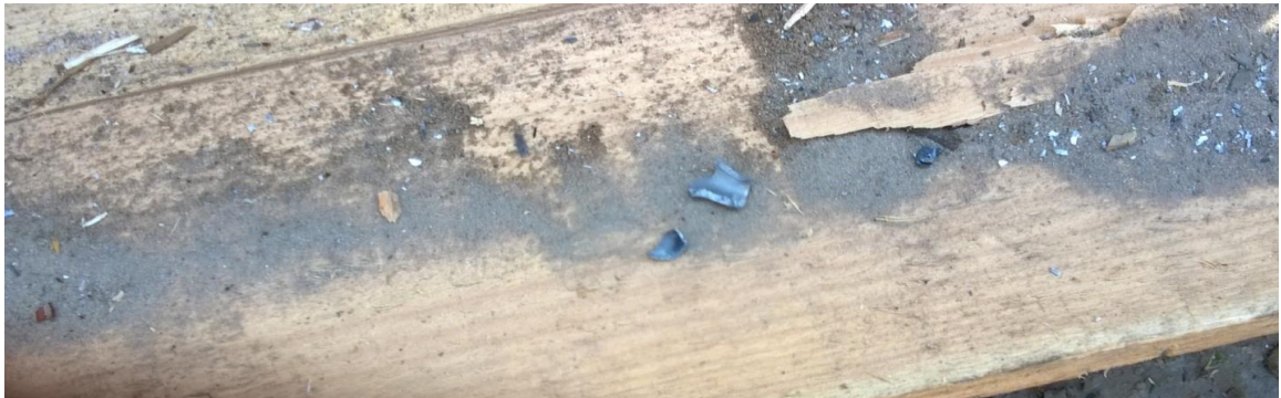
Figure A.192 - Secondary striking elements ("plugs" from target sheets)
