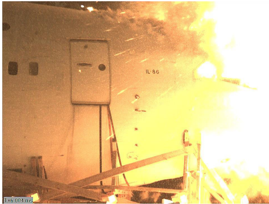
Figure 4.11 - Detonation of the 9H314M warhead
