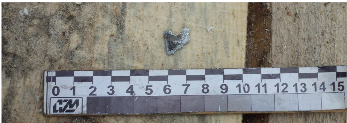
Figure A.194 - Secondary striking element ("plug") shaped like a "bowtie"
