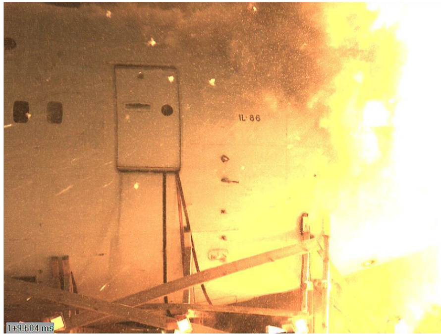
Figure 4.21 - Detonation of the 9H314M warhead
