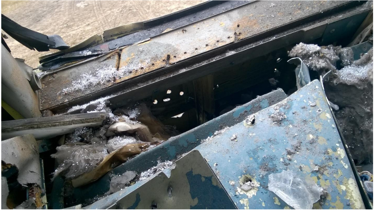
Figure 5.53 - Fragment of the port side in the area of the aircraft commander's direct-vision window
