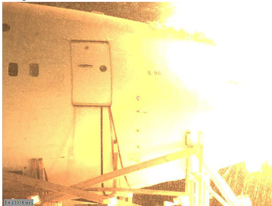
Figure 4.5 - Detonation of the 9H314M warhead
