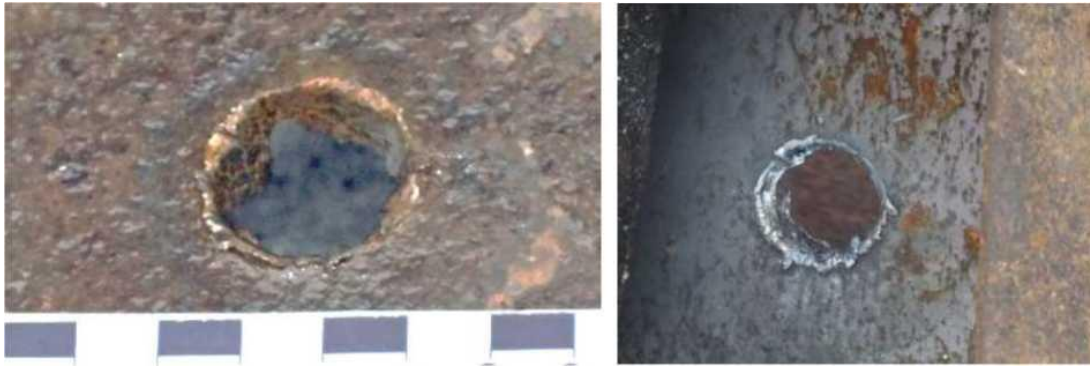
Figure B.4.17 - Exterior view of steel shield (St3 x 5.00 mm) after interaction with projectiles penetrating beyond the barrier (left side is a breach from element 9H314M 1-10 "bowtie")
