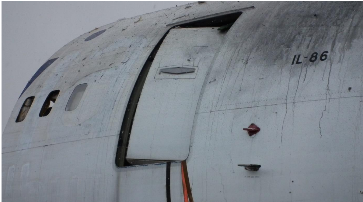
Figure 5.81 - Cockpit starboard side near door R1. Thermal burn marks can be seen in the upper right corner of the photograph
