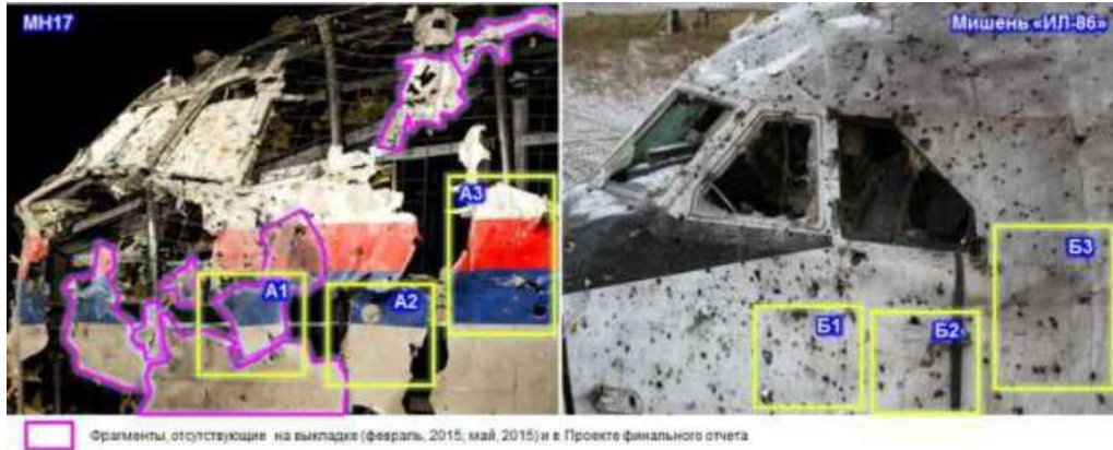
Figure A.4.1 - Fragments of the left side of a Boeing 777 (left) and an IL-86 target aircraft (right)
