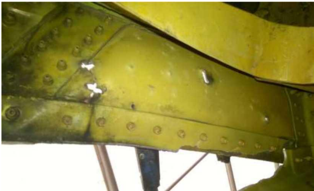
Figure 5.1.10 - Appearance of through-and-through holes. View from the inside of the fragment (photo of May 2015)
