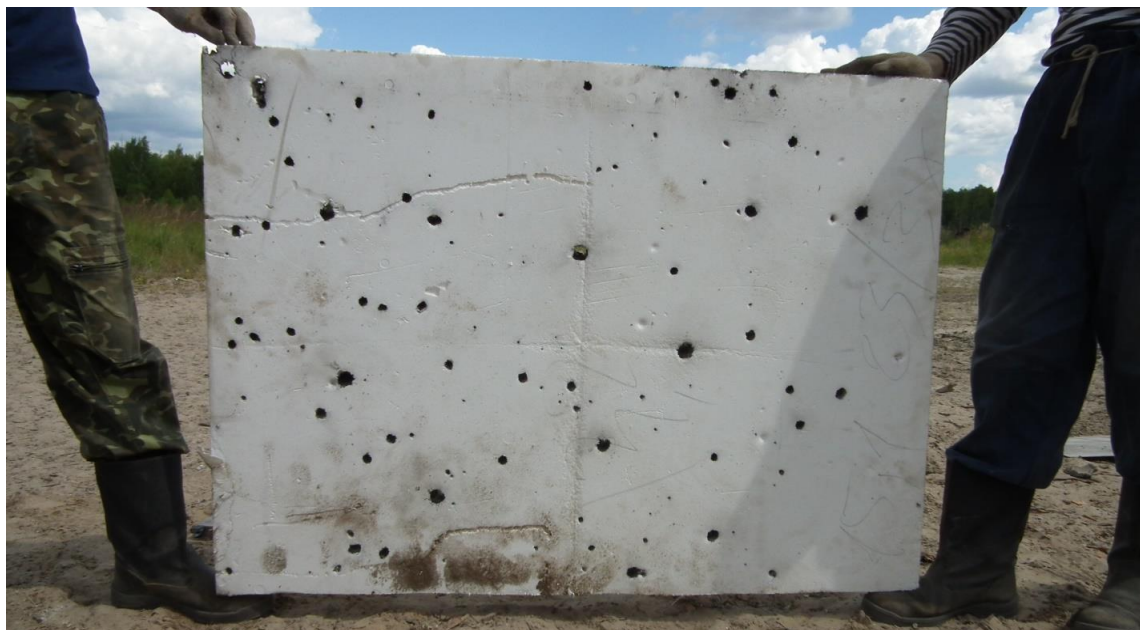
Figure A.33 - Example of a "butterfly"-shaped hole in the first barrier of trap L1 after the testing
