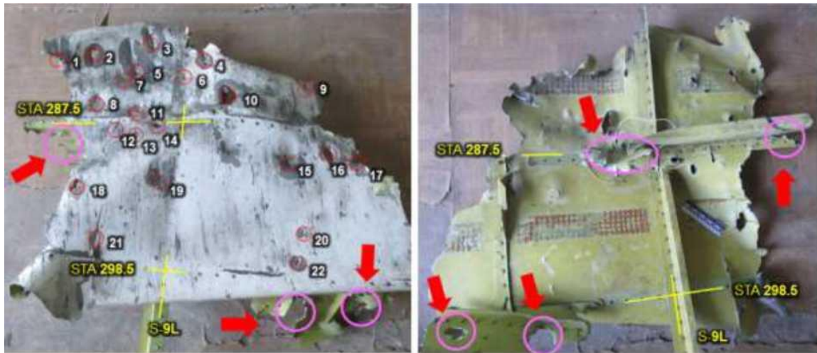
Figure 5.1.40 – Fragment of roof and upper part of the port side: external (left) and internal (right) views. Multiple holes in bulkheads STA 287.5 and STA 298.5 led to deformation and collapse of the structural elements (red arrows indicate characteristic damage)
