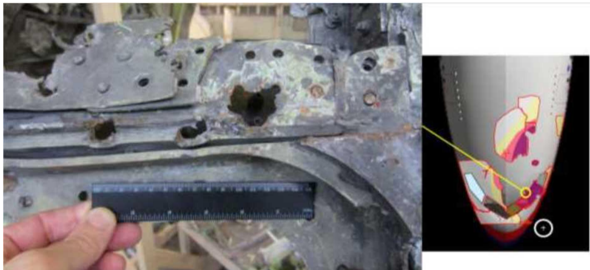
Figure 5.1.30 - Upper part of the frame of the left-hand cockpit window
