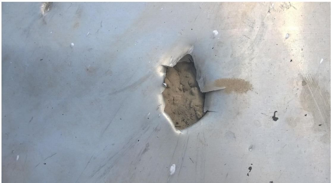
Figure A.177 - Hole left by a hull fragment
