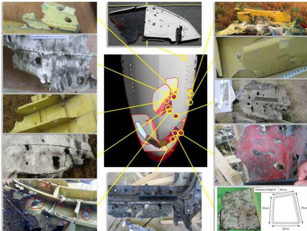
Figure 5.1.35 - Layout of the outer skin and airframe fragments with the highest density of damage and signs of close blast effects
