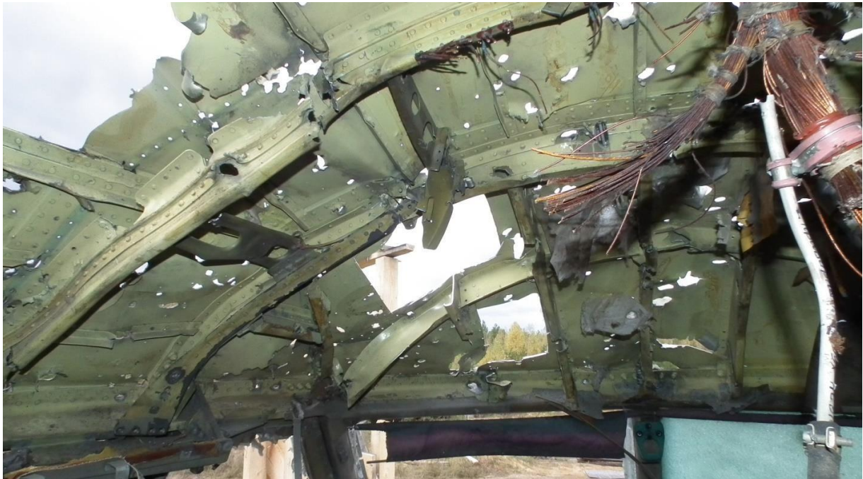
Figure 5.167 - Place of extraction of fragments No. 2 and No. 4 (internal view)
