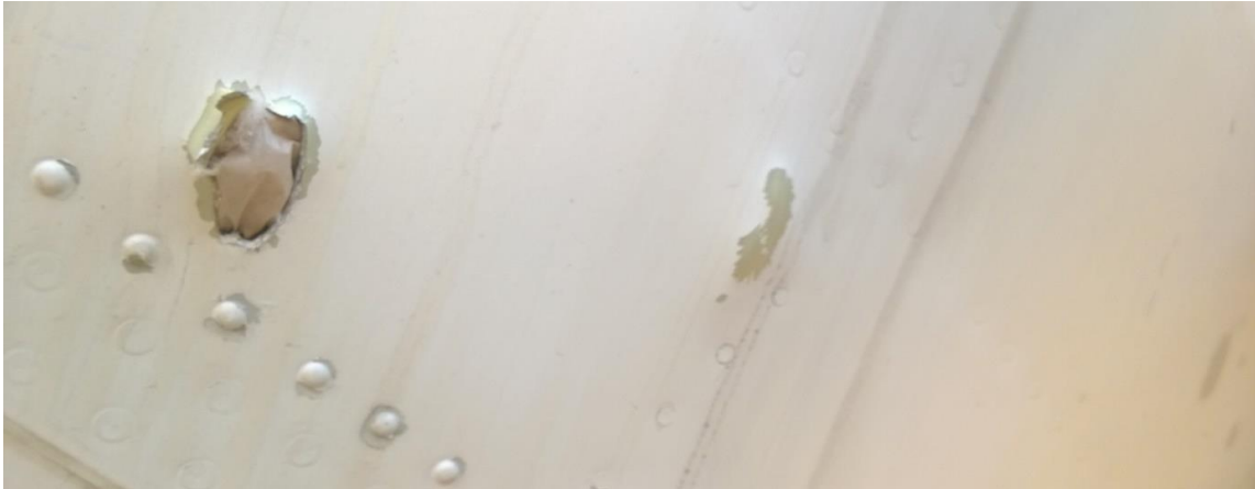
Figure 7.4 - Exit hole (left) and non-penetrating damage (right)
