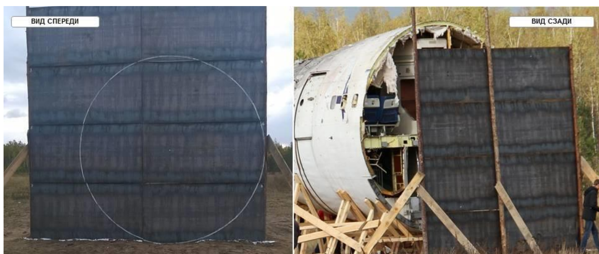
Figure 5.106 - Target No. 2 (left engine) after testing
