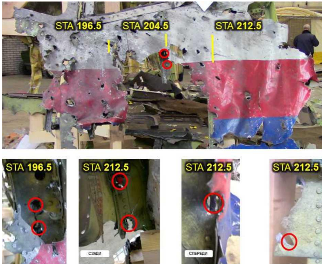
Figure A.3.2 - Punctures in bulkheads STA 196.5 - STA 212.5 under the glazing of the left side of the cockpit
