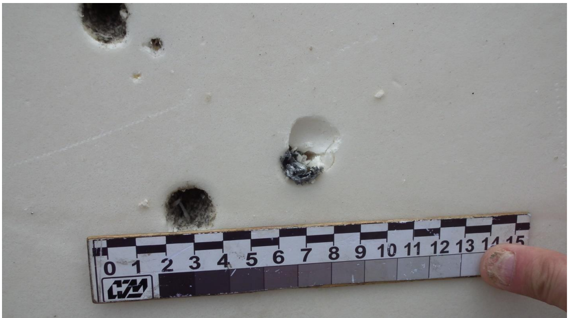
Figure A.37 - Hull fragment (that of the compartment hull) lodged in the third layer of stopping foam plastic PS-1-150
