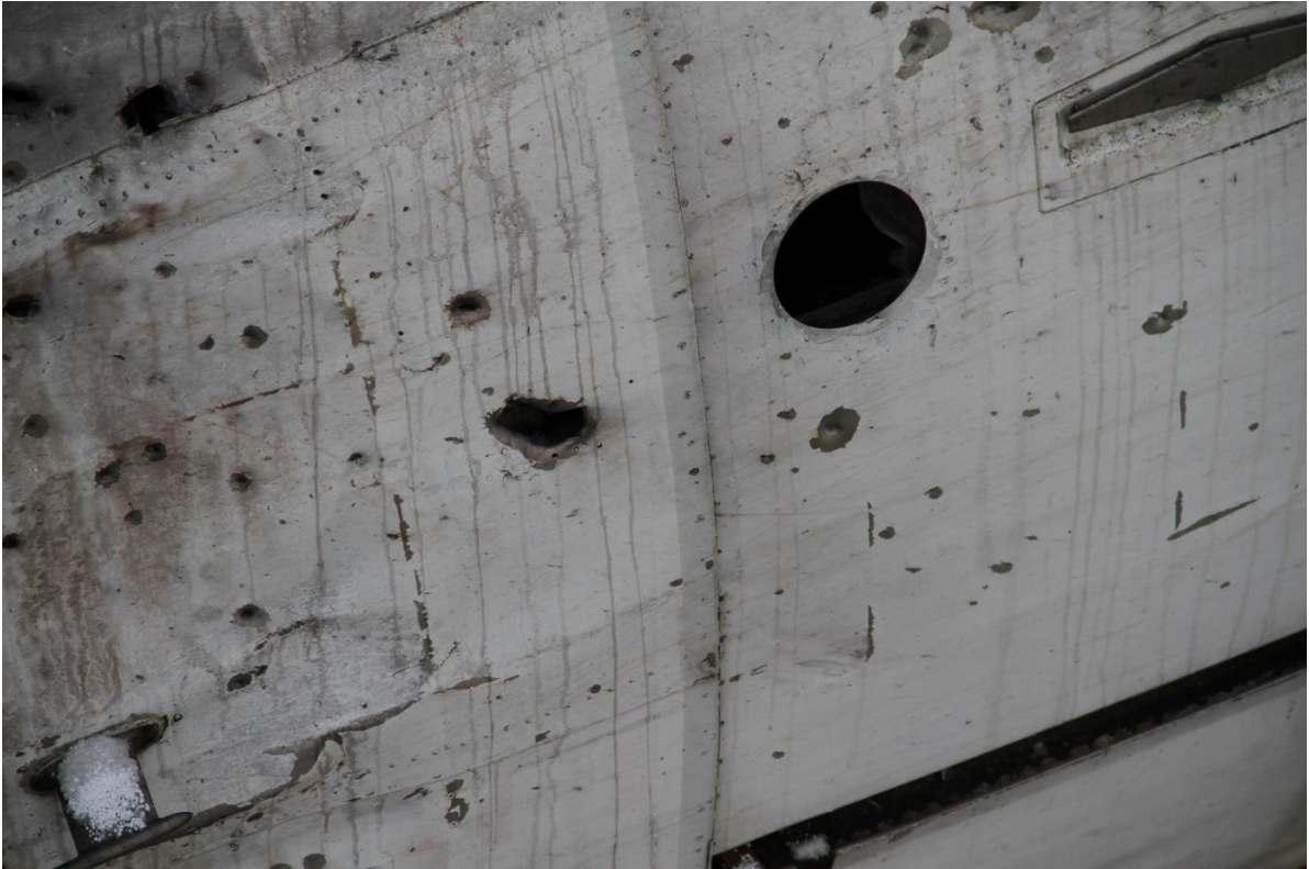
Figure 5.31 - Port side in L1 door area. Characteristic holes caused by hull fragments are seen the dimensions of which are significantly greater than those of holes caused by ready-made projectiles
