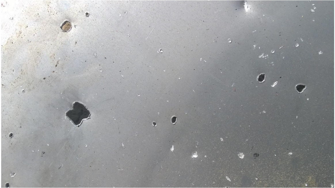
Figure A.190 - Fragment of target with marks of secondary damage
