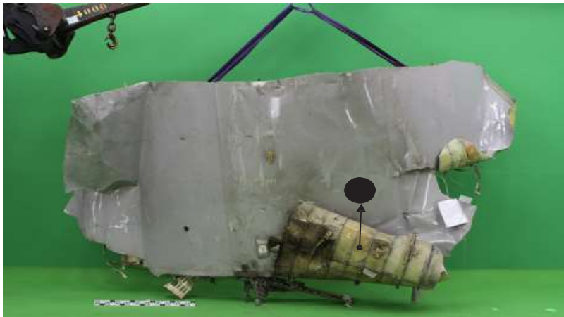
Figure 55 – Example of bending/peeling at a fracture line located along STA655 associated with the final separation between two pieces of wreckage.
