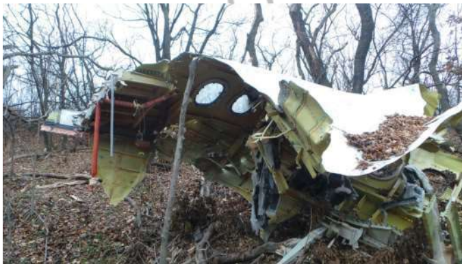
19 20 Figure 63 – Severely deformed fuselage structure aft of passenger door 3R, 21 including aft cargo door surrounding structure (source: DSB) 22
