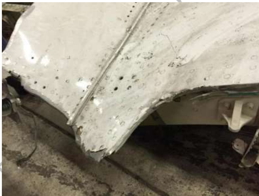
Figure 59 – Tensile overstress fracture at the upper right door corner of passenger door 3L
