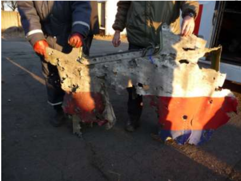
17 Figure 19 – Handover of the left cockpit window to the DSB by members of the 18 SES. (Source: DSB)
