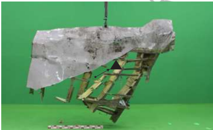
Figure 56 – Example of skin/sub-structure separation in the nose section immediately forward of the door 1R.
