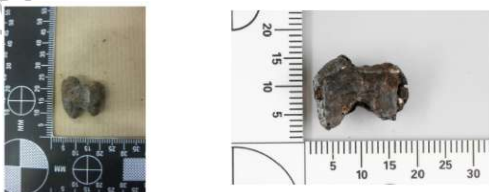
26 Figure 21 – Fragments found with butterfly or bow-tie shape. The right hand 27 fragment was found in the body of a flight crew member (Source: NFI)
