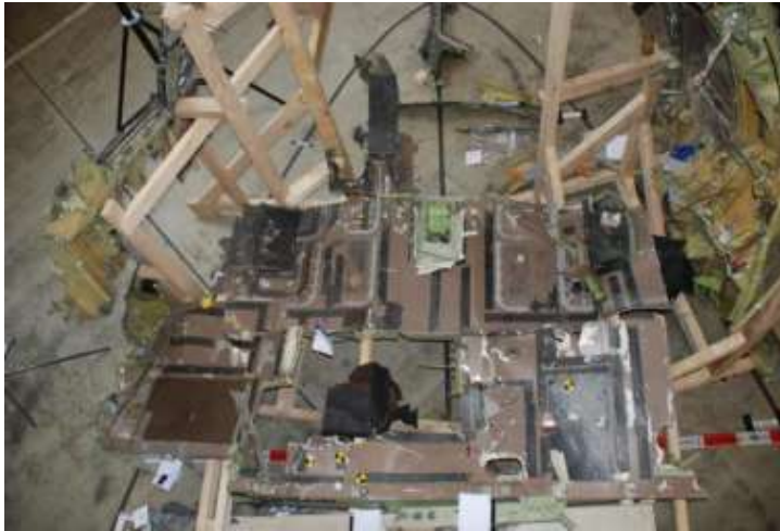
5 Figure 17 - Cockpit floor overview partially reconstructed in Gilze-Rijen (Source: 6 DSB)
