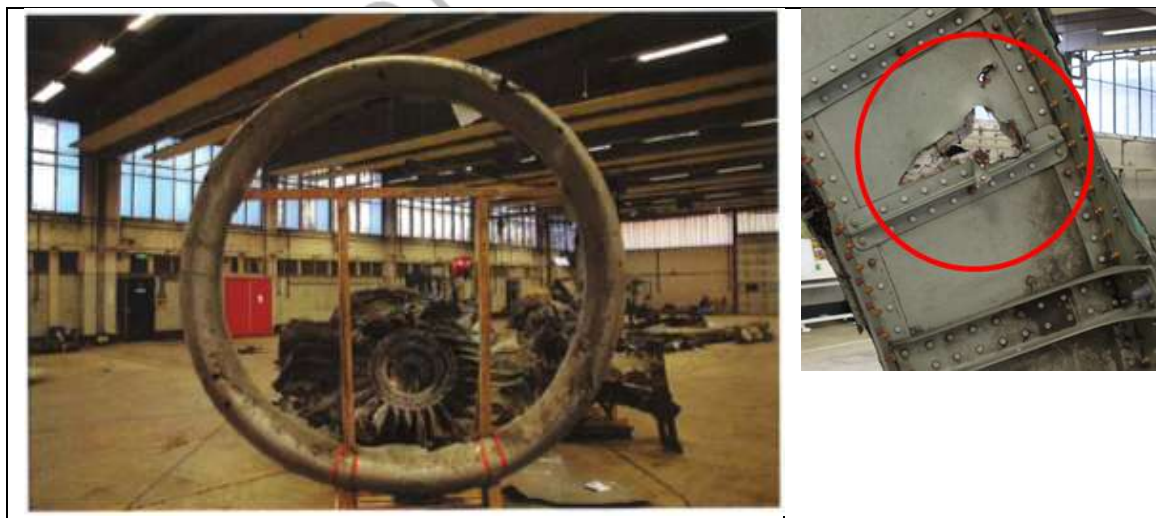
25 Figure 14 – Damaged left engine nacelle leading edge (left) and impact marks at 26 the 200 degree position shown from the rear side (right) (Source: DSB)
