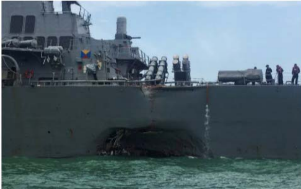
Damage on the US Navy guided-missile destroyer USS John S. McCain after a collision CREDIT: REUTERS
