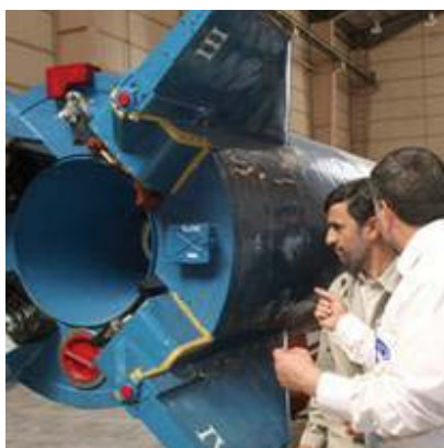
Safir space launch vehicle first stage Shahab-3 medium-range ballistic missile
