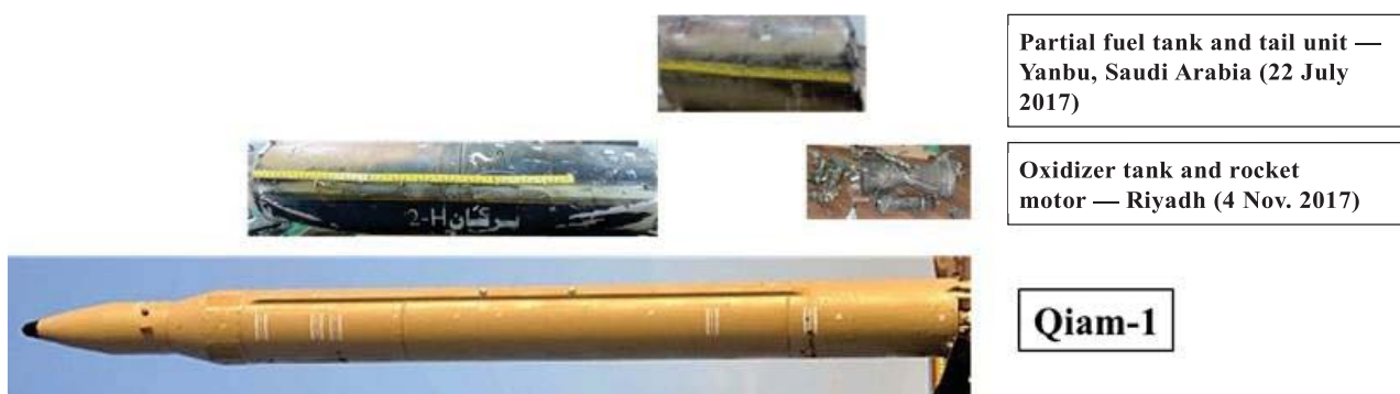
Figure IV Major components and their relative position compared to a Qiam-1 short-range ballistic missile a
