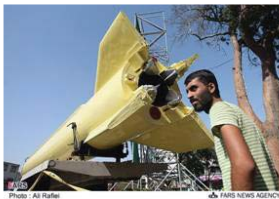
Safir space launch vehicle first stage Shahab-3 medium-range ballistic missile
