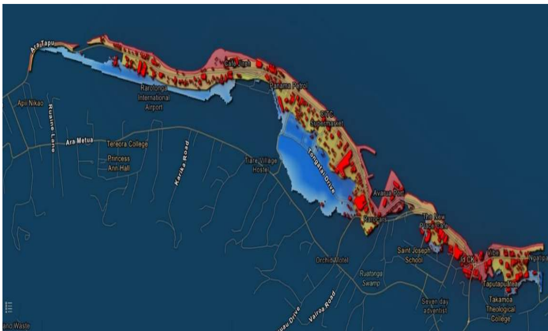
Figure 11. Map of One in 20-year average recurrence interval (ARI) for tropical cyclone events on the Avarua to Nikao coastline 152
