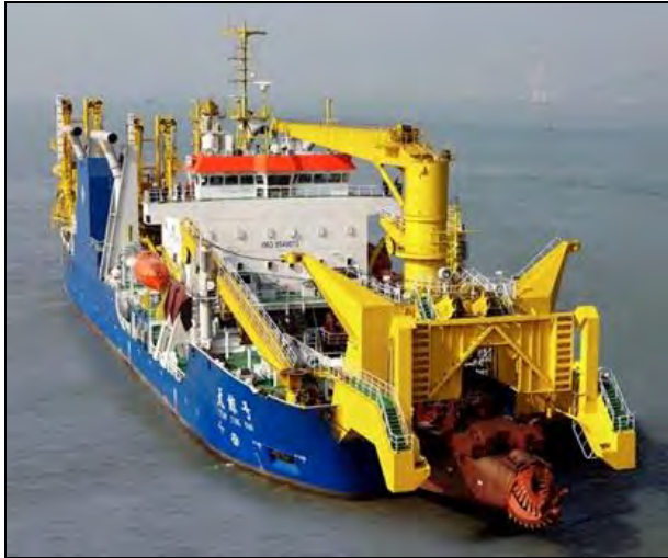
Figure 15: Tian Jing Hao, Cutter-Suction Dredge (Annex 858)
