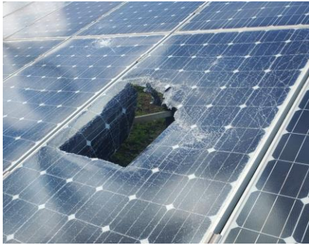
Evidence of damage caused by flying objects and projectiles.
