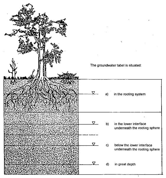
Figure 17: Effects of drop or rise of the groundwater table on the capillary water supply in the rooted sphere within a homogenous, sandy permeable medium.
