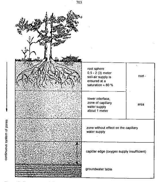
Figure 15: Characteristics of alluvial soil layers in a rooted, sandy, porous, homogenous seeping system (without scale) (Hary & Nachtnebel, 1989, p. 272).
