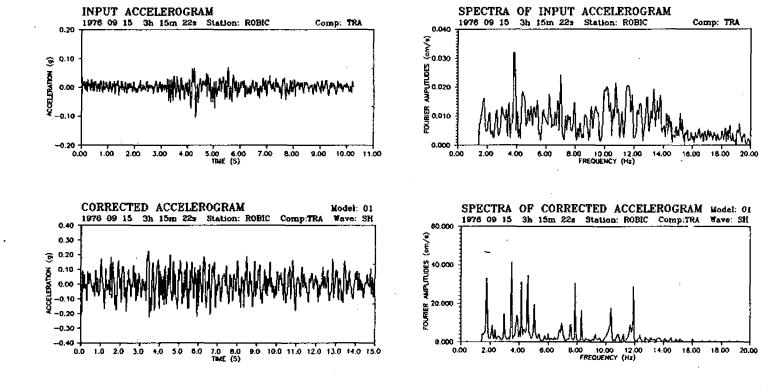
Figure 3. Transformation of acceleration appearing surface; transversal component on the bed-rock 5 the
