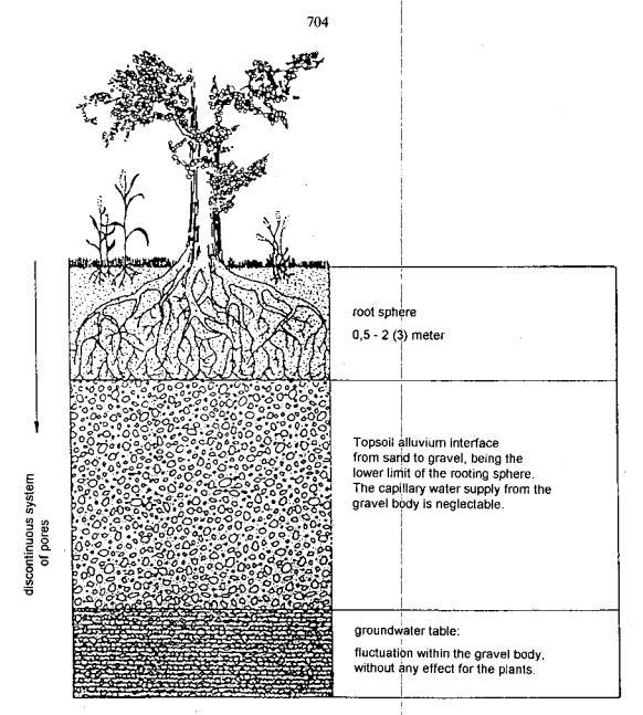
Figure 16: Characteristics of alluvial soil layers in an heterogeneous, two-layered seepage system of sand above gravel (Hary & Nachtnebel, 1989, p. 275).
