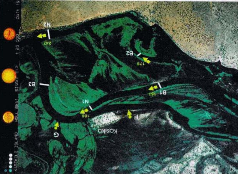
Figure 2 Measured flows in the northern and southern channels 30 April - 2 May 1998 Date of photography 19 April 1998
